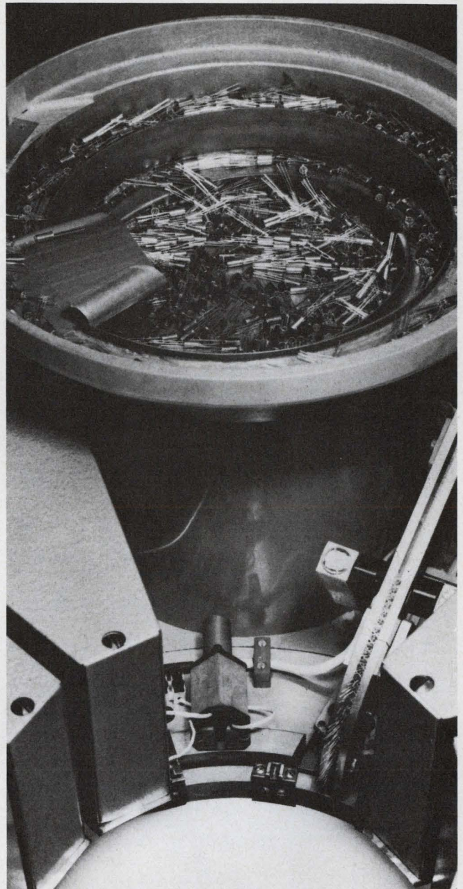
Transistors automatically tested from dc to rf, classified and then sorted. Page 176
