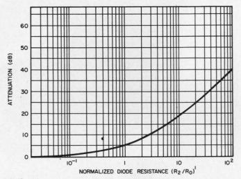
2. Continuously variable attenuation is achieved by changing the diode's resistance. Here the resistance is normalized with respect to the system's impedance,  $R_o$ . It is assumed that both diodes in Fig. 1 have the same resistances; which vary from 0.5 to 5000 ohms. The range of the attenuator is greater than 40 dB, and its insertion loss is less than 0.1 dB.
