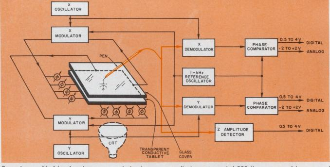
**Computer graphical input system** uses an electronic pen and a transparent conductive tablet. The pen makes capacitive contact with the conductive layer, and its co-
