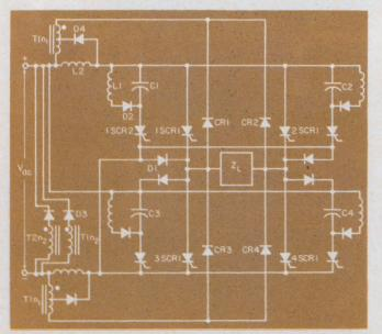
4. Simplified schematic of a 1.5-kVA inverter using the swinging turn-off circuit is shown without high-voltage suppressing and balancing networks. SCR1s form a bridge to provide a square-wave voltage across the load  $Z_L$ . Turn-off circuit for 1SCR1 consists of L1, D2, C1, 1SCR2, D1, D3, T1, L2, D4. CR1, CR2, CR3, CR4 provide current paths to discharge inductive loads into supply. See box for the component values.
