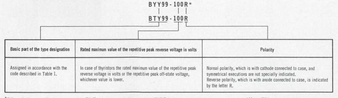
\*Silicon diodes, a rectifier in the case of the "BY" and a thyristor in the case of the "BT," for use in professional equipment. Both have 100-volt PRV and reverse polarity.
