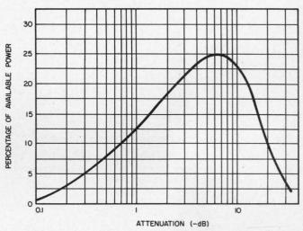
3. Dissipation in the diodes reaches its peak at the 6-dB attenuation level. The absorbed power is expressed as a percentage of the total input power. Each diode must therefore be rated to dissipate one-fourth of the controllable power. However, if  $R_1R_2 = R_0^2$ , then even a larger percentage of the input can be dissipated in a diode. Diodes can dissipate 1 to 5 watts with good heat sinks.
