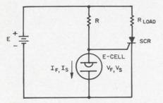
1. Basic timing circuit requires resistor and SCR.  $V_{\rm F}$  is voltage in timing condition,  $V_{\rm S}$  afterward. The max forward current  $l_{\rm F}$  must exceed sum of stop current,  $l_{\rm S}$ , and threshold current to fire SCR gate.
