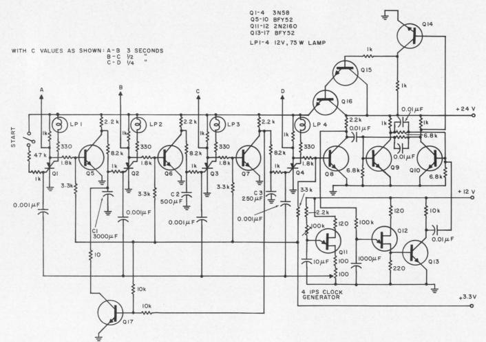
Time delay between events can be varied in this programed sequence switch. Input to the switch may be either mechanical or electrical. Time delay is approximately 1 ms/ $\mu$ F; delays up to 10 seconds are possible.
