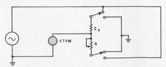
**Real part of Z** is determined by adjusting R until voltages across  $Z_x$  and R are equal. The value is then read off the dial of the decade box, R.
