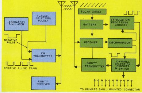
1. General Electric Mark II telestimulator permits remote stimulation of more than one monkey in outdoor primate colony. Miniaturized switch steps output pulses through 11 electrodes.
