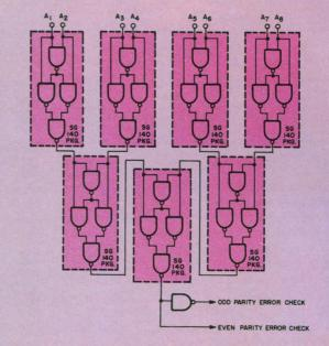
Fig. 3-Parity checking for 8-bit binary word which includes the parity bit.
