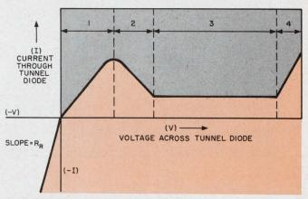
3. Four approximately linear regions make up the characteristic curve of a tunnel diode.
