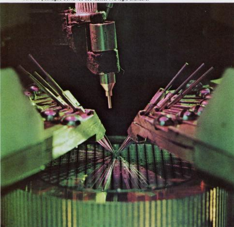
Mechanized wafer-level testing with this 14-point probe.
