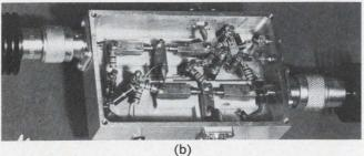
5. **Power attenuator** is designed for 200 MHz. A spdt diode switch (D3 and D4) has been added to provide a fixed attenuation of 23 dB. The variable attenuation of 28 dB is controlled by  $V_{C1}$ , as shown in (a). The size of the prototype package is about 4 x 2.5 x 1 inches (b).
