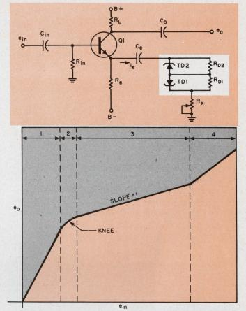
1. The basic circuit for a tunnel-diode log-amp stage (top) produces duo-gain characteristics (bottom). The circuit exploits regions 1 and 3. Region 2, the curve's knee, is minimized by selection of  $R_x$ . Region 4 is not used.
