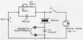
Versatile relaxation oscillator results when a neon bulb is combined with an audio crystal.
