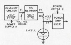
3. **Double-integration function** is performed as E-cell provides a signal source which indicates the distance from the voltage output of an accelerometer. Uses are in airborne cargo drops or ordnance.
