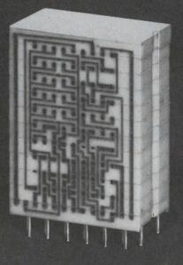
If you are working with a single chip or with complex circuit networks, Coors micro-ceramic modules offer you high reliability packaging. In the example above, the design engineer utilized base, frame, and lid modules to form a universal stacked package that can grow to fit any circuit density required. Each module is approximately 5/16" wide, 11/16"long and .050" high – indexed for high speed assembly. Because of the unique properties of Coors Ceramics, modules can be consider Coors ceramics
