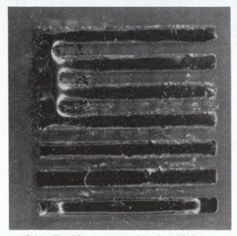
1. "Bridged" solder encountered in dip soldering operation is shown at left. Assembly at right shows uniform
