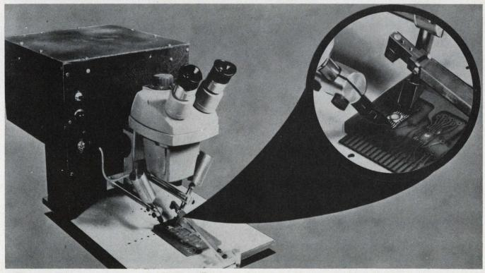
5. Typical resistance soldering setup. A Weller Electric Corp. unit is used. Soldering temperature is about 100°F
