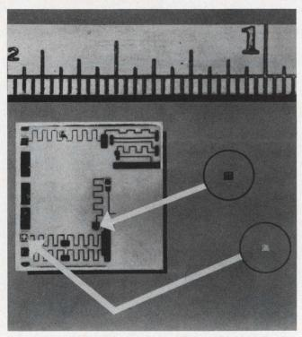
Active devices joined to a hybrid microcircuit. The same soldering techniques as for flat packs may be used.
