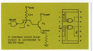
in the Figure. Here, the driving gate (or gates) is connected to the input of an SG-270 dual 4-input OR expander.
