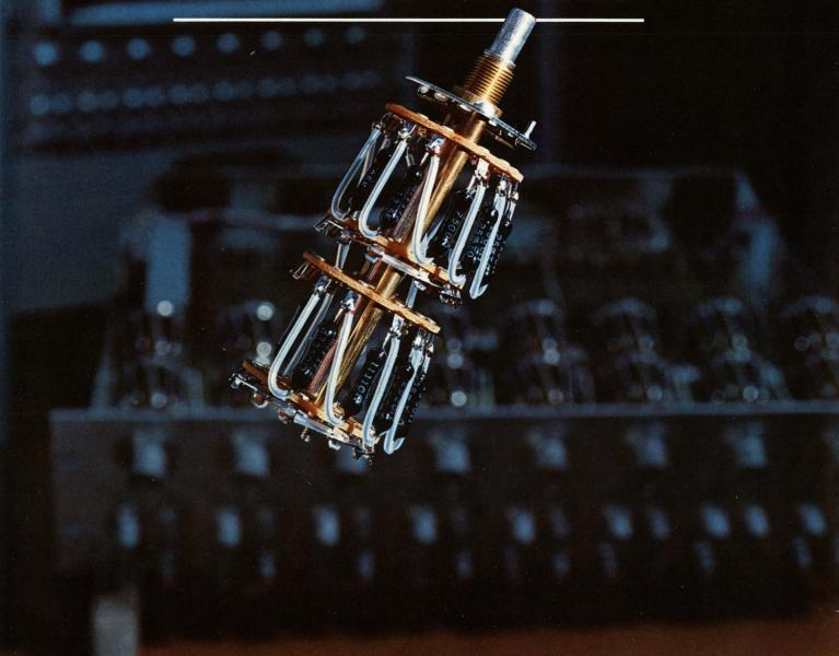
Dale Metal Film Resistors provide precise voltage attenuation in the Brush Mark 200 Recorder. This highly accurate direct writing system is now in use in the Apollo Deep Space Program.
