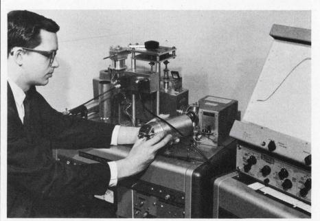
**Photoelectric cell** is plugged into new photodetector response recorder by National Bureau of Standards engineer David Goebel. A plot, representing a 4-minute scan of a photoelectric device, is shown on the x-y recorder. The monochromatic light source is in the background.
