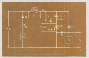
1. SCR swinging turn-off circuit to control power SCR1 is built with the components enclosed by the dashed lines. Load impedance has no effect on its operation.
