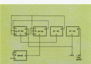
Fig. 1-Simple, accurate 1-Hertz generator using SUHL ICs.
