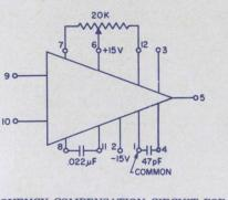
FREQUENCY COMPENSATION CIRCUIT FOR 6 dB/OCTAVE ROLLOFF (Ref: Note 2) FIGURE 3
