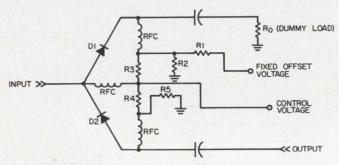
4. A single control source may bias both diodes if one of the diodes is reversed. Here diode D2 is reversed with respect to its original direction in Fig. 1.
