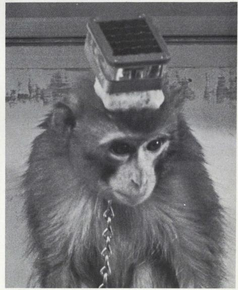
Solar array powers receiver-stimulator developed by General Electric Co. for Dr. Bryan Robinson. Head-mounted unit weighs 200 grams and measures  $7 \times 6 \times 3$  cm.
