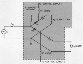
1. Basic attenuator circuit is built around two RF diodes. Both the generator and load impedances are assumed to be equal to  $R_o$ . The diodes are pin type and have resistive impedances through their bias range. The attenuation is continuously variable through the bias of the diodes, which varies their impedances from about 0.5 to 5000 ohms.
