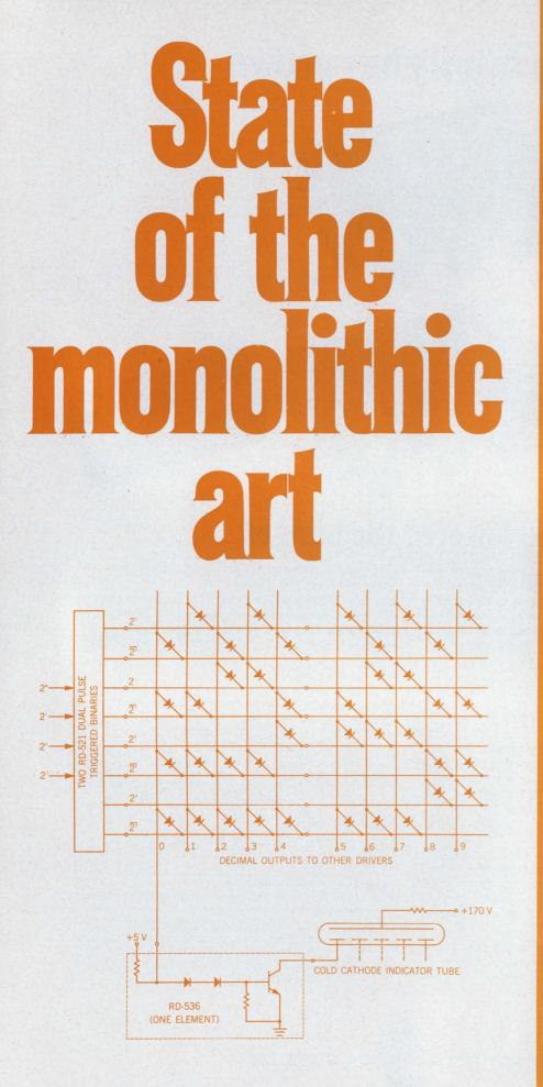
Radiation's Diode Matrices and High Voltage interface circuits provide all monolithic circuits for a cold cathode numeric display
