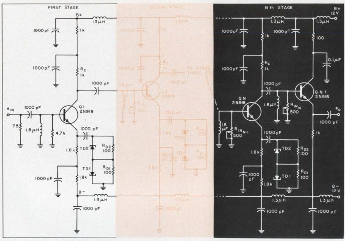
7. Complete schematic shows input stage, output stage and  $N^{\rm th}$  stage. All capacitor values are in pF. Transistors
