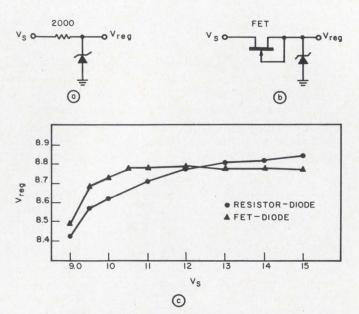
**Stable voltage output** results when a series resistor in a standard regulator circuit (a) is replaced by a suitable FET (b). The improvement is shown in (c).
