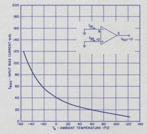
INPUT BIAS CURRENT VS AMBIENT TEMPERATURE FIGURE 7
