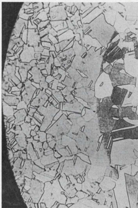
Oxide won't penetrate boron de-oxidized copper wire. Page 254
