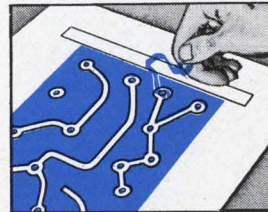
Now carefully peel off the film as outlined leaving a completed photo mask, positive or negative, that corresponds exactly to the desired pattern.
