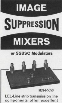
components offer excellent characteristics at microwave frequencies. **Image suppression mixers**, for example, are quickly available in 11 ranges from 925 to 5900 MHz. When used as SSBSC modulators there is a choice of IF's to 180 MHz. Specifications include:
