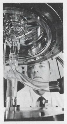
A sensitive air chamber in a fluidic gyro responds to motion changes by forming detectable vortical patterns.
