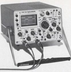
Tektronix Type 453 portable oscilloscope
