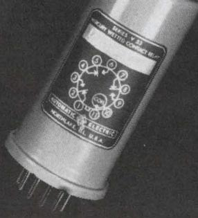
**CLASS V MERCURY-WETTED RELAY.** For computers, data processing and control equipment. Up to 200 operations per second. No contact erosion, no bounce. Over 1 billion operations without change, maintenance or adjustment. Can be operated within 30° of vertical. Polarized and nonpolarized versions. 1 pole to 4 pole double throw contact forms.
