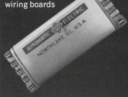
**PRINTED CIRCUIT CORREEDS.\*** Strong, moisture-resistant, compact. Unstressed contact leads provide firm, positive connections. Glass-filled plastic bobbins prevent moisture absorption. Low profiles and magnetic shielding permit high density within standard PC terminal spacing (multiples of 0.200 inches). Available with 1, 2, 3 and 5 capsules and magnetic latching. Contact forms A, B, & C.
