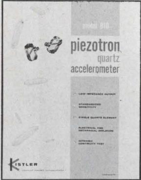
Four-page Bulletin 813106 provides answers to frequently asked questions concerning Kistler's new, easy-to-use, low impedance Piezotron quartz transducers which require only one wire for both signal and power. Subjects covered include power requirements, interface considerations, shock measurements, use with long cables, and environmental characteristics.
