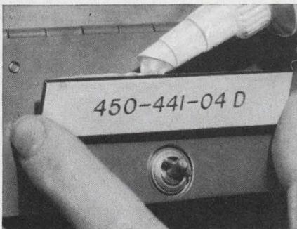
Screws and drilling are eliminated by adhering identification plates with RTV adhesive sealant. It won't harden, soften, crack or shrink.
