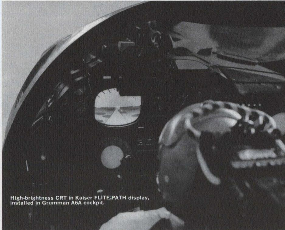
High-brightness CRT in Kaiser FLITE-PATH display, installed in Grumman A6A cockpit.
