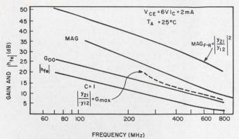
5. Gain and stability vs frequency curves for a commonemitter transistor configuration point up the fact that the maximum stable gain can be practically obtained only with a negative real termination.
