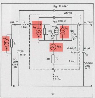
3. Accurate calculation of the noise figure requires an equivalent circuit that includes package parasitics. For a germanium planar transistor in a stripline package, the noise generators are  $i_{\rm ns}$ ,  $i_{\rm ne}$ ,  $i_{\rm ne}$ , and  $e_{\rm nb}$ .
