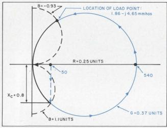
8. Load resistance transforming network transforms 50 ohms to 1.86-j4.65 mmhos. The capacitor also takes care of the dc isolation.
