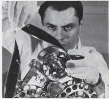
A new electronic reconnaissance and surveillance camera records images on a plastic film that has no magnetic surface and needs no chemical development. The film records images by storing electric charge in its dielectric surface.
