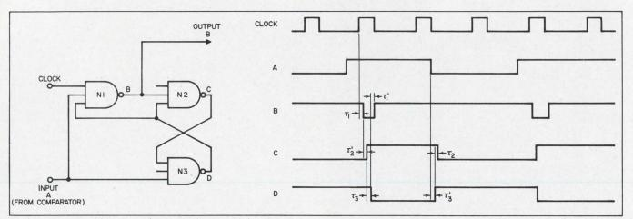
5. The narrow pulse (waveform B) generated by the differentiation circuit is used to transfer the content of the master counter into the appropriate storage circuit.
