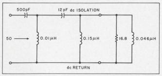
12. Input admittance of terminated stage at 450 MHz (left) requires a matching network toward the generator (right), dc return to the base and dc isolation.
