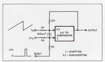
4. Comparison between input voltage and sawtooth waveforms is accomplished by the comparator circuit which uses an off-the-shelf IC differential amplifier.
