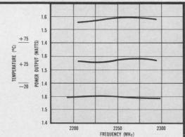
Typical Results: 1.5 watts from our X8 Multiplier at 2250 MC. Spurious signals down at least 30db-mid-band efficiency typically 25%
