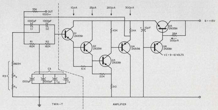
2. Twin-T network is inserted into the negative feedback loop of the amplifier. The regulator-filter (05 and 06)
