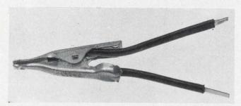
Flexible circuit probe is made from standard alligator clips and double-clad flexible printed-circuit material.
