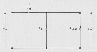
3. Simpler model of regulator circuit assumes operation over the more linear portion of the characteristic curve. As a result, the regulator often appears to have poorer regulation than it actually has.
