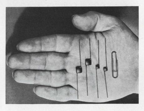
The Mallory TUR is a miniature solid electrolyte tantalum capacitor designed for use with integrated circuits, thin film and other microelectronic circuits. It is supplied unencapsulated to provide extremely small size per rating. It is intended for use with microcircuits where it will be encapsulated after assembly.
