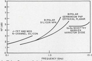
1. Noise figures of devices capable of microwave amplification indicate optimum performance for each type. The data were taken with bias currents and source immitances that yield the best results for each device.
