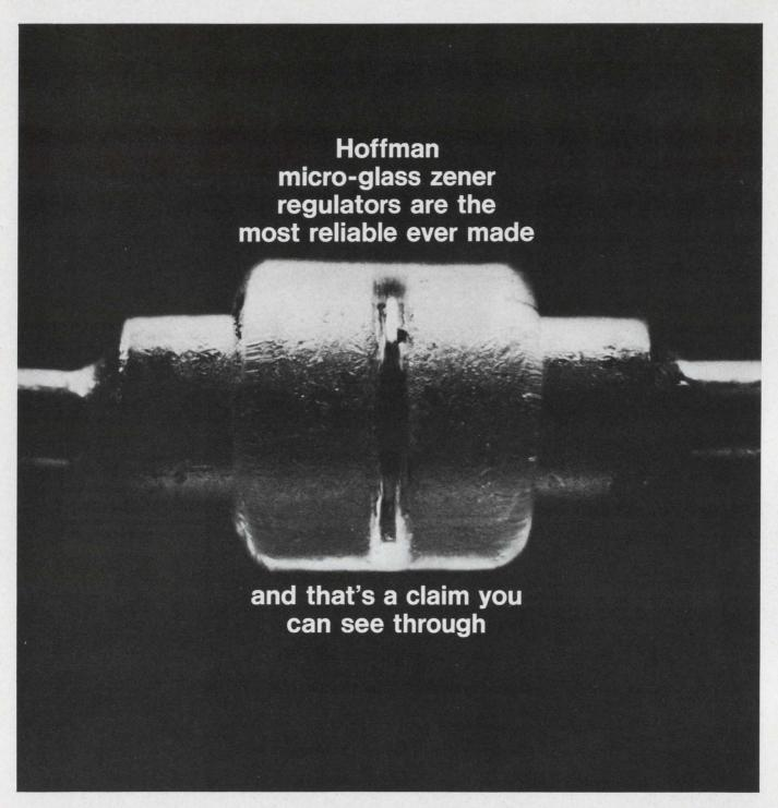
The reasons are hermetically sealed in glass. That's our exclusive way of keeping contaminants out and preventing any fusion of the metal-glass interface. The passivated silicon wafer looks like it's floating in the sleeve the glass doesn't touch the
