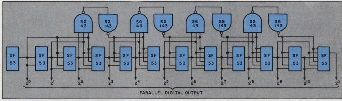
2. Binary digital outputs from this master counter drive the D/A converter which generates the sawtooth voltage
