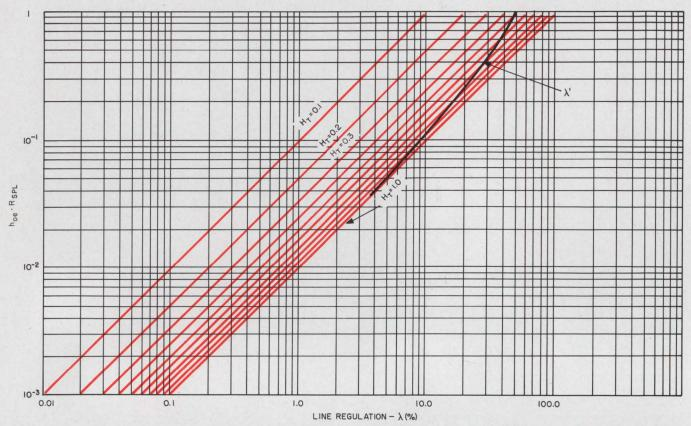
4. Line regulation as a function of the parameters and for various values of  $\mathbf{H}_T$ . For any given regulation the best
