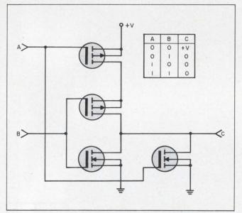
8. Complementary NOR gate has p-channel MOS-FETs in series and n-channel units in parallel (cf. NAND network in Fig. 7). Output (c) is "high" only when both inputs A and B are "low."
