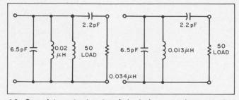
10. Complete output network includes a tuning capacitor of 6.5 pF and an inductance that resonates at 450 MHz (0.02  $\mu$ H).
