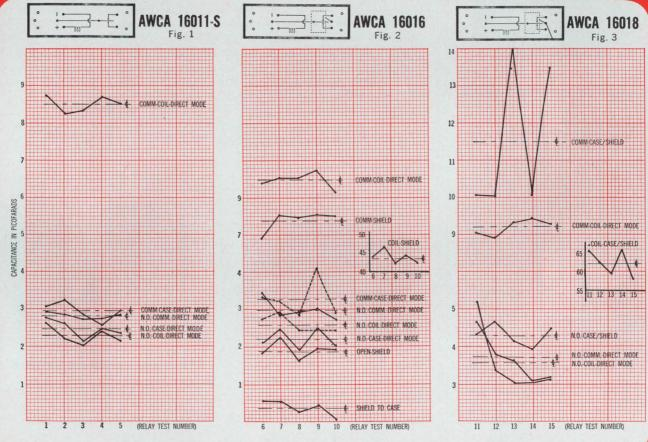
Data was obtained using a Booton Electronics Corporation Capacitance Bridge, Model 75-A-S8 at 1MHz
