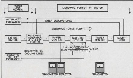
A clear plasma can be generated with this microwave plasma generator. In addition to their use in industry, microwaves are a valuable research tool in the investigations of materials. The high-power microwave beam frees ions and electrons in a moving stream of gas without introducing either a catalyst or electrodes.
