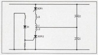
Saturable choke LS provides a trigger pulse for triggering SCR2 each time SCR1 is quenched.
