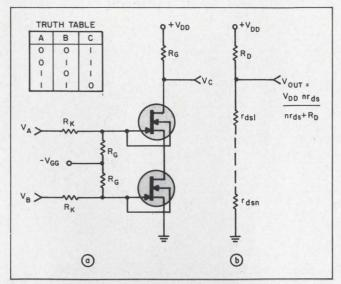
1. NAND gate is formed by connecting two J-FET inverters in series (a). If the truth table definitions of logical 1 and 0 were reversed, a NOR gate would result. Equivalent circuit for ON state of NAND gate appears in (b).
