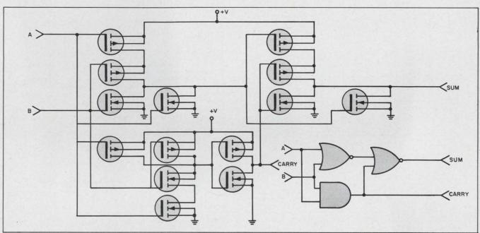
10. This half-adder requires no complementary inputs because a NOR gate in the half-adder of Fig. 9 has been replaced by an AND gate. In addition to its greater com-
