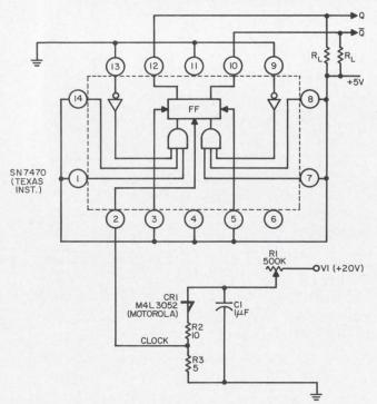
1. Square-wave generator uses four-layer diode (M4L3052) in relaxation oscillator. Pulse output of oscillator triggers clock input of integrated-circuit flip-flop.
