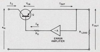
1. Regulator uses an error amplifier which compares the output voltage to an internal reference. The transistor's base drive is adjusted to regulate the output volatge.
