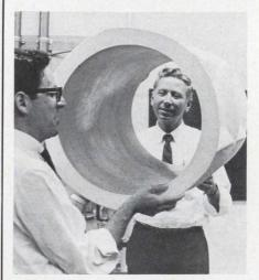
Microwave power pipeline section made of plastic foam is displayed by Prof. Donald Dunn (right) and a graduate student, Walter Loewenstern, Jr., both of Stanford University. By converting the electric power to microwave energy, they believe such a pipeline could carry billions of watts for hundreds of miles underground to cities of the future.
