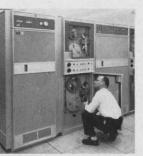
High Speed Data Communications Terminal—unique system extends computer processing facilities to remote locations via broadband transmission.
