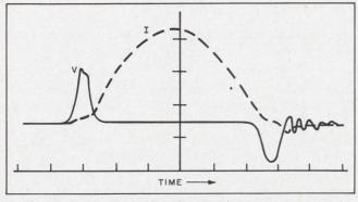
5. Waveforms from a saturable inductance in a series inverter are highly suitable for triggering other SCRs.
