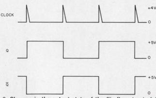
2. Changes in the output state of the flip-flop closely follow the input trigger from the relaxation oscillator. Output risetimes are on the order of 100 ns.
