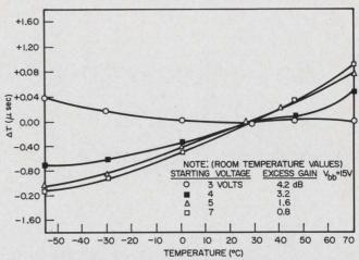
4. The total period change over the temperature range may be adjusted with the excess gain. The starting voltage is determined by the need for reliable starting. An excess gain of 1.5 to 2 dB seems optimum.
