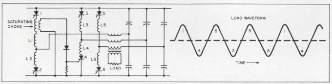
7. Complex high-frequency inverter consists of three series inverters sequentially feeding a common load. Sequential
