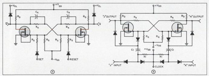
5. Flip-flops are easily built with J-FETs by vacuum tube design techniques. The reset-set (a) and J-K (b) multivibrator versions demonstrate this. One benefit of these circuits over their bipolar-transistor counterparts is their
