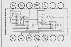
Two-bit numbers are added in this Dual Adder (a) just announced by Texas Instruments. Entire circuit is monolithically integrated (b).
