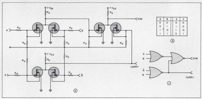
3. Half-adder is constructed with parallel NOR gates (a). Truth table (b) and logic diagram (c) show that comple-
