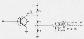
2. A resistor, R4, attenuates the saturation voltage. The amount of attenuation is limited by the ratio of E and V1 (OFF).
