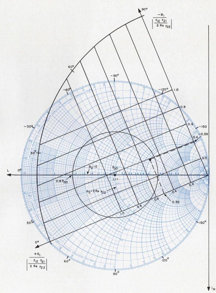
11. Quadrant chart, superimposed over the Linvill chart, allows a rapid analysis of the input immittance. The
