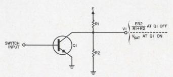
1. Basic shunt switch is used in many applications to produce a voltage level, V1, and then switch the output to zero. However, in practice the zero level is not reached because of the saturation voltage of the transistor.
