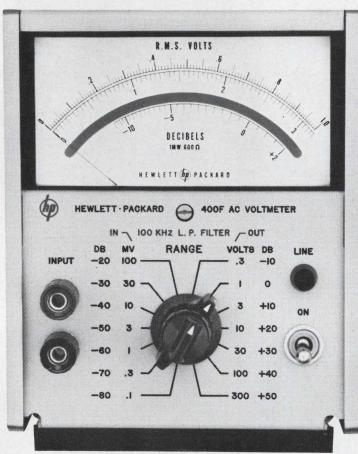
$100\mu v$  sensitivity—for unprecedented low-level ac measurements
