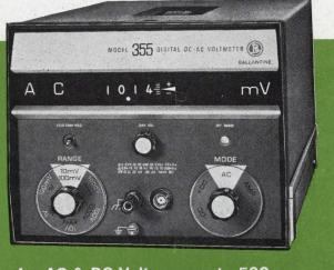
1/4% Accuracy f.s. for AC & DC Voltages up to 500 and for mid-band AC Frequencies
