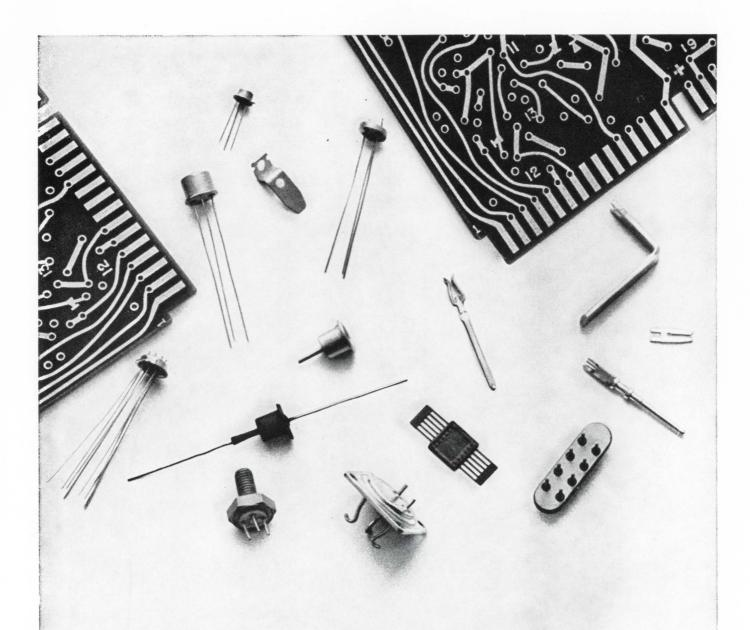
Gold-plated components conduct better, solder easier, reflect heat, and resist wear, corrosion, oxidation, galling.
