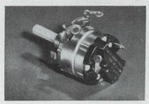
OCB breaker switch attached to volume control.
