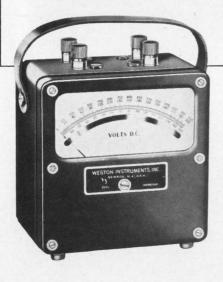
MODEL 622 PRECISION DC SERIES: ½% and ½% accuracy. Shielded permanent magnet mechanism. Many assorted range combinations from 5 UA full scale and up. Typical self-contained 20 range DC Volt-Milliammeter (½% accuracy); 750/300/150/75/30/15/7.5/3/1.5 Volts; 100/50 Millivolts; 3,000/1,500/750/300/150/75/30/15/7.5 Milliamps. Special RMS type thermocouple instruments with plug-in couples also available.
