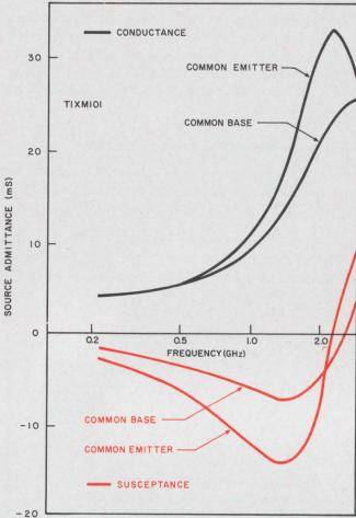
2. At microwave frequencies the optimum source immitances for low noise differ for common-emitter and common-base connections. The transistor is a bipolar germanium planar device.
