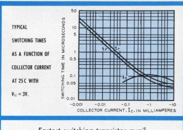
Fastest switching transistor available in the 1 to 100  $\mu$ A range.
