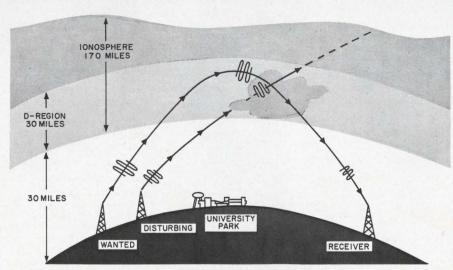
**lonospheric-disturbance experiment** is conducted by Penn State engineers with high-frequency radio signals. One signal, beamed into the ionosphere, causes a change in phase of a second signal, by heating the electrons in the ionosphere at the intersection point.
