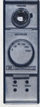
Use if for: Amplifying signals from low-level resistive transducers, such as thermocouples, strain gages. High input and low output impedance make it ideal for amplification over long transmission lines; use it, with resistive or reactive loads, such as x-y, strip-chart or oscillographic recorders, digital voltmeters, null detectors and servo systems, telemetry systems... or use it as a highperformance bench amplifier.
