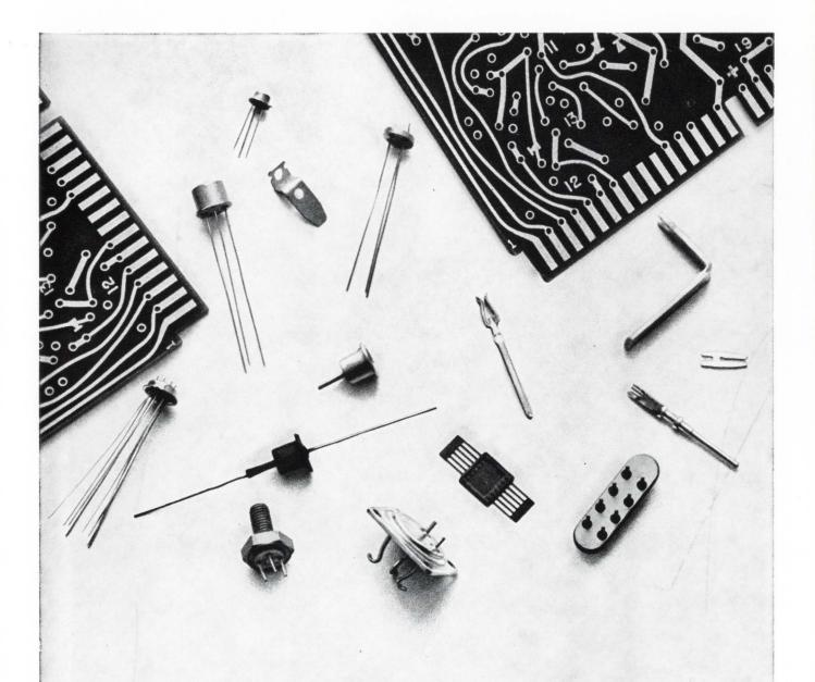
Gold-plated components conduct better, solder easier, reflect heat, and resist wear, corrosion, oxidation, galling.
