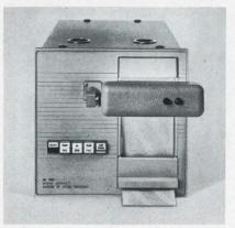
Monroe Datalog<sup>®</sup>'s MC 4000 ultra high speed optical printer records 6000 lines per minute, or any speed less that your application requires. Truly synchronous or asynchronous. Completely silent. Absolutely reliable—only two moving parts. Available in numeric or alphanumeric models—both 32 columns wide. Any 4 or 6 line code with any logic level.
