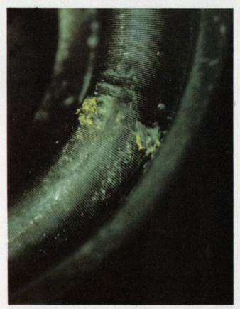
The entry of chemical agents caused a small section of the element to deteriorate. The resultant chemical action caused noisy performance.
