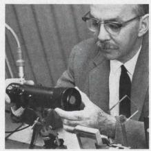
**Silicon disk** is placed over the aperture of a photodetector housing as an attenuator for laser measurements.
