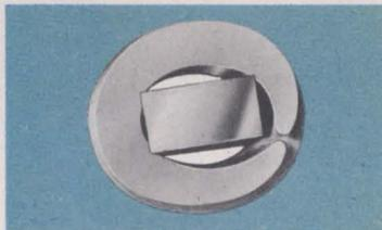
Film is scraped from wire and terminal at contact points. High pressure metal-to-metal contact invites solid state diffusion, maintaining low connection resistance.
