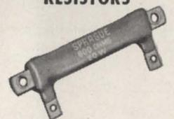
Flat silhouette permits stacking of resistor banks in close quarters. Aluminum thru-bar simplifies mounting and conducts heat from resistance element. Vitreous enamel protective coating. Meet MIL-R-26C performance requirements. Send for Bulletin 7430.
