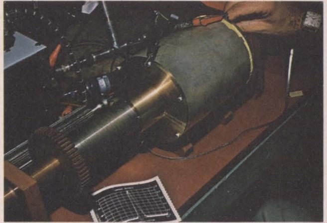
**High-Q cavity reduces noise** of cw Gunn oscillators. However, the cavity is large and not tunable electronically.
