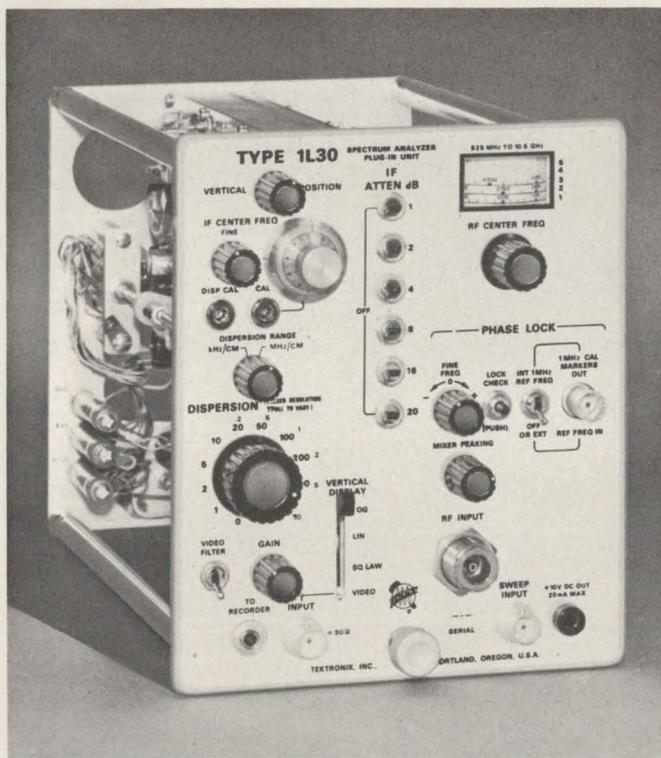
**phase lock**—Permits stable displays at 1 kHz/cm dispersion by locking the frequency of the RF local oscillator to the internal 1-MHz crystal-controlled reference, or to an external standard frequency.
