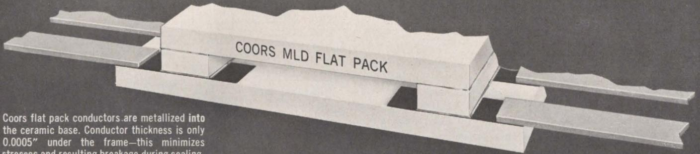
Coors flat pack conductors are metallized into the ceramic base. Conductor thickness is only 0.0005" under the frame—this minimizes stresses and resulting breakage during sealing.
