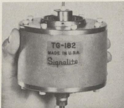
A triggered spark gap, type TG-182, has an externally adjustable main gap spacing and replaceable electrodes. This unit can be adjusted by loosening a locknut and adjusting the electrode by hand for a main gap breakdown range of 0 to 25 kV. It can be used over an applied voltage range of 1 to 20 kV and its energy handling capability is 6000 joules.
