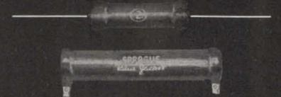
All-welded end cap construction with special vitreous coating for long-term dependability. Axial-lead style for conventional wiring or on printed boards. Tab terminals for higher wattage applications. Meet MIL-R-26C requirements. Send for Bulletins 7400B, 7410D, 7411A.
