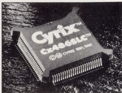
The Cyrix Cx486SLC \mu P runs i486 object code, features a CPU suspend mode, and has the same package size and pin assignments as the i386SX \mu P.
