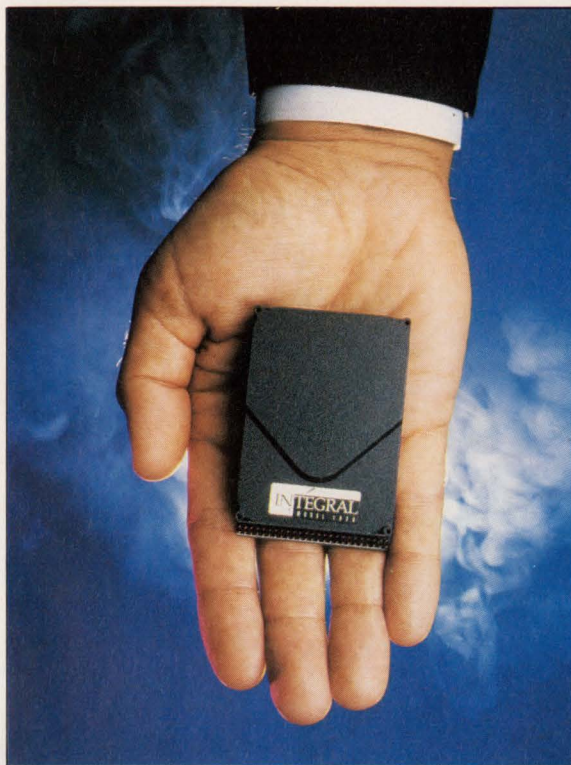
About the size of a small matchbox, this 1.8-in. hard-disk drive can store 21.4 Mbytes and operate from batteries.
