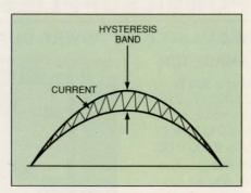
Fig 4—Using hysteretic current-mode control, the CS-3810 from Cherry Semiconductor generates a hysteresis band from a sinusoidal reference and an offset also derived from the reference. The average value of the waveform determines the inductor current.
