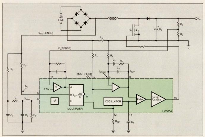
Fig 3—Typical of many of the power-factor-correction circuits is the UC3854 from Unitrode. Shown here in simplified form, the circuit contains both a current loop and a voltage loop.
