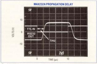
The MAX232A improves propagation delay and symmetry
