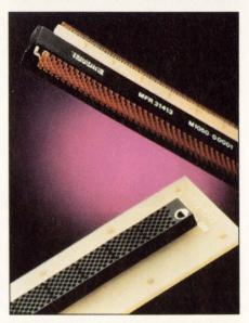
Featuring 396 contacts in a 5.44-in.-long housing, VHSICon UHD connectors from Teradyne accommodate high-density military/avionics applications.
