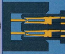
Precision Lead-In Design – assures that repeated connect/disconnect functions are consistently smooth and without pin damage.
