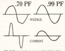
With .70 PF, current is drawn as narrow spikes during a short period of each half cycle. Power available from the line is cut by about 30%. In addition, harmonics generated by the excess ive peak current produce substantial power line noise and distortion.
