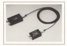
automatic gain control keeps the signal levels constant without readjustment.
