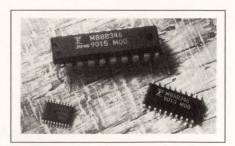
of the DAC accepts 2.5-MHz serial data. This data is loaded into internal data latches before the device converts the digital information into analog dc voltages in 60-µsec settling time. The DAC provides a serial data output that allows you to cascade devices. In 20-pin DIPs and SOJs (small outline J-lead) plastic flatpacks, \$4.50 (1000).
