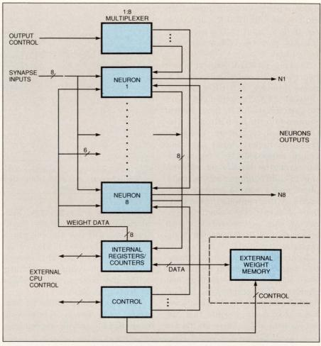
Fig 2—Eight neurons and 256 synaptic inputs make up the MD1220 neural-bit slice from Micro Devices. Via μP control, you can simulate large networks with a single IC, or you can cascade ICs and dedicate a neuron to every neuron in your model.
