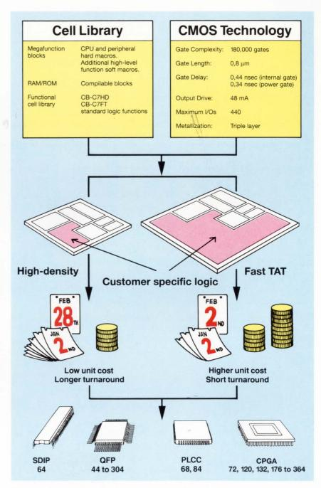
blocks and optimizing user-defined logic. It is then floor-planned using ChipPlan, simulated with System Hilo or Verilog, and placed and routed using Cell-3 Ensemble. After post-layout simulation and design-rule checks, we pass pattern generation data to one of our wafer fabrication facilities in Japan, the USA or Europe.
