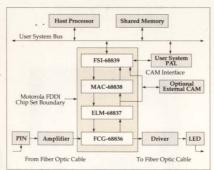
Media Access Controller. Together, they handle all FDDI functions quickly and efficiently, without the hassle or expense of external memory or high-speed logic.
