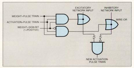
Fig 3—This multiply-accumulate model demonstrates how the NUSU32 IC from Neural Semiconductor uses pulse arithmetic to implement neural weights with less than 10 transistors per weight.
