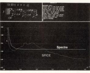
Charge-conserving device models allow Spectre to produce more accurate results than Spice.
