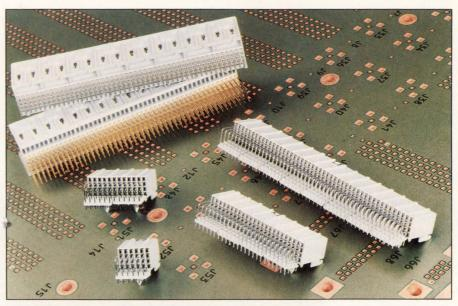
A modular system based on 2-mm centers, AT&T's Metral interconnects feature a basic building block that is 12 mm long and 4 rows wide. The modules are available in  $4 \times 6$ ,  $4 \times 12$ ,  $4 \times 24$ , and  $4 \times 48$  sizes and are designed to stack end-to-end on a card edge or backplane without loss of positions.
