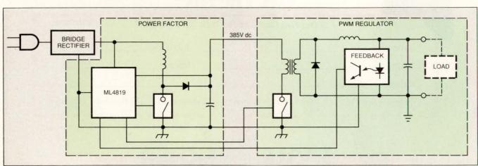
Fig 5—Combining PWM and power-factor controllers, the ML4819 from Micro Linear needs fewer components than other implementations.
