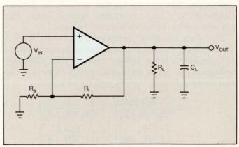
Fig 1—By adjusting the value of  $R_F$ , the feedback resistor that determines a current-feedback amplifier's bandwidth, you can optimize your circuit to drive almost any capacitive load.
