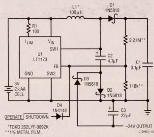
Figure 2. DC to DC Converter Generates –24V from 3V or 5V
