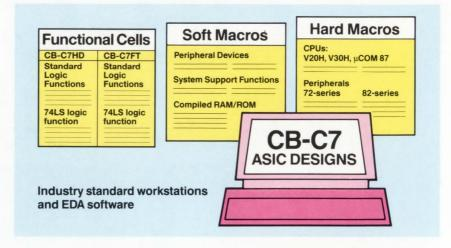
For example, the library of megafunction blocks contains cores of our  $\mu\text{COM87}, \text{V20H}$  and V30H microprocessors, plus intelligent peripheral functions such as those provided by NEC's 72-series and 82-series standard peripheral devices. And because most of these megafunction blocks are hard macros, derived directly from the chip layouts of our standard parts, they have fully characterized timing parameters and can be tested with the standard part test vectors.
