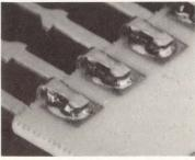
Precise amounts of the right solder and the shape of the ''Claw'' grip provide control of solder flow without a solder stop. This assures perfect mechanical and electrical bonding without wicking or bridging.
