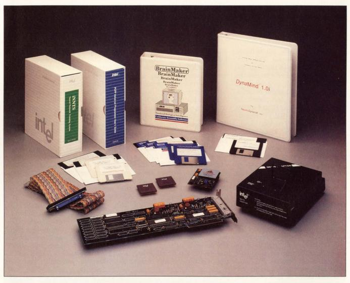
available and soon-to-be available neural-network ICs. Intel leads the way with the 80170NX ETANN (electrically trainable, analog neural-network) IC. The ETANN chip includes 64 neurons and 10,240 synaptic weights. The chip is based on the company's floating-gate memory-cell technology used in EEPROM ICs.
