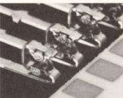
Direct contact between solder preforms and conductor pads produces a beneficial wiping action as clips are attached, either manually or with a lead attachment machine.
