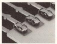
Interference fit holds clips firmly in position for reflow. Top and bottom preforms are reflowed in one operation using any method that raises temperatures to reflow levels.
