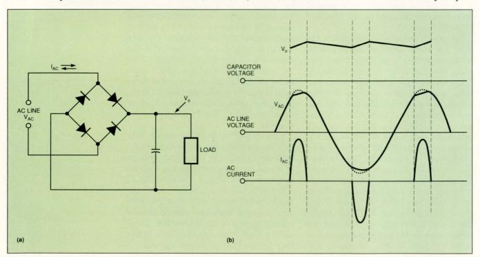
Fig 1—Power supplies using bridge-configured line rectifiers and a capacitor-input filter (a), draw current in a nonsinusoidal way (b). The full-wave rectifier charges the capacitor with pulses of current that occur only at the peak of each half cycle of the ac line voltage.
