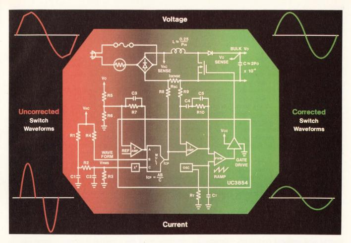
Because they don't deliver any power to the load, harmonics serve no useful purpose. Harmonics do, however, contribute to the total line loss, add to the current drain from the line, and dictate the need for higher-capacity wiring.
