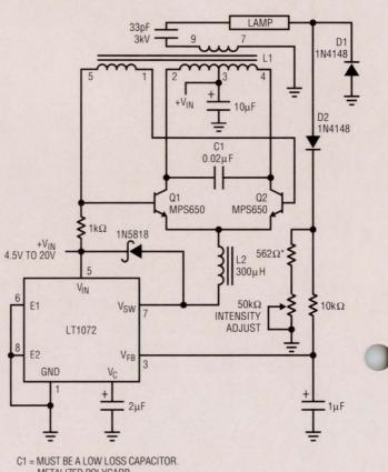
C1 = MUST BE A LOW LOSS CAPACITOR.
