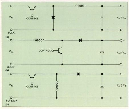
Fig 2—The three basic topologies used for power-factor correction are buck, boost, and flyback (buck-boost).
