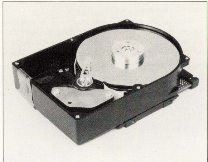
Synchronous 10M-byte/sec SCSI-2 data transfers suit the 540M-byte Rodime 3004T drives for use in workstations and file servers. The drives also feature spindle synchronization for array applications.
