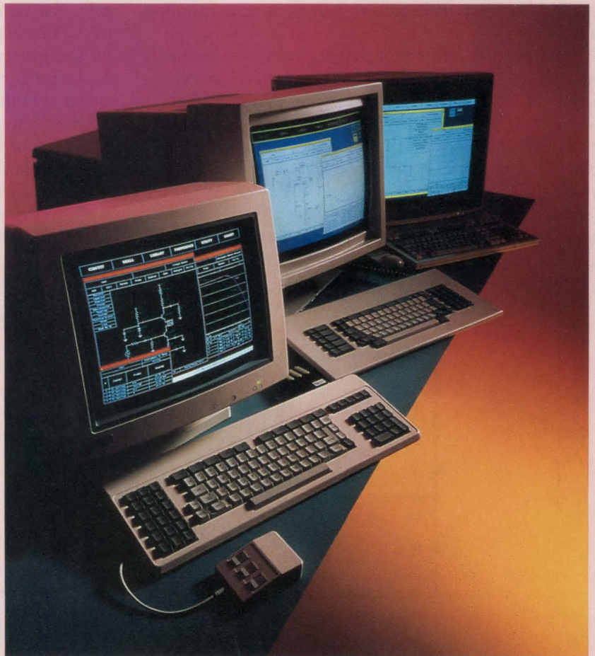
An interactive windowing environment allows designers who use Analog Design Tools' Analog Workbench to experiment with circuit models on a variety of workstations.
