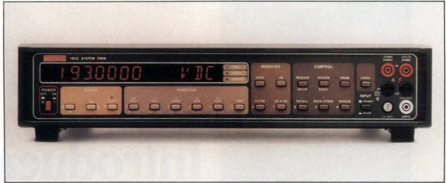
Translator software confers chameleon-like qualities on Keithley's Model 193 DMM. By storing new command definitions in its nonvolatile memory, you can make the DMM's IEEE-488 vocabulary mimic that of competitive meters.
