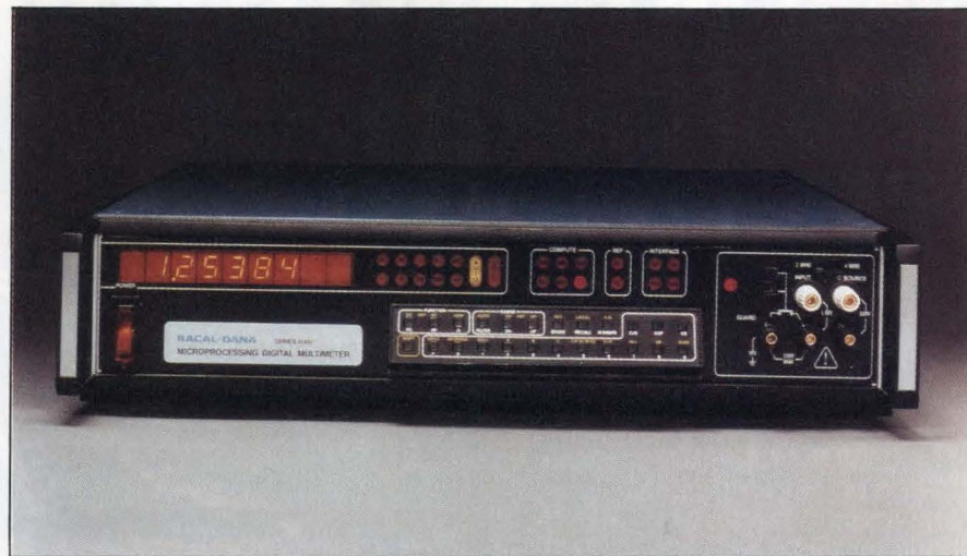
You don't have to take these meters out of service to calibrate them. In Racal-Dana's Series 6000 DMMs, all components that affect calibration are in a module—removable from the rear of the instrument—that you can exchange when the unit needs calibration.
