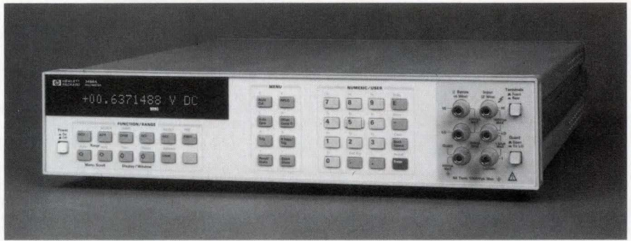
Called a "system multimeter" by its manufacturer, Hewlett-Packard, the Model 3458A performs 100,000 conversions/sec at 16-bit resolution. For a year after calibration, on its 10V dc range it delivers 8½-digit readings accurate to 8 ppm of reading plus 1 µV at 6 conversions/sec.
