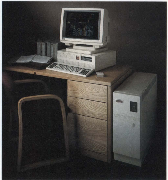
With the 192M-byte expanded-memory option, the Compute Engine Model M can simulate designs having as many as 325,000 gates. The Model M typically allows Apollo workstations to perform logic simulations 24 times faster than they could without the accelerator. This acceleration allows you to perform mixed-mode ASIC simulation at the system level.
