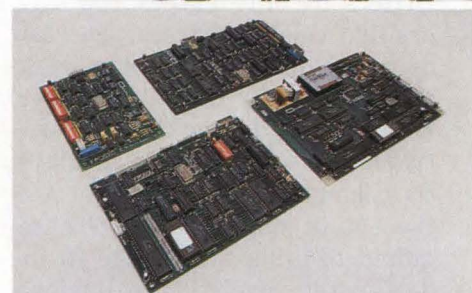
Interface and Controller Boards
