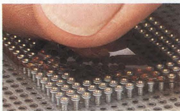
After the VisInPak socket is wave soldered into place, the carrier is removed to permit visual inspection of the terminals.
