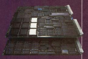
The 15 MFLOP SKY WARRIOR isn't simply a minor technological advance. It's nearly a revolution, fully twice as cost effective as anything else on the market. Capable of performing 15 million 32-bit floating point operations per second. And ½ million operations per second on 64-bit data.
