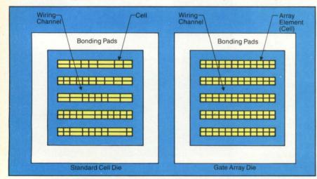
Figure 2: Traditional standard cells have fixed heights and variable widths. In gate arrays, the basic cell has a fixed height and a fixed width. When defining a logic function on a gate array, a complete cell must be accessed whether or not all the transistors within the cell are used. Since all of the masks in a standard cell design are customized, 100% of the transistors are utilized.
