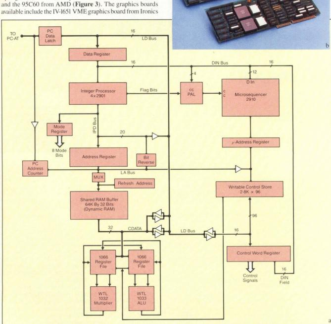
Figure 2: (a) Block diagram of Weitek's solids modeling engine which was first shown at SIGGRAPH last month. (b) The two-board set, implemented on the IBM PC/AT, is capable of complex graphics functions.
