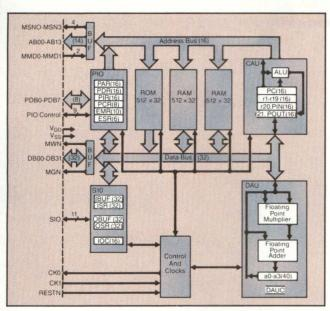
Figure 6: According to AT&T, its digital signal processor with 32-bit floating point arithmetic has a performance of 8 MFLOPs.
