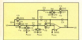
Figure 6: Switched-capacitor filters can be constructed easily with Gould AMI's library. The filter is designed using three cell types: a switch array, an operational amplifier and capacitor cells. Eliminating C1 results in the formation of a high-pass filter, eliminating C2, a low-pass filter.
