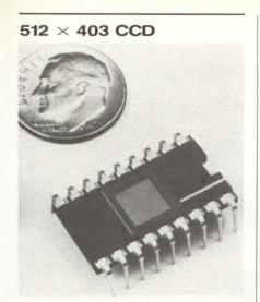
Intended for producing standard interlaced 525-line video with precision image geometry, the SID504 CCD contains 512 vertical × 403 horizontal pixels (206,336 picture elements). It has a spectral response that includes both visible wavelengths between 400 and 700 nm, and wavelengths extending into the nearinfrared spectrum to about 1100 nm. **RCA**, Lancaster, PA **Circle 191**
