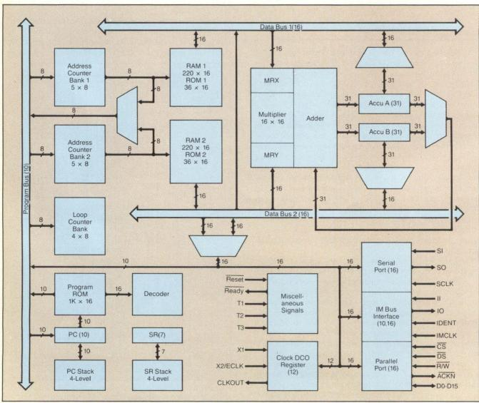
Figure 2: ITT Intermetall's digital signal processor has a data bus divided into two equal parts.
