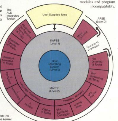
Figure 1: The ALS Integrated Toolset from SofTech illustrates the relationship between the 74 MAPSE and user-defined tools, the kernel and the host operating system.
