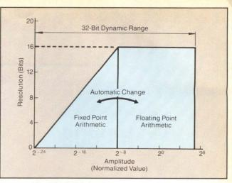
Figure 5: Hitachi's digital signal processor, the HD61810, achieves a 32-bit wide dynamic range and maximum 16-bit resolution using floating point arithmetic.
