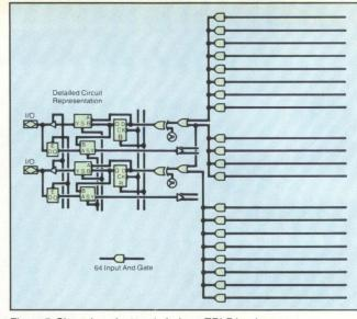
Figure 5: Shared product terms help an EPLD implement some counter and state machine applications efficiently. The two I/O cells shown here share the four middle product terms.
