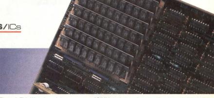
Figure 2: This Wang board shows an array of SIMMs in their sockets standing at an angle to reduce board-to-board spacing. The board shown will be used in a product to be announced soon. Since the module baby boards are not soldered in, customers can change and upgrade the system themselves without waiting for a repairman or an entire board to swap.
