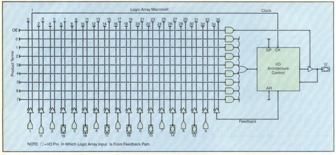
Figure 1: One macrocell shows that the structure underlying any EPLD consists of an EPROM-like memory array that controls I/O circuitry. An electrically programmable transistor lies at the intersection of each line in the array. This diagram illustrates one of the eight macrocells in Altera's EP300.
