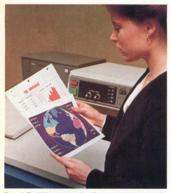
Figure 2: The 6500 color printer from Xerox combines laser scanning and xerography to produce 3 pages/min with 100 dot/in resolution.
