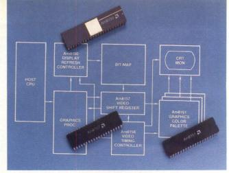
Figure 3: AMD's programmable three-chip graphics chip set is typical of the VLSI devices now available for graphics. Shown are the Am8150 display refresh controller, the Am8151 graphics color palette and the Am8157 video shift register.
