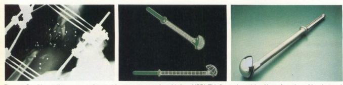
Figure 4: Graphics and image processing combine on systems such as this from MPDI. This figure shows (a) an X-ray of a patient with a shattered arm bone, (b) the CAD/CAM display of the upper arm bone generated on a Unigraphics II system after image pre-processing and vectorization and (c) a custom humerus shaft manufactured by CAD/CAM instructions.
