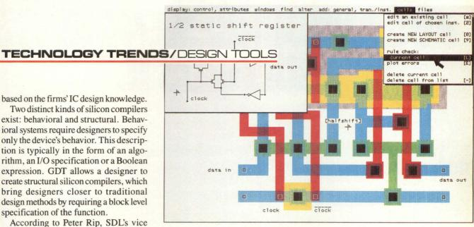
Figure 2: L-Editor, an interactive graphical editor, is the primary means of viewing the output of generators written in L. Its role is to aid in the development of module generators. Multiple windows and pull-down menus are among its features.
