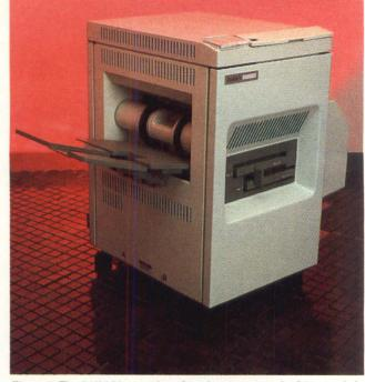
Figure 3: The 24/300 laser printer from Imagen can print 24 pages/min with 300 dot/in resolution and is based on the Xerox XP-24 print engine.
