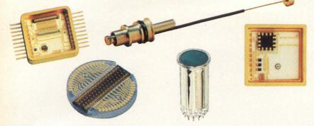
Cincinnati Electronics provides superior performance, high reliability, and on-time delivery in a broad range of custom and standard indium antimonide (InSb) IR detectors and custom hybrid focal plane assemblies.
