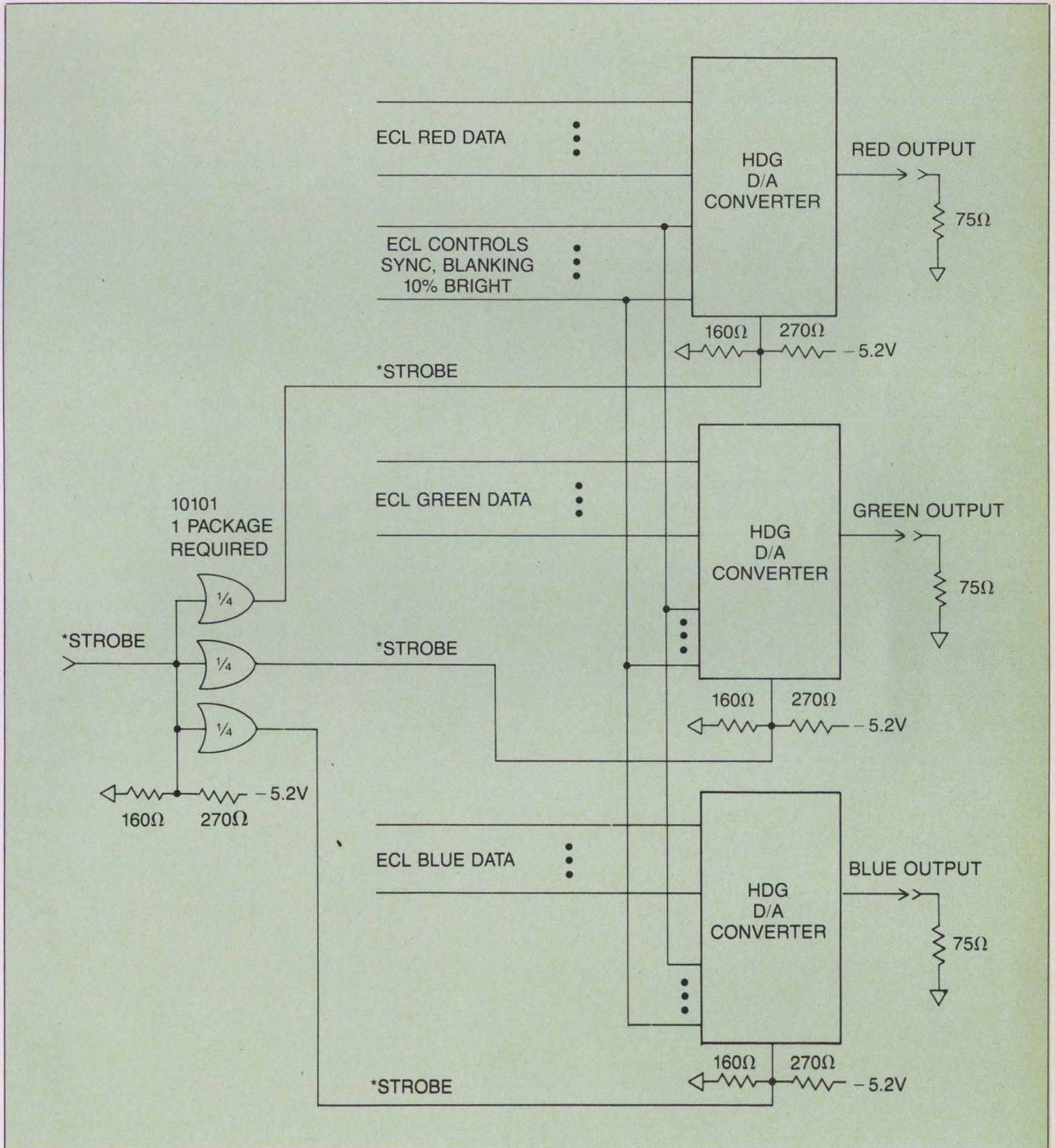
Figure 7: Strobe driver circuit. \*Note: Use 100Ω microstrip for strobe lines. Terminate data and control lines in 1000Ω to -5.2V for runs less than 1 inch. For longer runs use microstrip techniques as shown for strobe lines.
