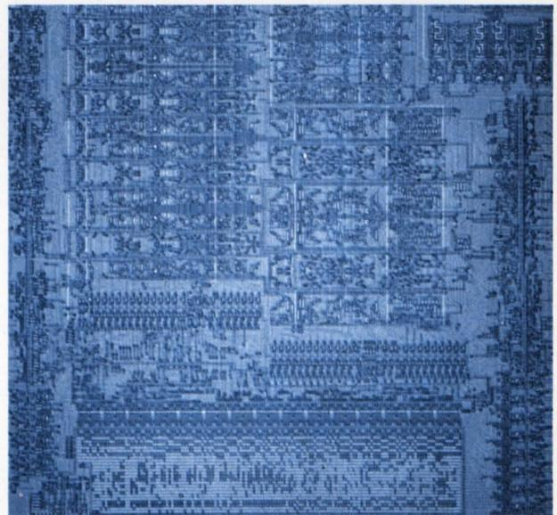
Figure 1: ZyMOS Corp's new "core  $\mu$ P" cell allows users to customize their own single-chip microcomputer. The new cell, designated ZyCOMP-4, is a general-purpose 4-bit  $\mu$ P without memory or I/O ports. By adding to the core processor appropriate memory cells, counters, timers and I/O ports from ZyMOS' ZyP design automation system library, users can quickly tailor the microcomputer chip to meet specific applications.
