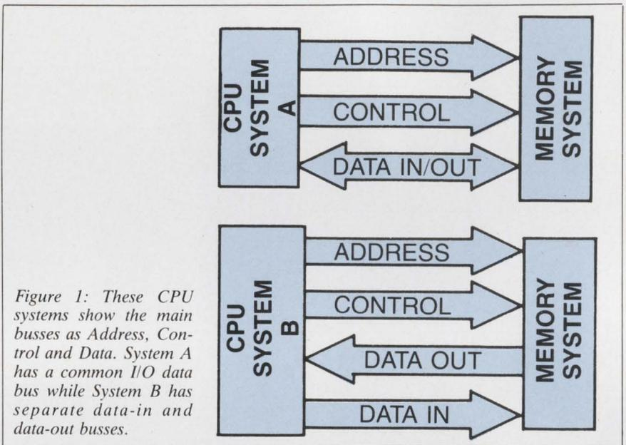
Figure 1: These CPU systems show the main busses as Address, Control and Data. System A has a common I/O data bus while System B has separate data-in and data-out busses.
