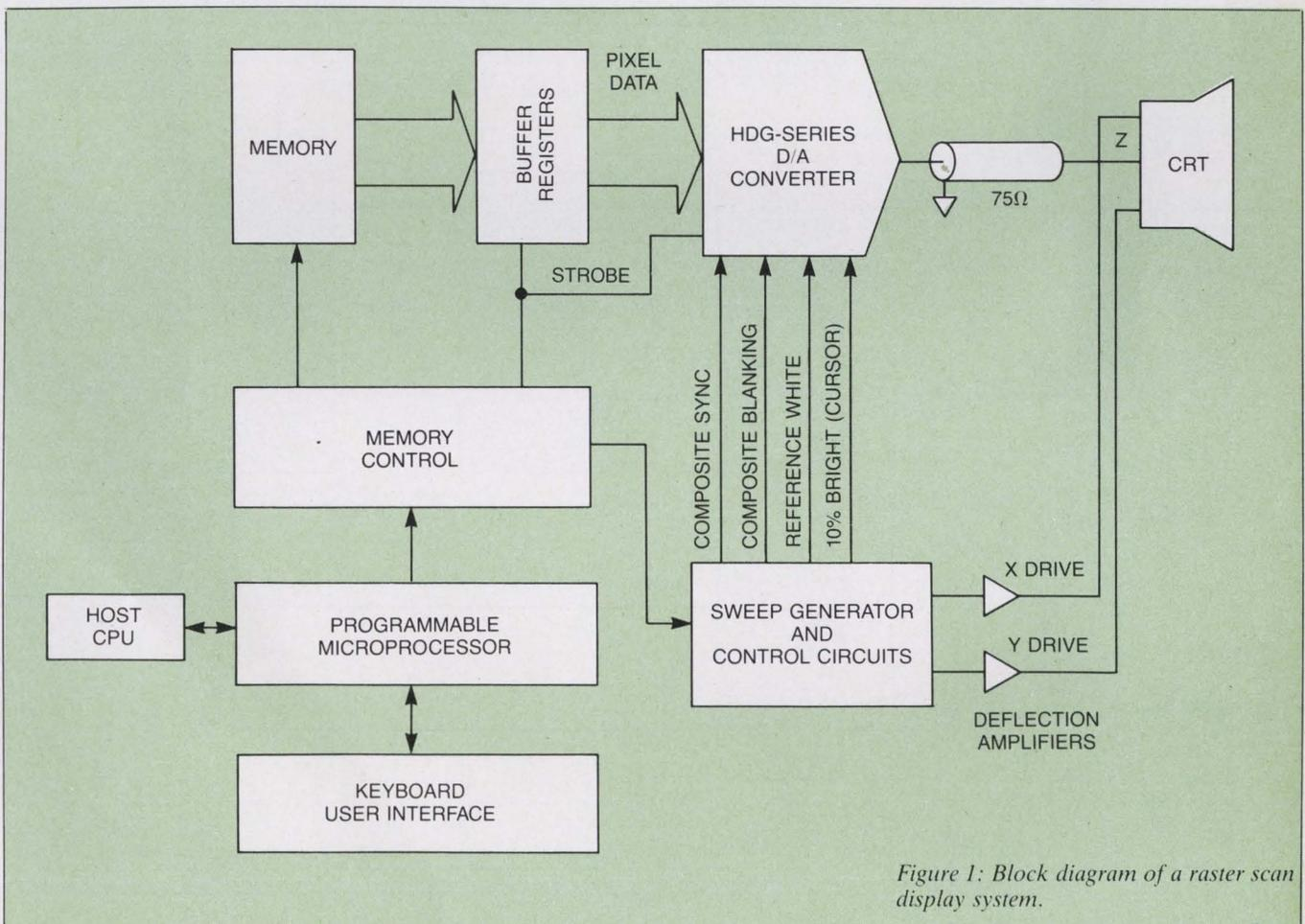
Figure 1: Block diagram of a raster scan display system.
