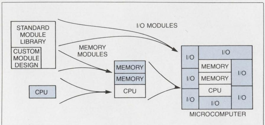
Figure 4: A custom alterable  $\mu$ C is made of modules. Modules may be used intact from the library, may be modified from standard library modules, or may be custom designed and placed in the library. In this illustration, memory and I/O modules are attached to the CPU to make a custom  $\mu$ C.
