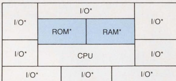
Figure 5: A modified "standard cell" design approach allows the system designer to configure an alterable  $\mu$ C to the application. In this drawing, all portions of the system marked with an asterisk (\*) are drawn from the standard module library or are custom configured. Only the CPU selection is fixed, and this restriction will undoubtedly disappear in the future.
