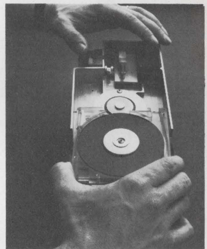
Figure 1: The SQ306 from Syquest Technology offers 5 Mbytes of storage in a 100mm removable cartridge drive.
