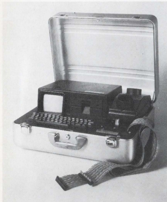
Figure 5: Detachable diagnostic devices, remotely tracing equipment problems, will soon be used routinely by field engineers. Failures in the field can be solved in this fashion 95% of the time.
