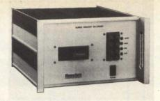
2000 bps, capacity of each bubble cassette — 64,000 bits, error rate of 1 bit in 10<sup>10</sup>, memory that remains undisturbed when power is turned off or when the cassette is re-
