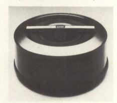
drives. It has 10 recording disks, 19 recording surfaces, plus top and bottom protective disks. A servo surface is prerecorded to provide precise control data for seeking, position sensing, and clocking. Track density is 384 tpi; bit density is 6,038 bpi. \$1,100. **BASF Systems Corp**, Crosby Drive, Bedford, MA 01730. **Circle 137**
