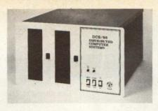
ports, 2 of which are capable of high level bit protocols such as HDLC and SDLC. One of the protocol ports is RS-232 and the other is RS 422/423 for network communications. The CPU also contains 24bits of parallel I/O
