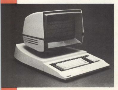
height of character. Operating power: 110/60Hz or 220/50Hz. It has a line or block graphic capability and is ASCII compatible.
