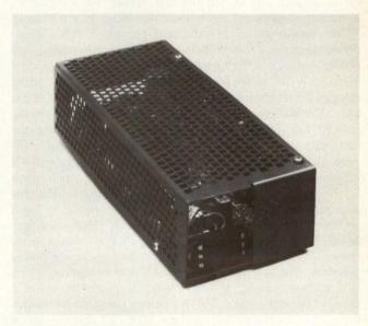
Figure 1: With 115 Vac or 230 Vac input at 47 to 440 Hz, Standard Logic's SWS 150 Series is designed for either domestic or European applications. It has good regulation on all outputs. Features include single phase input, 75% efficiency, low parts count, remote sense and remote shutdown capability.
