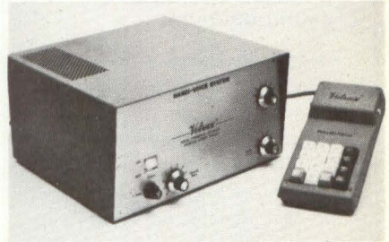
Artificial voice system stores 400 words, letters or phrases, which a verbally handicapped user can call up by entering an appropriate 3-digit code on the system's calculator-type keyboard.
