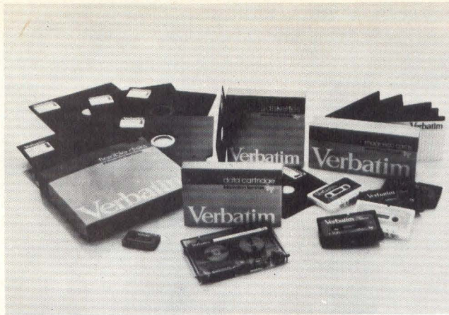
Fig 1 Typical mini media L to R — rear: diskette, minidiskette, magnetic cards; front: mini data cassette, data cartridge, data cassettes.
