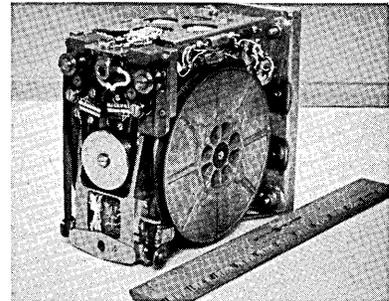
insure reliability. The tape unit includes a tape remaining indicator that transmits its information to the ground along with its communication data. All electronics use solid-state components and include record and reproduce amplifiers and a power supply which converts dc to ac for the drive motor and regulates the dc supply. CONSOLIDATED ELECTRODYNAMICS CORP., 360 Sierra Madre Villa, Pasadena, Calif. For information:
