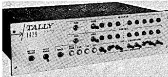
in one operation. The new unit handles tapes from one through eight channels in any code structure. The 1429 will verify duplicate at 60 ch/sec and failure to verify automatically stops the duplication function without punching an error character. Characters in disagreement are displayed for possible correction. Electrical requirements — 115V, 60 cycle AC at approximately four amperes. TALLY REGISTER CORP., 1310 Mercer St., Seattle, Wash. For information:
