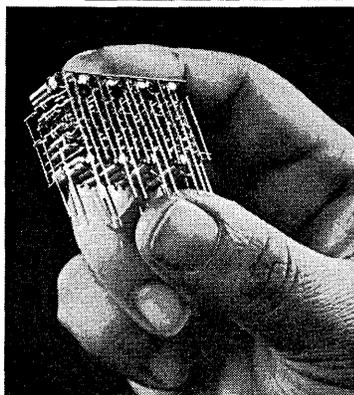
Welded wire techniques substantially increase component packing densities.
