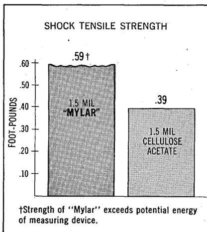
**Less breakage from shock.** Chart 1 compares shock tensile strength of "Mylar" with that of cellulose acetate. The strength of "Mylar" actually exceeds the range of the measuring device, while acetate failed at 0.39 foot-pounds. With
