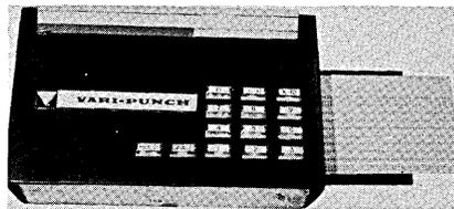
hole. An all-electric unit, it allows the insertion of variable data on an IBM card, directly at the source. It is available in two production models, will punch and print 40 columns (model A) or 80 columns (model B). **VARIFAB, INC.**, High Falls, N.Y. For information:
