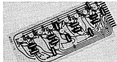
direct collector connections enable up to three milliampere loading for many external logical manipulations. Designed to operate from zero to 100 KC the counter supply voltage may be varied by over 2 to 1 margin. This feature
