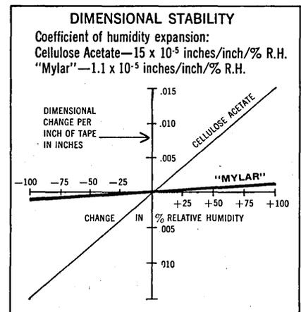
**Fewer weak or garbled signals.** Chart 3 shows dimensional change in "Mylar" with temperature or humidity change is negligible compared with that of cellulose acetate. This exceptional stability prevents tape shrinking, swelling or cupping that could result in shifting of tracks or loss of contact with the recording or playback head. Possibility of signal dropout or garbled or weak signals is minimized, and reliability of recorded data is improved.
