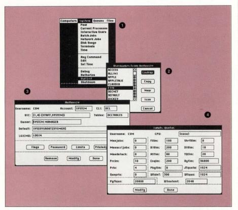
Screen 2: (1) A list of the users for the selected VAX system is requested through CSM and (2) returned through a CSM scrolling dialog box. (3) The selected user's account information is displayed and, by using the mouse to press the Limits button, (4) the user's quotas are displayed.
