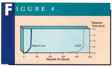
Comparison of response time vs. I/O demand for typical VMS timesharing I/O workload.
