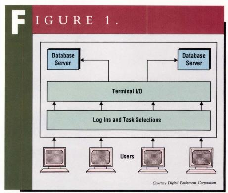
In DEC's multifile solution, which spreads the database across disks to increase throughput, users don't need to know where their data resides. The transaction generator (at terminal I/O) directs input to various database servers. The servers then direct it to the disks.
