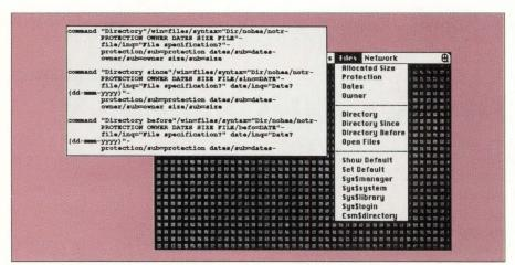
Screen 3: The relationship between commands in a CSM database file and the options presented within a CSM menu is shown. Site-specific commands can be incorporated into CSM by editing the appropriate CSM database files on the VAX.
