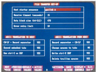
Screen 1: Reflection's File Transfer Setup screen lets you change a number of file transfer parameters.
