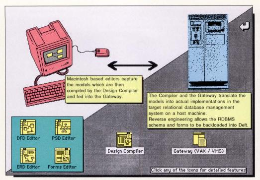
Front-end design is done on the Mac. An application is generated on the VAX.
