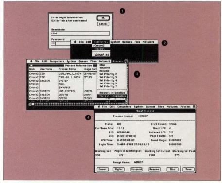
Screen 1: (1) Example CSM session begins with CSM log in. (2) VAX systems to be managed are selected from CSM's Computers menu. Current Processes then is selected from the System menu. (3) A particular process can be selected and controlled. (4) CSM's Show Process dialog box presents process information and accepts management functions.
