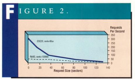
Comparison of request rate vs. request size, ESE20 vs. RA90.
