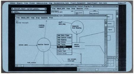
Screen 2: The DFD Editor allows you to draw Data Flow Diagrams that follow the Yourdon/DeMarco system-analysis methodology. The diagram's data can be entered automatically into the model's project database.
