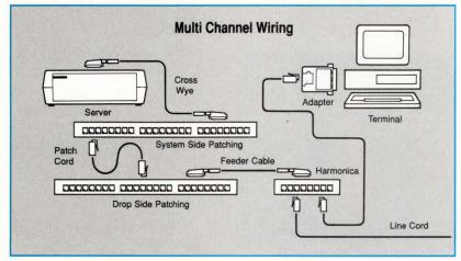
25 Pair multi channel cables consolidate individual wiring channels. These channels run from the wiring closet to the feeder split (harmonica) located in the office area. Perfect for use in open/modular office environments. Greatly reduces installation costs, provides versatility, and restores order to your communications wiring system.
