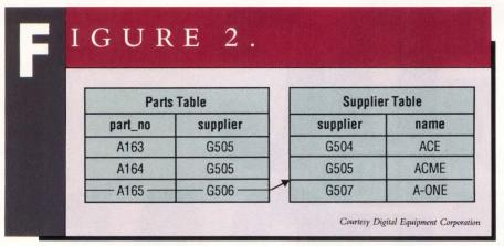
Rdb/VMS currently offers referential integrity with constraints. Here, in a design to keep the database consistent, it's impossible to enter "A165/G506" from the Parts Table into the database because that code doesn't exist in the Supplier Table.
