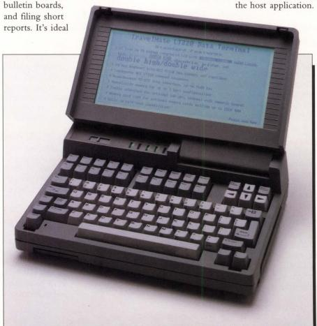
The diminutive LT220, from Texas Instruments, features a 25-line screen and communications at 1,200 or 2,400 bps.
