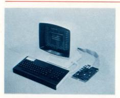
VDC11-C intelligent display controller provides add-in graphics capability for Q-bus systems.
