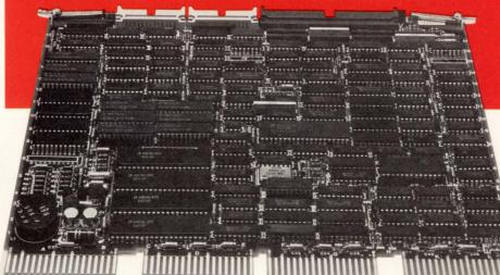
LSI-11<sup>®</sup> compatible controller for 80-300MB CDC, Ampex and Fujitsu CMD/SMD
