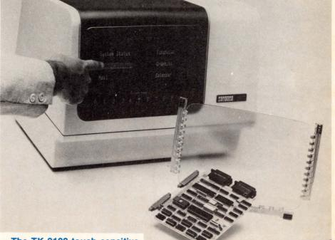
The TK-2100 touch-sensitive **CRT option for the DECTM** VT100TM by Interaction Systems, Inc. CLASSIFIED
