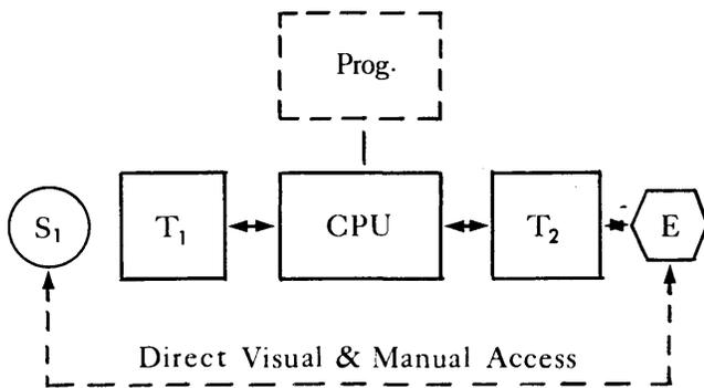
Figure 5. Arrangement incorporating "hands-on" student/equipment interaction with program monitoring.
