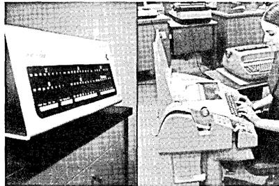
The central processor is an 8-bit computer, called the Wang 3300, with a 1.6 microsecond full cycle memory in 4K units expandable to 65K, binary and decimal arithmetic, a repertoire of 70 instructions, over 20 memory reference instructions, push/pop addressing system, both character bus and direct memory access I/O, and priority interrupt.
