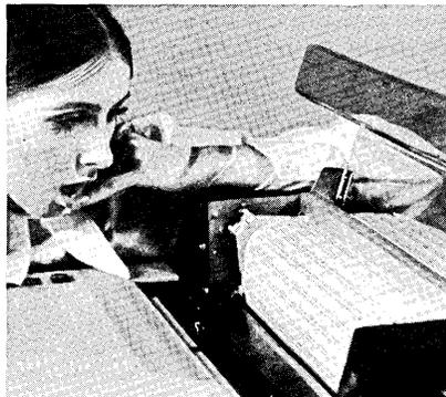
and line length are set to the computer industry norm (10 characters per inch and a line length of 136 characters). The character spacing is variable, however, from five to fifteen characters per inch allowing up to 204 characters on a single line. The device accommodates the 80 character line common in commun-
