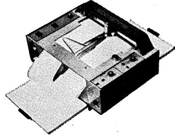
**DP-3** Digital Incremental Plotter with 22" wide plotting surface. Plots at 300 increments/sec. with .01" or .005" step size. Step size can be changed in minutes. Z-fold paper 22" wide x 144" is perforated for convenient tearout. DP-3 can be used online, offline or in time share mode. Accepts AC or DC coupled inputs. 5 year software plan included. Request Bulletin #868 DP-3.
