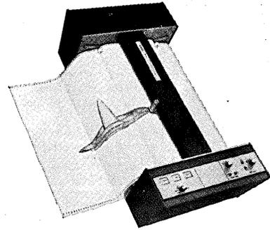
**DP-5** Ultra High Speed Digital Incremental Plotter for computer graphics. Plots at a continuous speed of 1200 increments/sec. Conventional (300 increments/sec.) programs can be used at approximately 4 times normal speed. Step size is factory set at .005" or .0025". DP-5 features 11" wide x 144" long Z-fold paper for operational convenience. May be used online or offline, and accepts AC or DC coupled inputs. House-keeping software for plotting for 5 years. Request Bulletin #269 DP-5.
