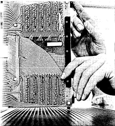
— Memory module: each module contains 4096 eight bit bytes. Modular concept allows Sigma 5 computers to be field-expanded to 131,072 words
