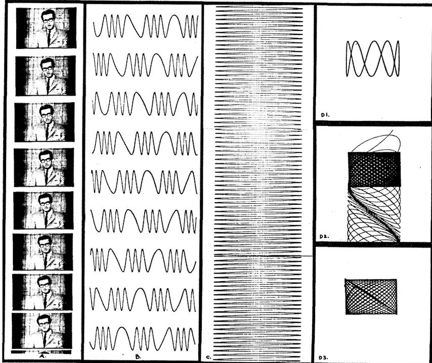
in the picture. Its capabilities include recording video pictures (A) in a series of individual frames; transverse (B) or longitudinal (C) recording of signals in a continuous mode; and combining both X and Y signals to obtain single 3x5-inch records (D1) or continuous records of X-Y plots and Lissajous patterns (D2 and D3).
