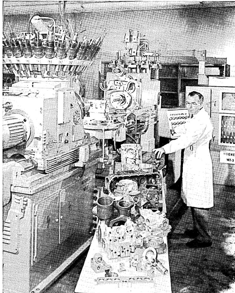
ventional single-purpose machines. Sample parts (in foreground) of aluminum, cast iron, steel and magnesium represent many industries including aerospace, automotive, industrial pumps, hydraulic assemblies and pneumatic assemblies. The universal drilling, tapping and boring head (upper left) not
