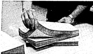
The finished stack is then taken to a padding station (photo, upper right) where a special penetrating adhesive is applied and the forms are allowed to dry. Then the padded stack is fanned apart (bottom) into unit sets with the simple flick of a thumb down the side of the padded stack. Forms are produced with the pre-collated paper in half the time it takes to make carbon-interleaved forms for approximately the same cost. (For more information, designate #41 on the Readers Service Card.)
