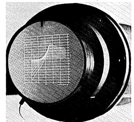
Magnetic tapes brought to the S-C 4020 are electronically converted into combinations of printed characters, lines and curves by use of a special cathode ray tube. Directly opposite the tube screen is a 16mm or 35mm recording camera and another optically aligned
