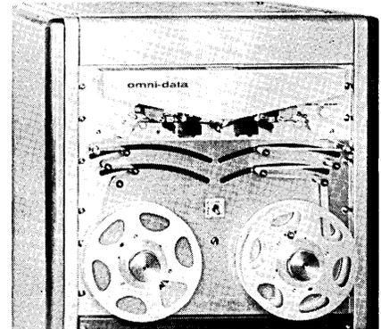
Double dancer arms on the new OMNI-DATA Model RS-500 (unidirectional with rewind) and Model RS-600 (bidirectional) reelers allow very high paper speeds without excessive back-and-forth motion of the arms. The new series is compatible with all OMNI-DATA readers and recorders and with all other paper-tape equipment. Both reelers normally accommodate NAB reels up to 8-inches in diameter.
