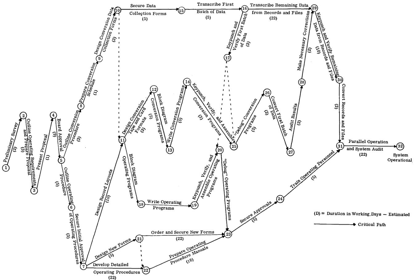
Figure 2 — Typical Critical Path Diagram, Showing Part of Computer Installation
