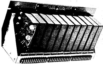
device transmits the total or net amount of these impulses to any one or a combination of the following: computer, data logger, telemetering equipment, printing demand meter, or other totalizer.
