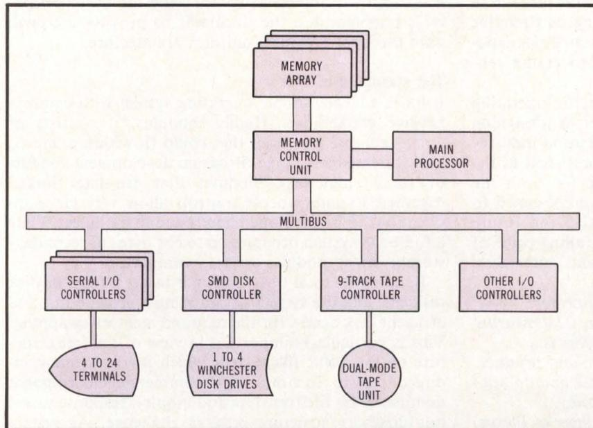
**Fig 1 Plexus P/40 block diagram. System relies on IEEE 796 bus (MULTIBUS) to communicate with its I/O device controllers. For greater speed, system memory is on separate bus.**
