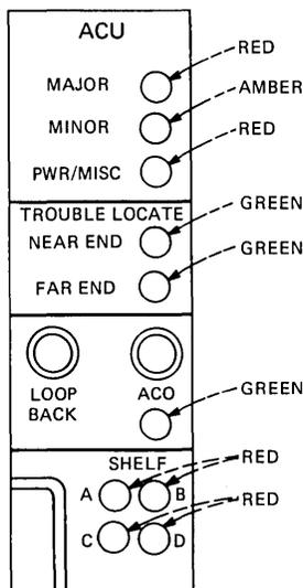
Fig. 2—Alarm control unit alarm indicators.
