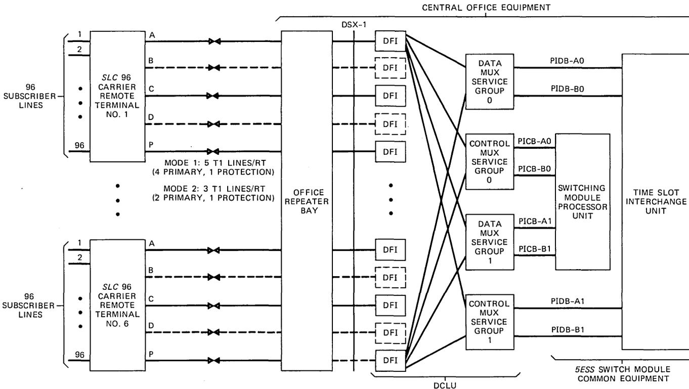
Fig. 5—5ESS switch digital carrier line unit with four PIDs to TSU.
