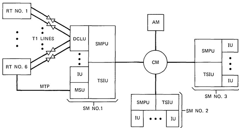
Fig. 1—5ESS switch equipped with digital carrier line unit.
