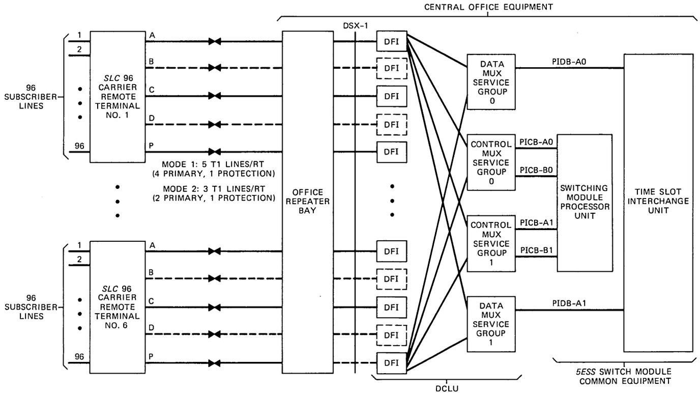
Fig. 4—5ESS switch digital carrier line unit with two PIDBs to TSIU.
