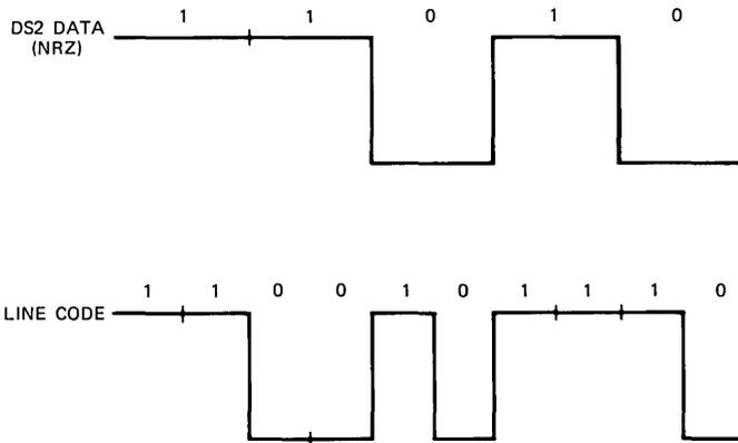
Fig. 9—Alternate dipulse coding.
