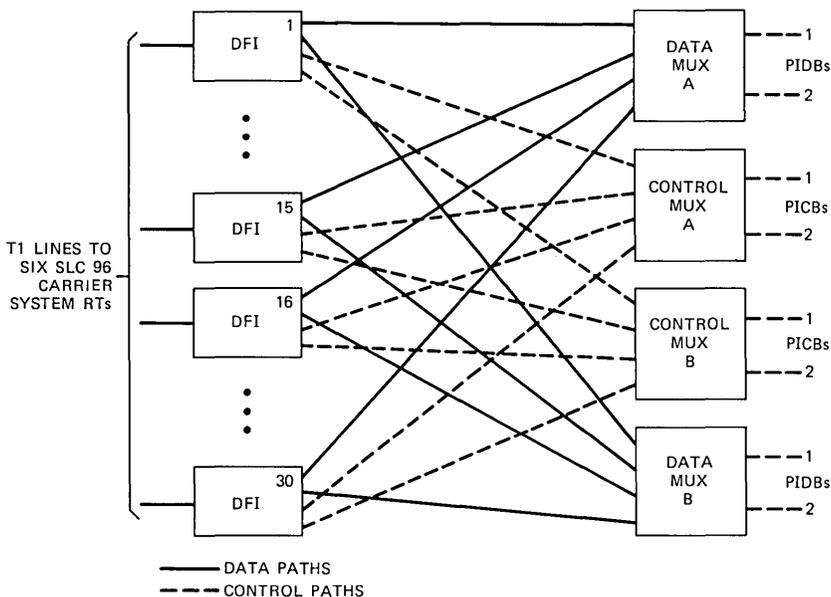
Fig. 2—5ESS switch digital carrier line unit.
