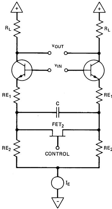
Fig. 14—Simplified circuit diagram of fixed-gain equalizing amplifier.
