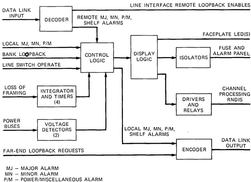
Fig. 14—Alarm control unit.
