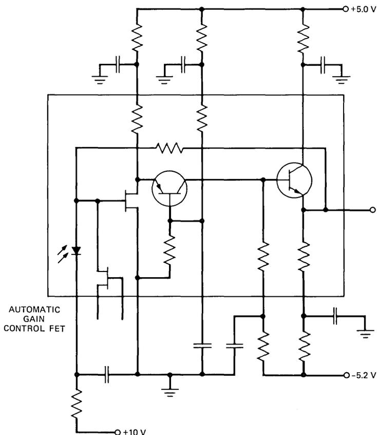
Fig. 5—1.3- $\mu\text{m}$  InGaAs PIN-GaAsFET receiver preamplifier.
