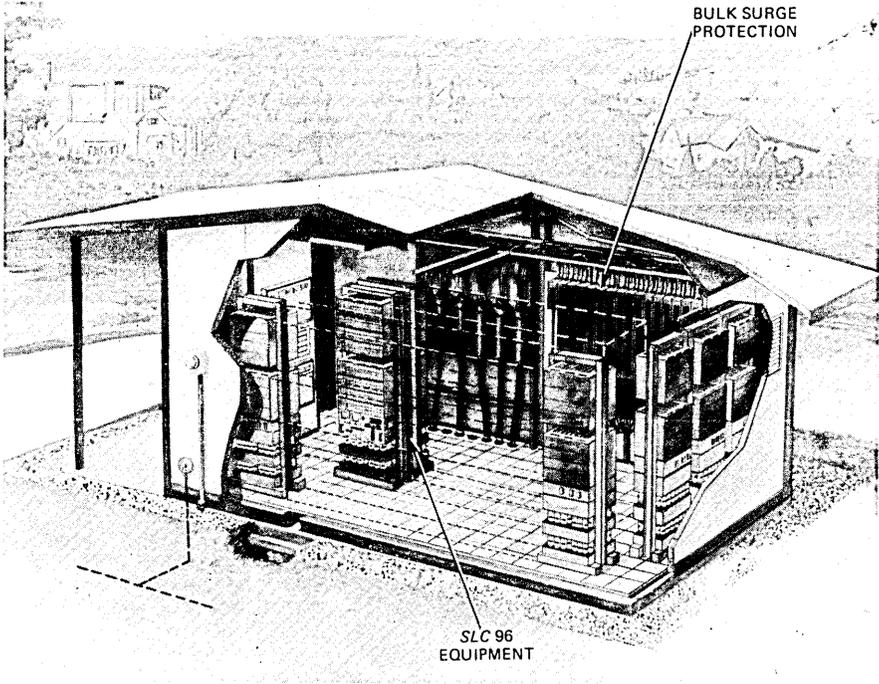
Fig. 18—Bulk surge protection arrangement in an electronic equipment enclosure.
