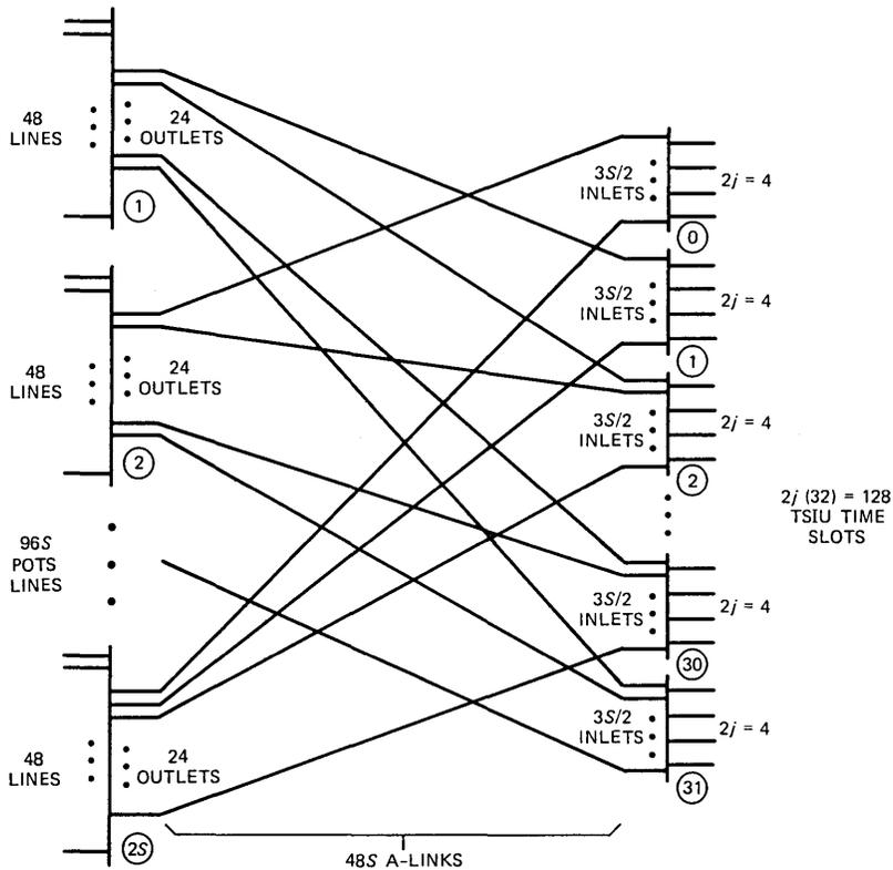
Fig. 7—RT and DCLU switching network topology with  $S(1 \leq S \leq 6)$  Mode 2 RTs and  $j = 2$  PIDBs to TSIU from each data multiplexer.
