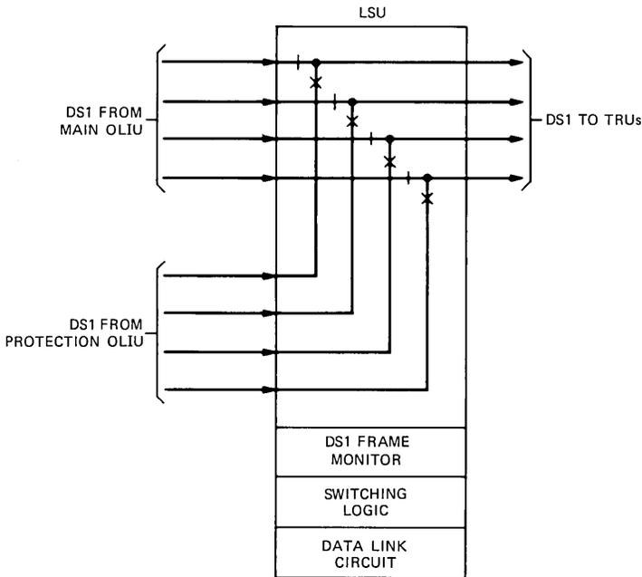
Fig. 10—Functional diagram of the line switch unit.
