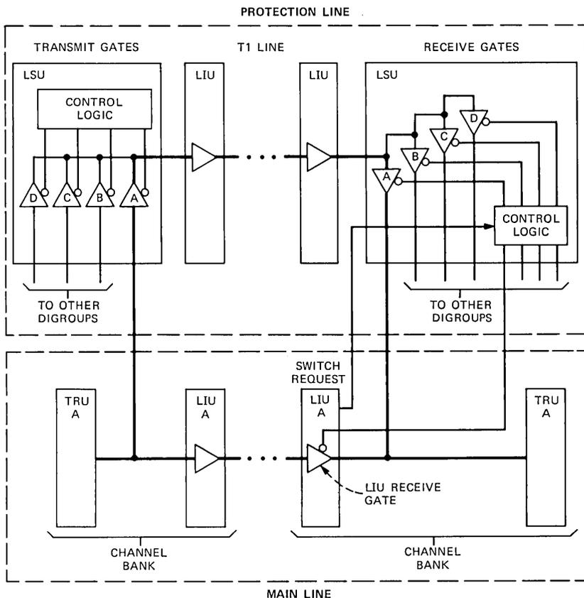
Fig. 12—Protection line switching with one direction shown.
