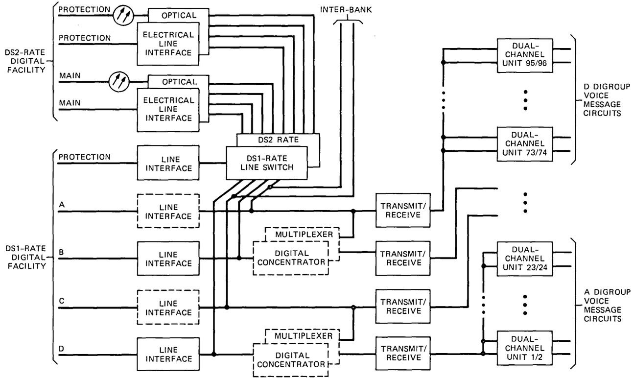
Fig. 1—SLC 96 carrier channel bank.
