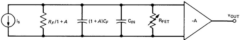
Fig. 15—Small signal representation of transimpedance preamplifier.
