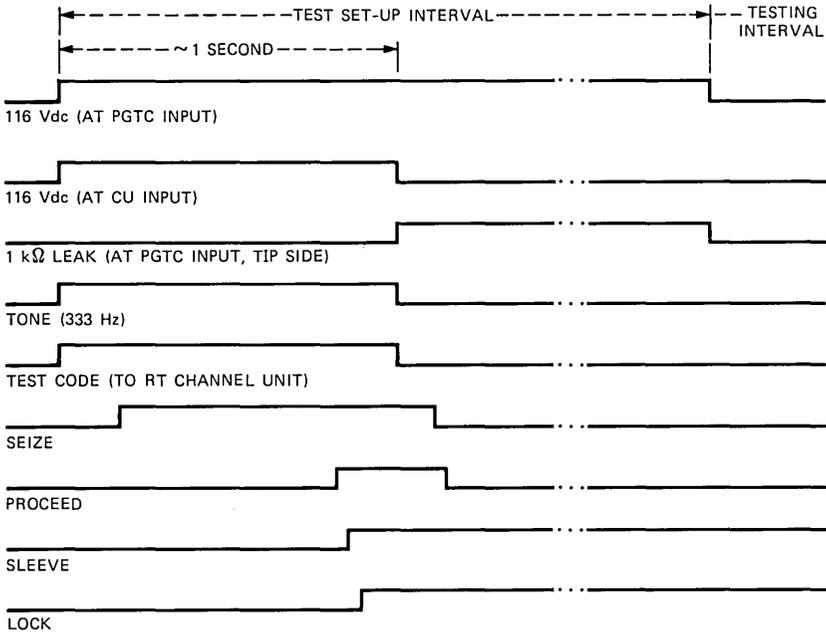
Fig. 16—Time sequence of events at interface between the PGTC and the COT channel test unit and channel unit under test.
