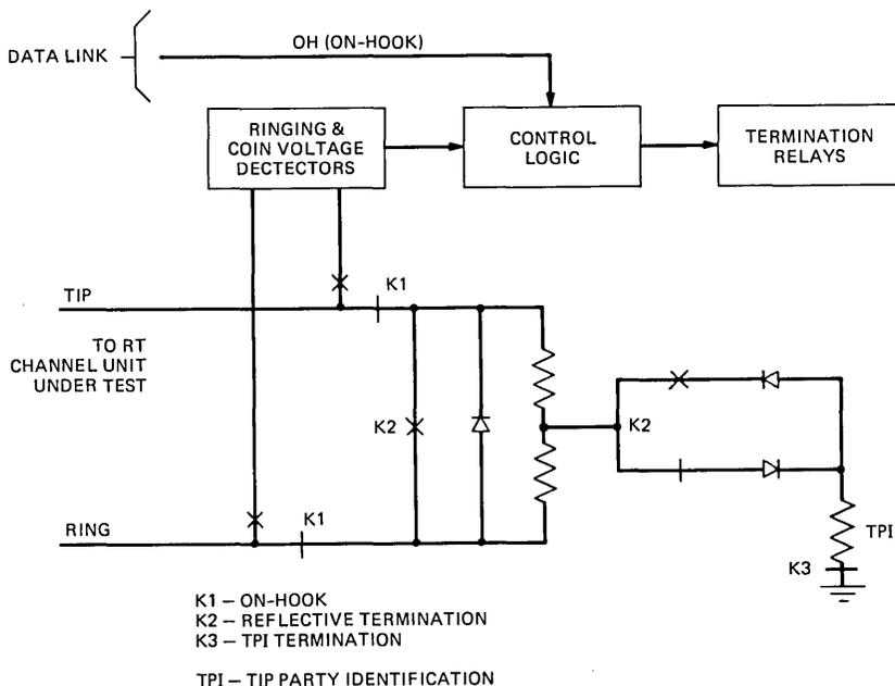
Fig. 6—Remote terminal termination circuit.
