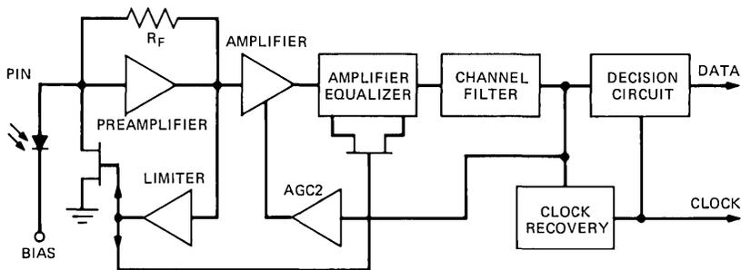
Fig. 12—Block diagram of an optical receiver.
