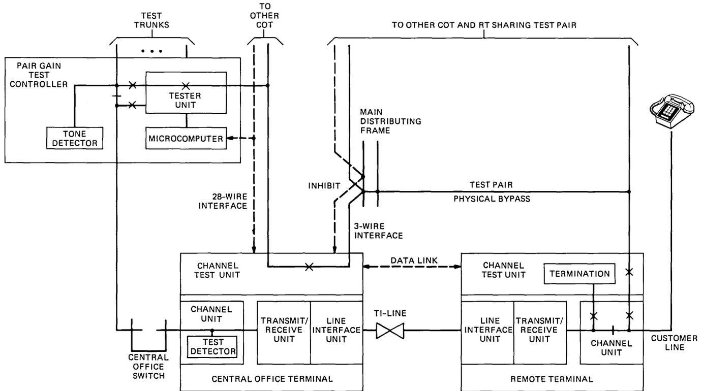
Fig. 3—Pair gain test controller interface to the SLC 96 carrier.
