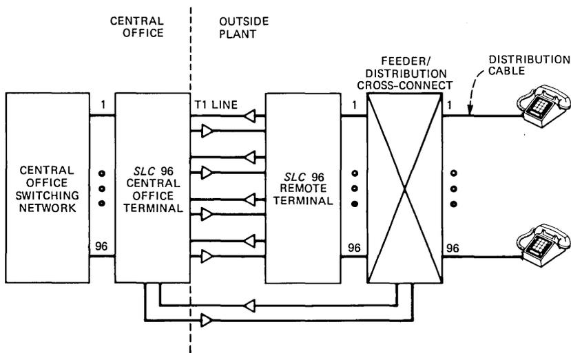
Fig. 1—*SLC 96* carrier system configuration.
