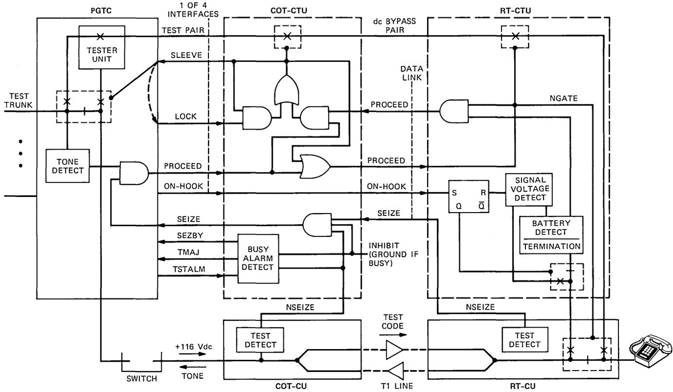
Fig. 15—Simplified schematic of COT and RT channel test units.
