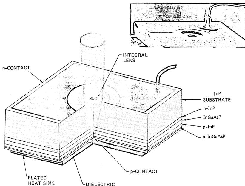
Fig. 1—Schematic illustration of surface-emitting 1.3- $\mu\text{m}$  LED with an integral lens. Inset is a scanning electron micrograph of a bonded LED chip.
