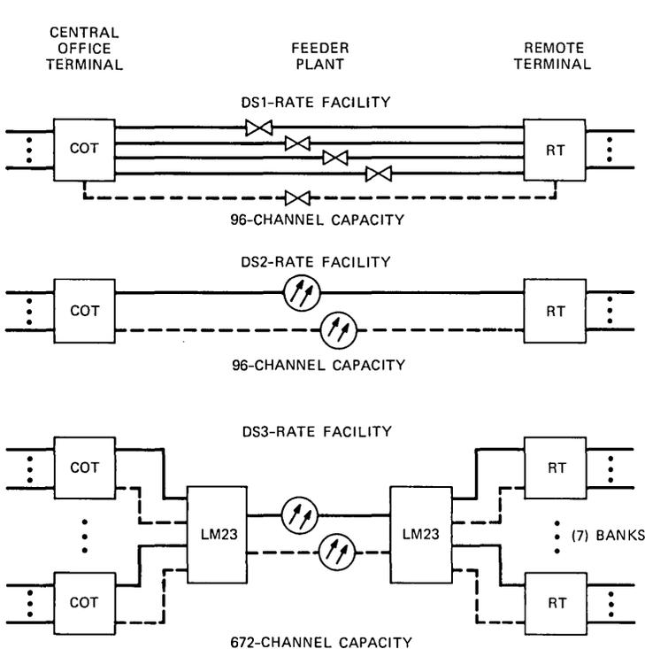
Fig. 3—SLC 96 carrier channel bank interfaces—Mode 1.
