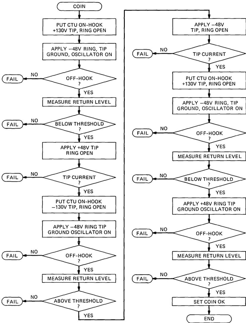
Fig. 9—Coin unit test sequence.
