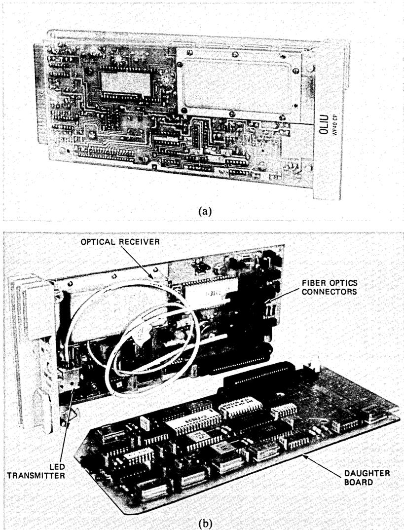
Fig. 9—Optical line interface unit: (a) assembled, and (b) unassembled.
