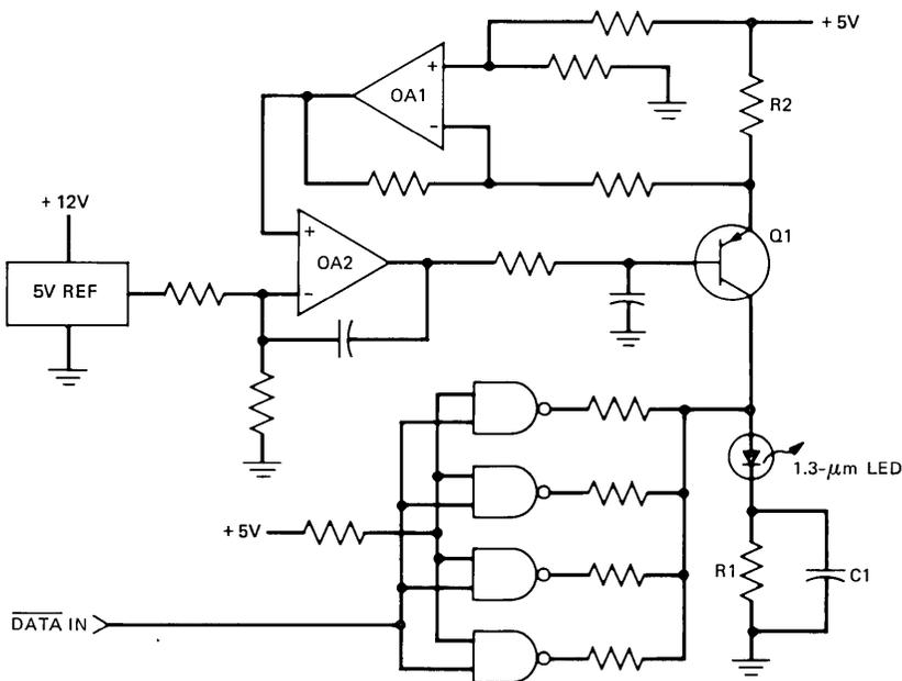
Fig. 11—Simplified circuit diagram of the LED transmitter.
