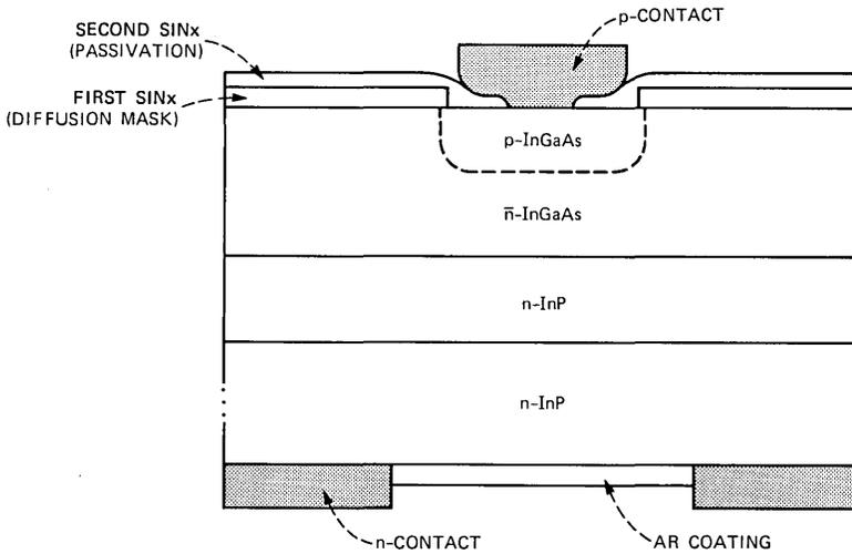
Fig. 4—Planar InGaAs PIN diode structure.
