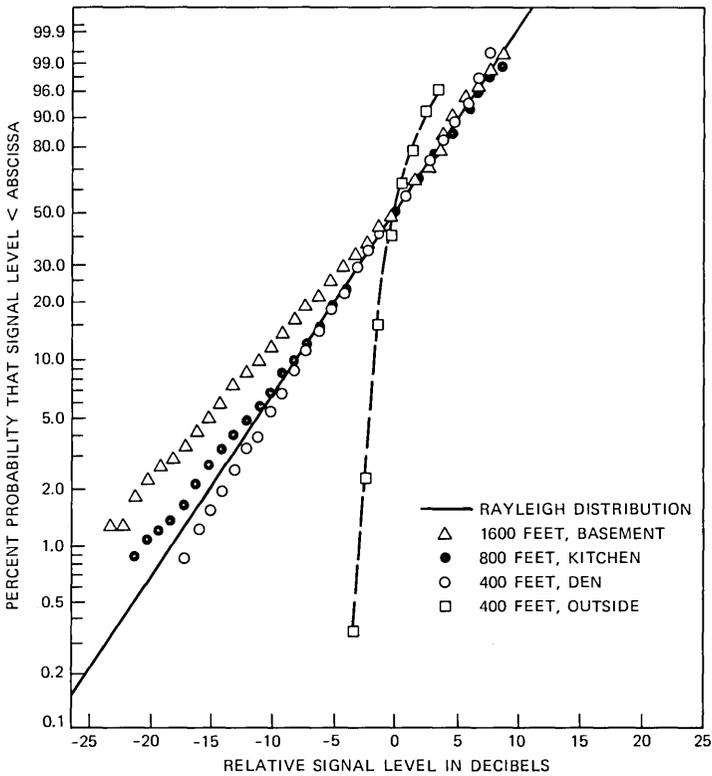
Fig. 5—Measured signal envelope distributions from four small (4-ft square) areas. On these coordinates, Rayleigh distributions are straight lines with the slope indicated. Distances between the van and the measurement location are indicated in the key.
