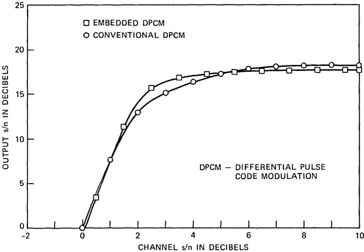
Fig. 5—A 24-kb/s speech transmission with a rate of 2/3 code (Format 3) used to summarize performance differences between embedded and conventional DPCM.
