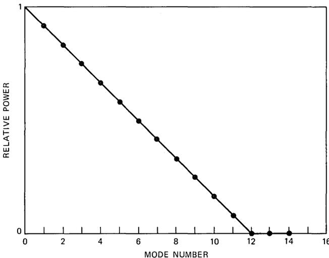
Fig. 7—A plot of the tapered modal-power distribution.
