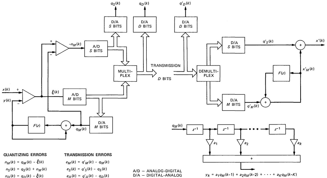
Fig. 6—The signal-processing operations of Fig. 2 and the notation used to analyze them. Three new digital-to-analog converters define signals that appear in the analysis.
