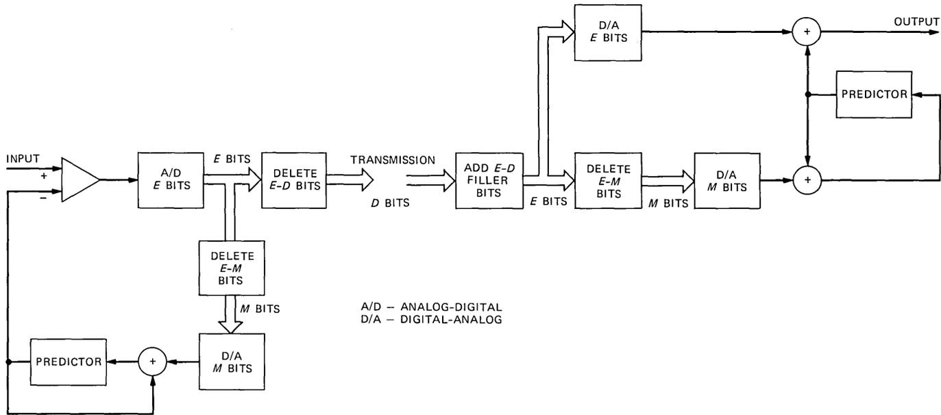
Fig. 1—Embedded DPCM encoder and decoder. Because both predictors operate on the same signal (with resolution  $M$  bits/sample) performance is unaffected by errors due to bit-rate adjustment. The channel can transmit between  $M$  bits/sample and  $E$  bits/sample.
