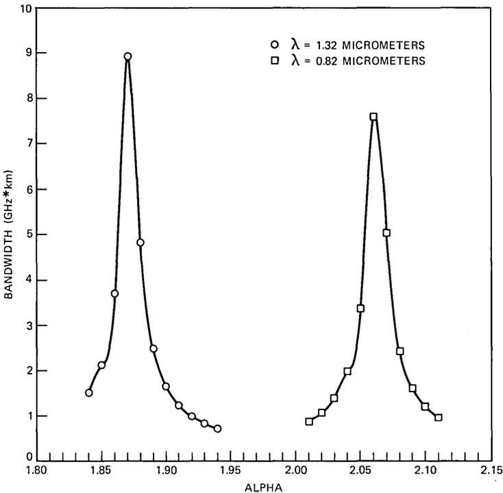
Fig. 10—Plots of bandwidth versus  $\alpha$  for  $\lambda = .82 \mu\text{m}$  and  $\lambda = 1.32 \mu\text{m}$  assuming equal excitation of modes having less than 0.1 percent power in cladding.
