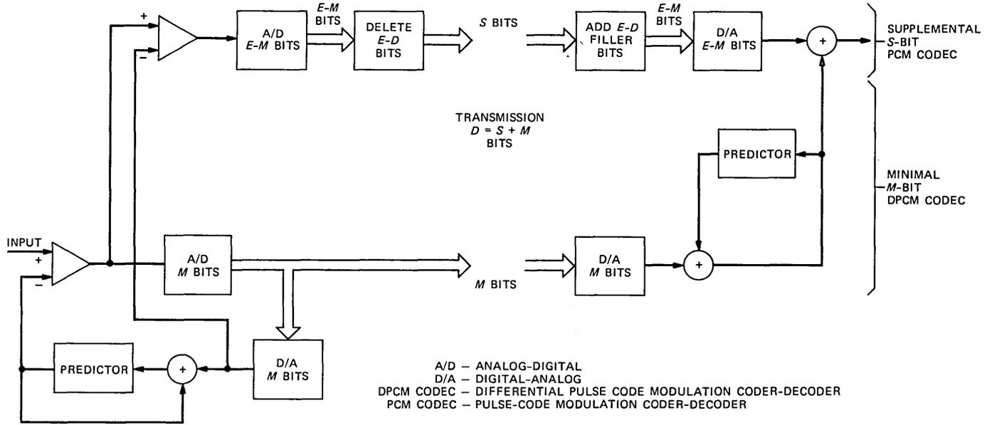
Fig. 2—Embedded DPCM encoder and decoder.  $E$ -bit analog-to-digital conversion is shown as a two-stage, successive-approximation process. All  $M$  minimal bits are transmitted.  $S$ , the number of supplemental bits transmitted, can range from 0 to  $E-M$ .
