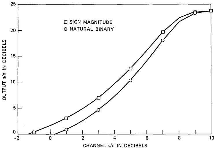
Fig. 8—Performance of embedded DPCM with sign-magnitude and natural-binary representations of quantizer outputs.
