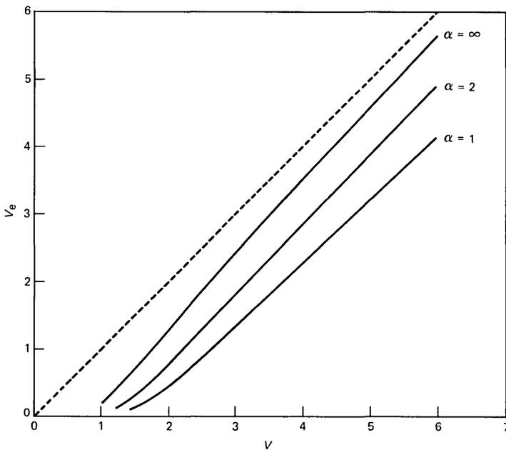
Fig. 16—Plots of  $V_e$  versus  $V$  for the  $HE_{11}$  mode of three power-law profiles.
