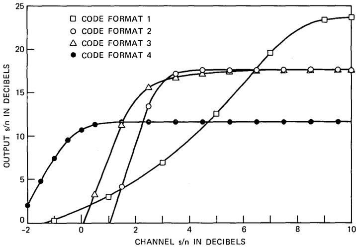
Fig. 3—Performance of embedded DPCM in four transmission environments.
