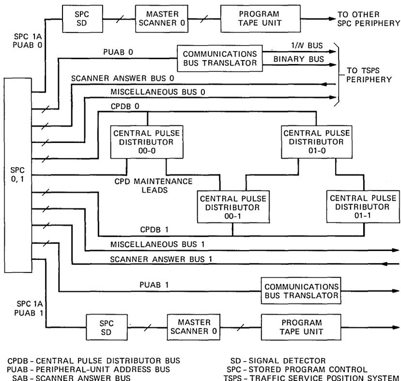
Fig. 2—TSPS No. 1 peripheral buses.
