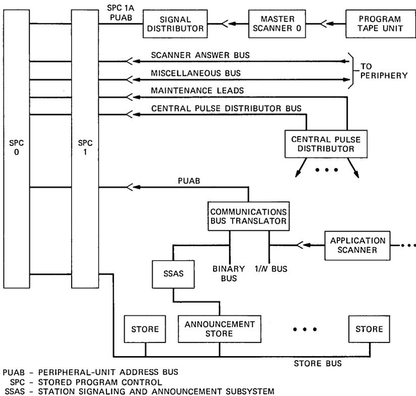
Fig. 3—Connectorized TSPS buses.
