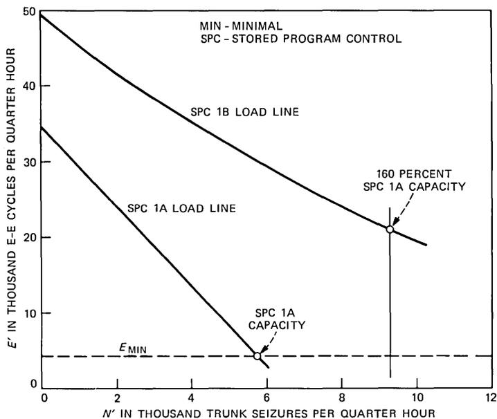
Fig. 5—Comparison between SPC 1A and SPC 1B load lines.
