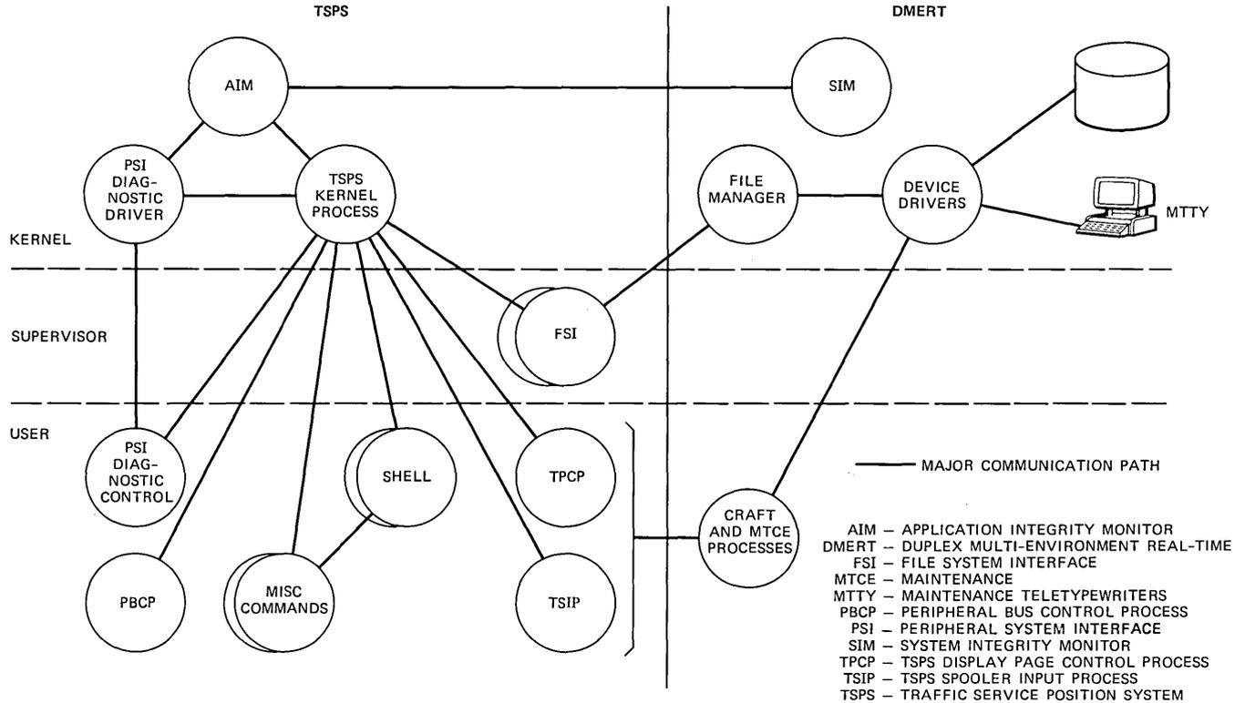
Fig. 13—Interaction between TSPS and DMERT processes in TSPS No. 1B process architecture.
