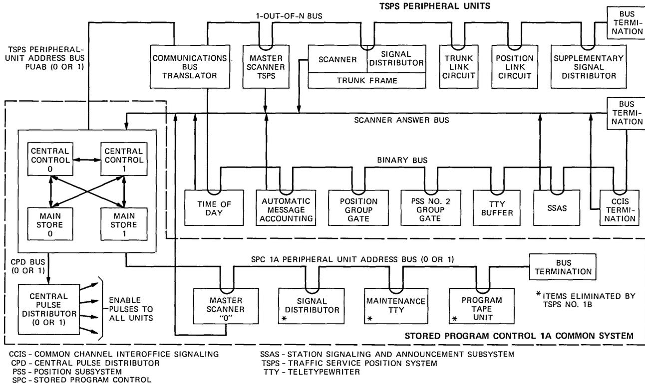
Fig. 2—Traffic Service Position System No. 1.
