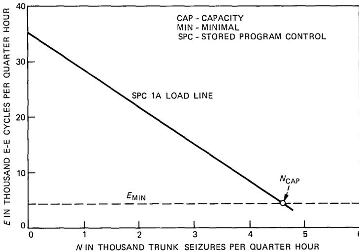
Fig. 1—Typical SPC 1A load line.
