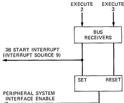
Fig. 5—Start and stop signals from SPC 1A.
