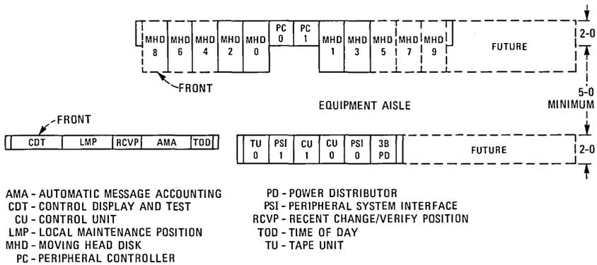
Fig. 12—Typical floor plan for TSPS No. 1B.
