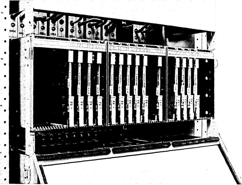
Fig. 9—Peripheral System Interface frame logic unit with circuit packs.
