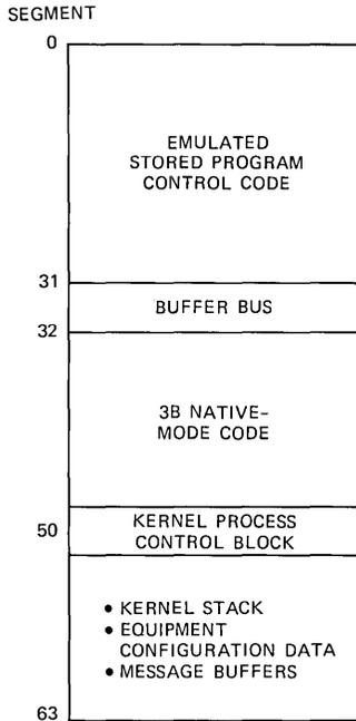
Fig. 9—Virtual address space in the TSPS process.
