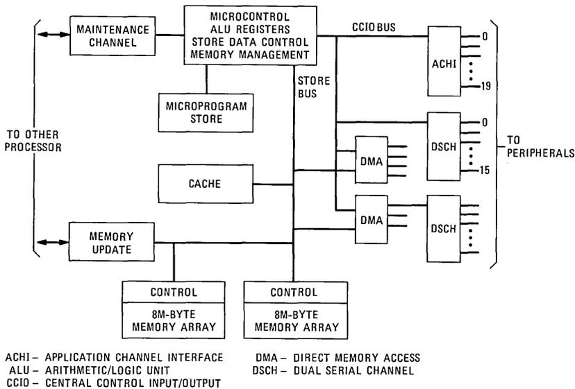
Fig. 3—3B Processor block diagram.
