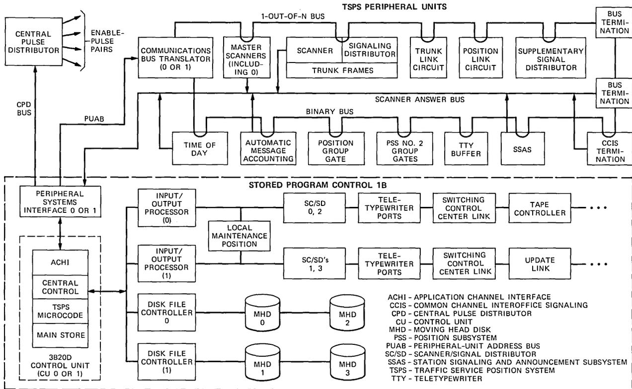
Fig. 3—The SPC 1B Processor and peripheral architecture.
