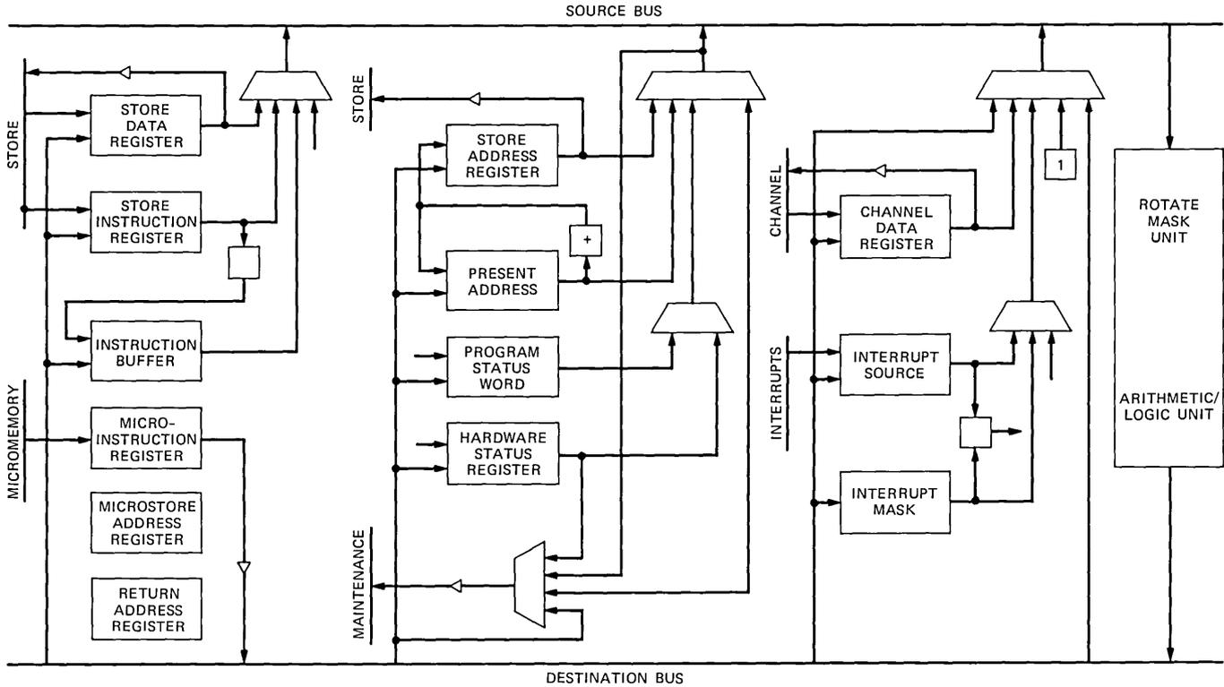
Fig. 5—Processor control architecture.
