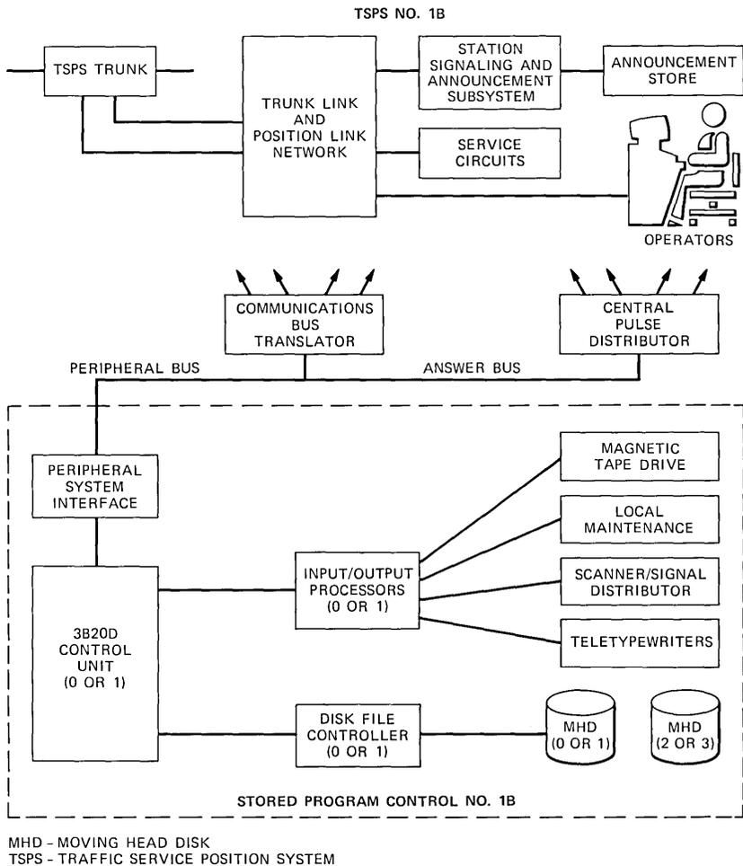
Fig. 1—Traffic Service Position System No. 1B.
