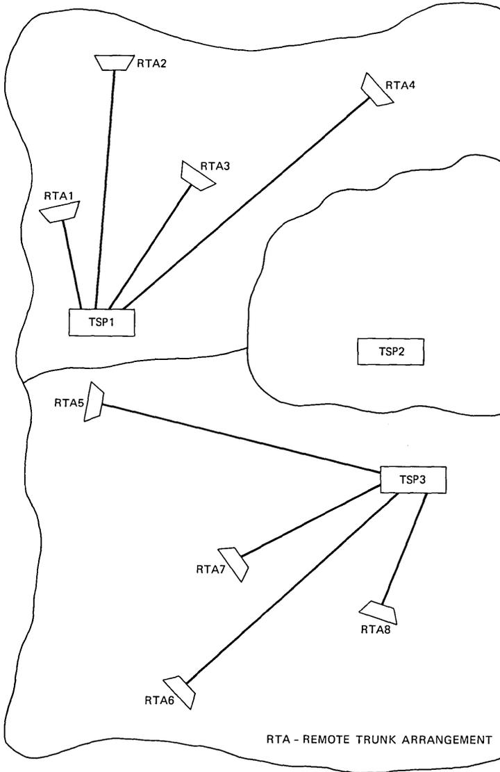
Fig. 5(a)—TSPS/RTA configuration before user move.
