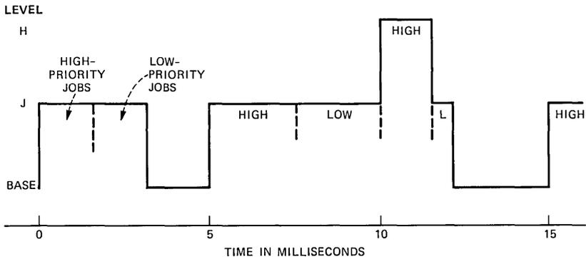
Fig. 1—5-ms input/output processing.
