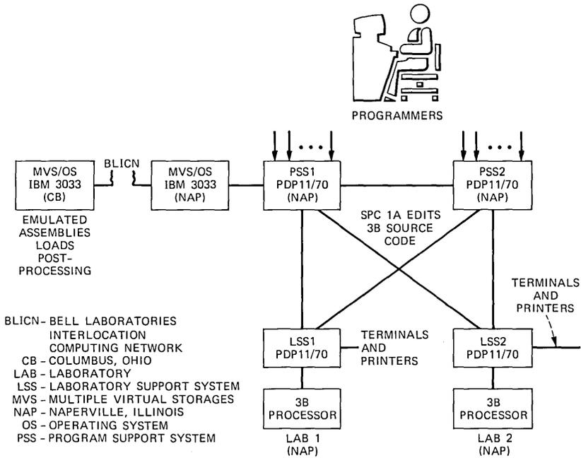
Fig. 1—Software Development System for TSPS No. 1B.
