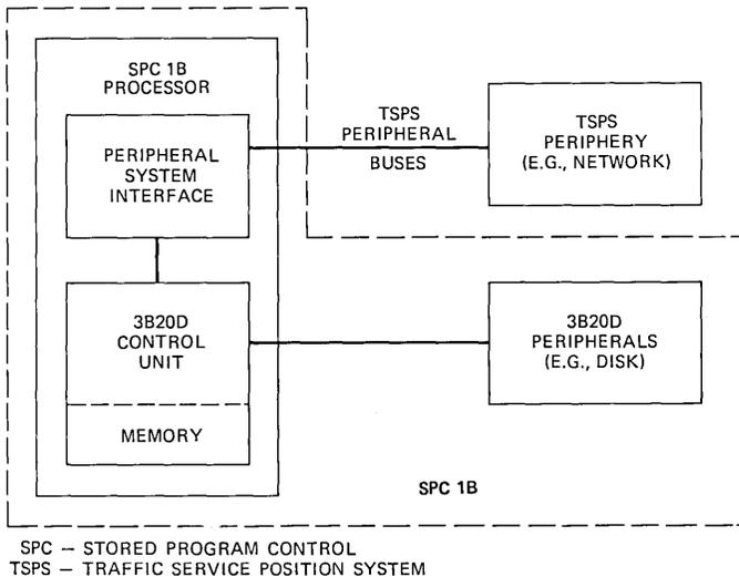
Fig. 2—TSPS No. 1B system structure.
