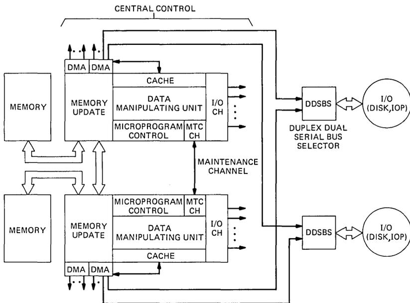
Fig. 1—General block diagram of the 3B20 Processor.
