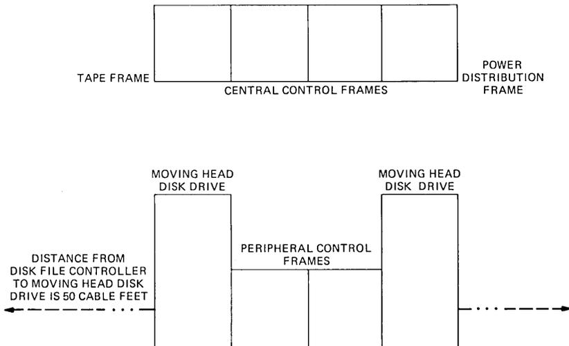
Fig. 4—Recommended floor plan for the 3B20D Processor.
