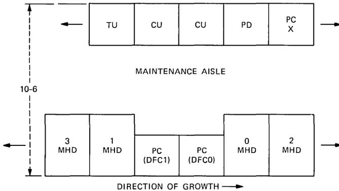
Fig. 5—Typical floor plan of the 3B20D Processor.
