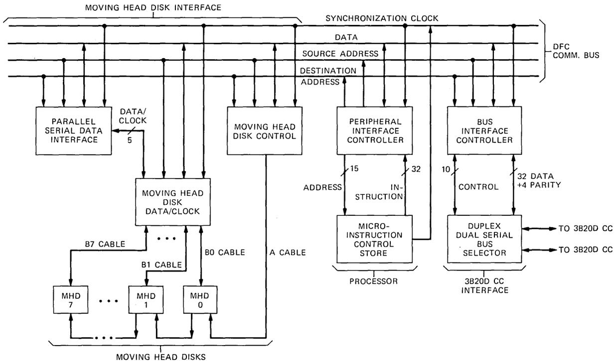
Fig. 7—Disk system block diagram.
