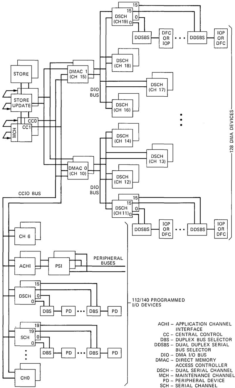
Fig. 4—The 3B20D Processor input/output architecture.
