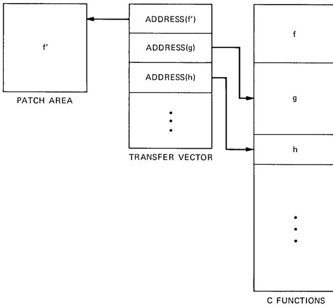
Fig. 6—Function *f* replaced by function *f'*.
