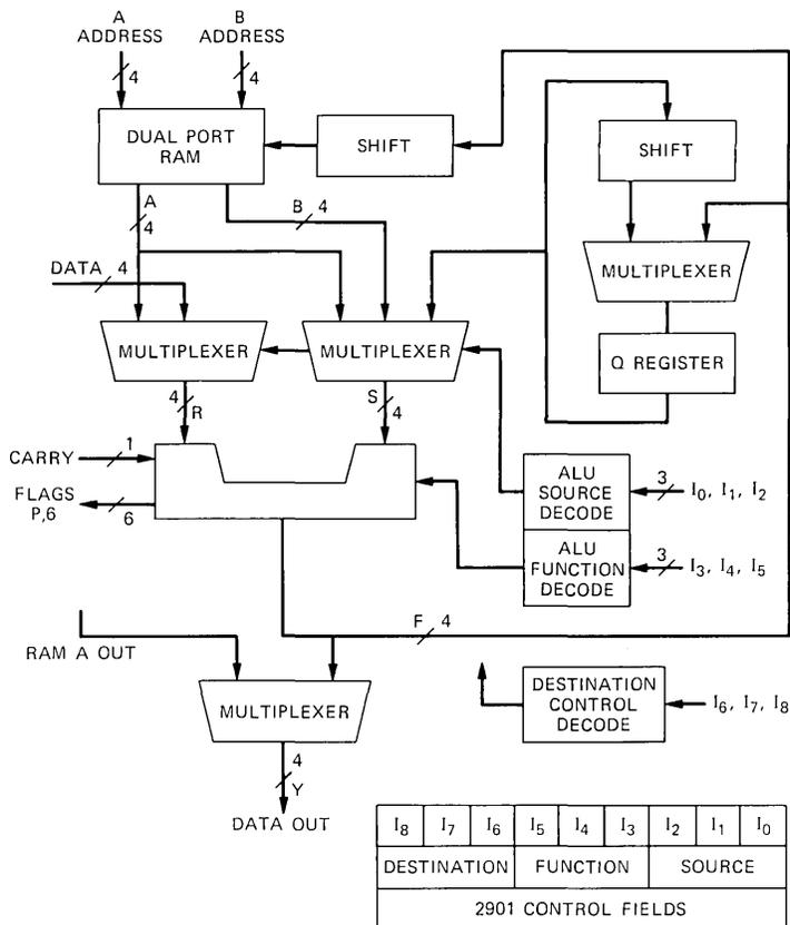
Fig. 3—The 2901 internal architecture.
