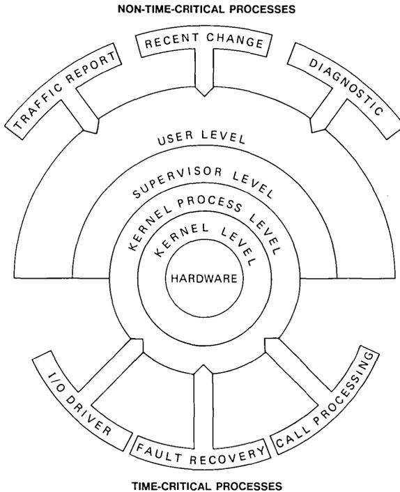
Fig. 3—Example of DMERT multienvironment structure.
