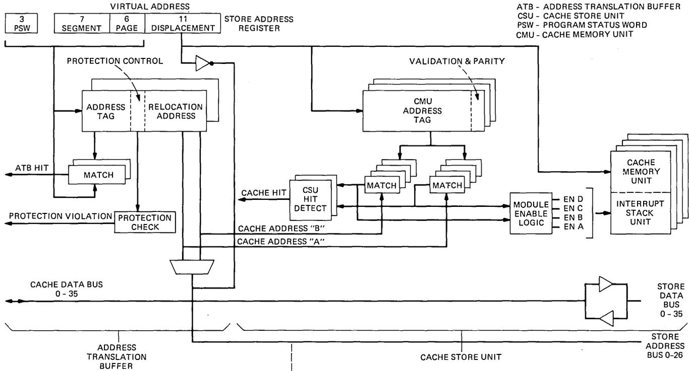
Fig. 2—Block diagram of the 3B20D Processor store address translator and cache store unit.
