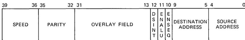
Fig. 8—Microinstruction of the peripheral interface controller.
