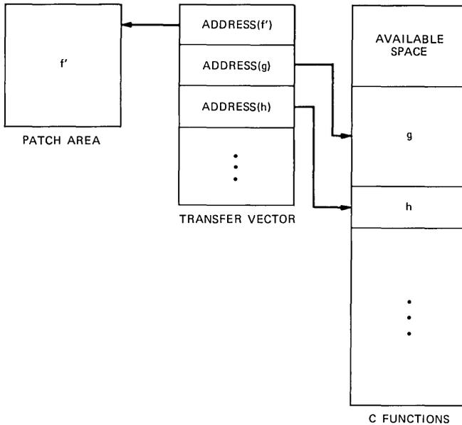
Fig. 7—Reclaiming the space occupied by function f.
