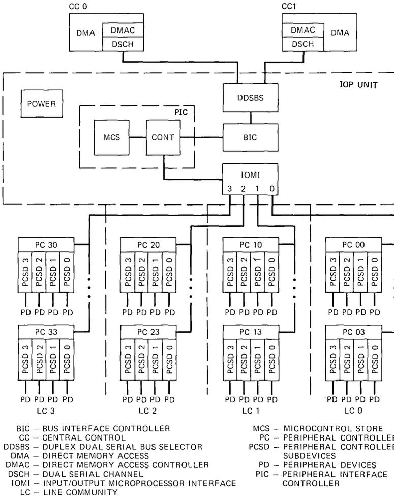
Fig. 1—Input/output processor.
