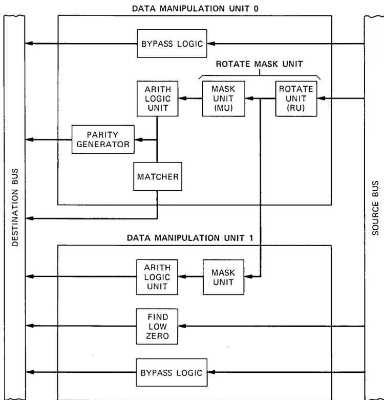
Fig. 2—Block diagram of the data manipulation unit.
