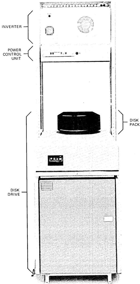
Fig. 1—Moving head disk frame.
