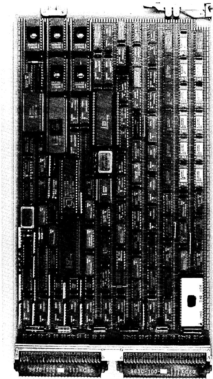
Fig. 3—Typical one-board peripheral controller design.
