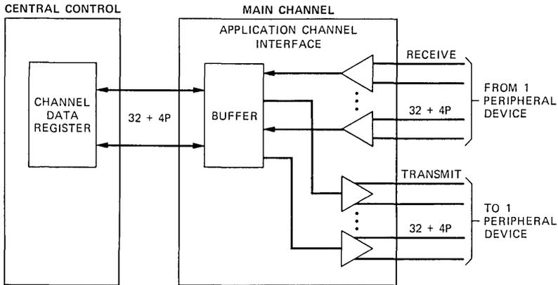
Fig. 6—Application channel interface.
