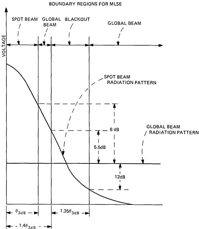
Fig. 11—One-dimensional plot showing the usable regions attainable via MSLE for a hybrid spot-area beam satellite system employing a  $K = 7, r = 1/2$  code for the area beam transmission. The spot beam antenna pattern is Gaussian shaped.
