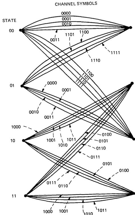
Fig. 4—State diagram for maximum-likelihood detection of interfering coded and uncoded signals. A  $K = 3$ ,  $r = 1/2$  convolutional code is assumed. For each transition, the first two channel digits correspond to the coded symbols, and the second two correspond to the uncoded symbols.
