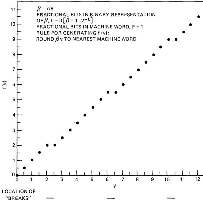
Fig. 2—An example of a naive machine arithmetic.
