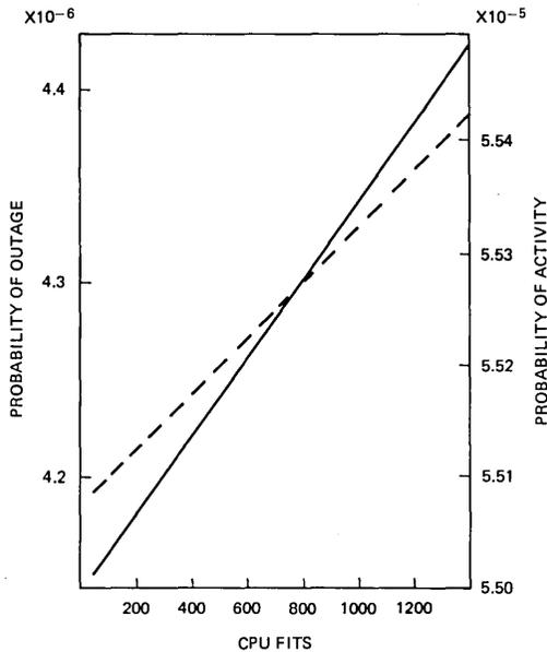
Fig. 5—Probabilities of outage and activity as functions of CPU failure rate.
