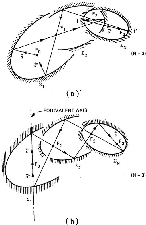
Fig. 4—(a)  $2N$  successive reflections. (b) The central path. The equivalent axis through  $F_0$  is obtained by varying in (a) the initial direction  $\vec{s}$  until  $\vec{s} = \vec{s}''$  as shown in (b).
