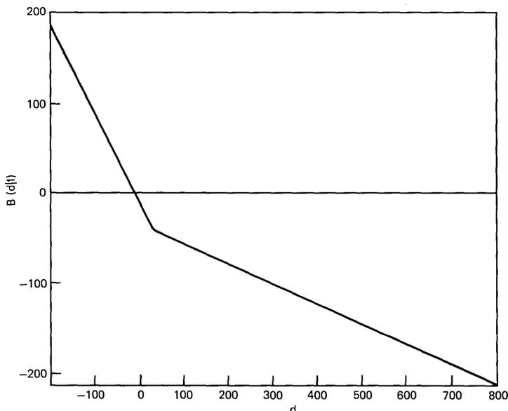
Fig. 6—The bias function for uniform 16-level quantizer and normally distributed input signal variables,  $\sigma = 1$ . Interleaving interval,  $I = 16$  and  $\gamma = 0.777$ . The log multipliers are given in (39).
