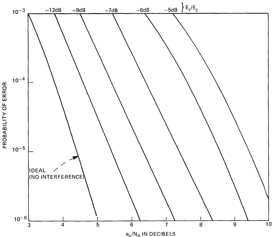
Fig. 10—Measured bit error rate performance of a  $K = 7$ ,  $r = 1/2$  convolutional code vs  $e_b/N_0$  for select values of interference. The interference is bit-synchronous with the encoded channel bits, and the ordinary Viterbi algorithm with soft (3-bit) quantization is employed.
