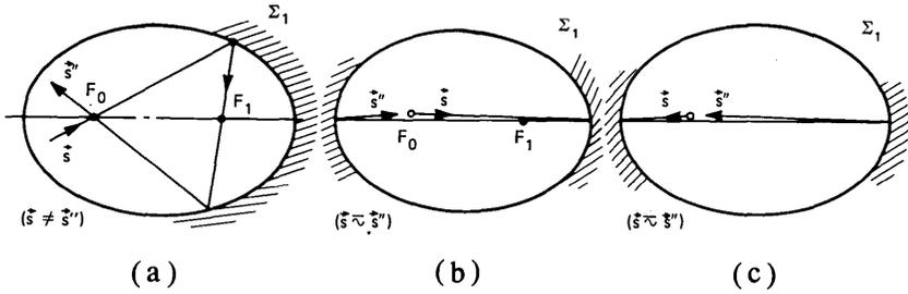
Fig. 3—The axis of  $\Sigma_1$  is determined by varying  $\bar{s}$  until  $\bar{s} = \bar{s}''$ .
