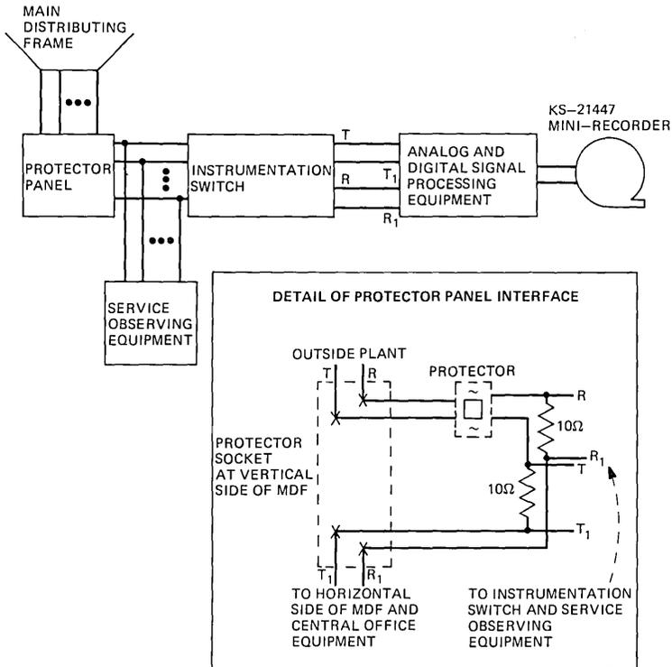
Fig. 19—Loop signal power survey data acquisition console.
