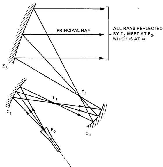
Fig. 2—The spherical wave from  $F_0$  is transformed into a plane wave by three confocal reflectors. The  $n$ th reflector transforms the spherical wave from  $F_{n-1}$  into a spherical wave converging towards  $F_n$ .
