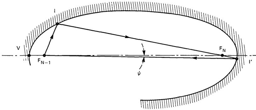
Fig. 5—As the distance of  $F_N$  from the other focus  $F_{N-1}$  is increased, keeping  $V$  and  $F_{N-1}$  fixed, the ellipsoid approaches a paraboloid with vertex  $V$  and focus  $F_{N-1}$ ; for the ray reflected at  $I'$  one has  $\psi \rightarrow 0$ .
