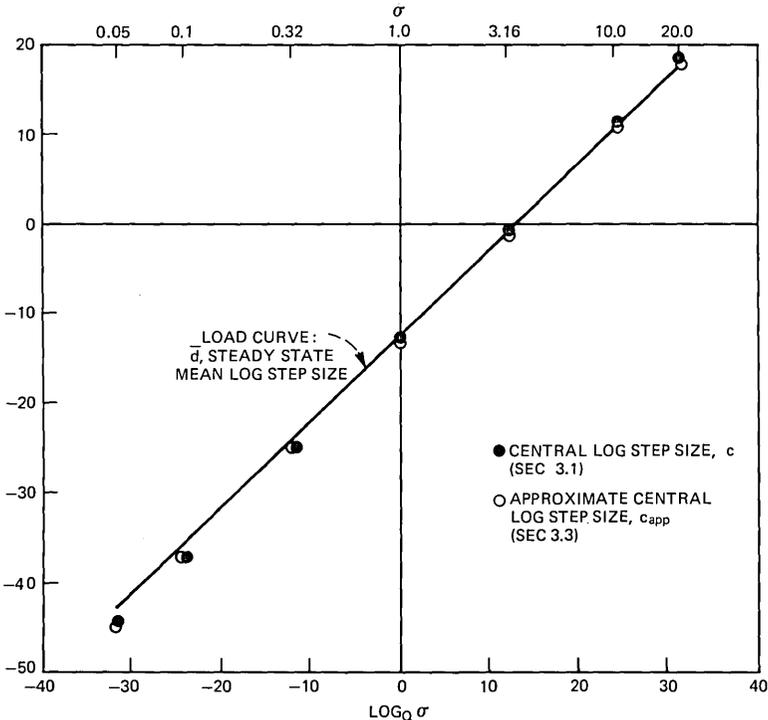
Fig. 7—Load curve ( $\bar{d}$ ), central log step size ( $c$ ), and approximate log step size ( $c_{app}$ ) for uniform 16-level quantizer and Gaussian, zero-mean, input signal variables of variance  $\sigma^2$ . The log multipliers are given in (39) and  $Q = 1.1$ . Interleaving interval,  $I = 16$  and leakage,  $\gamma = 0.777$ .
