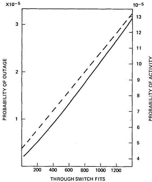
Fig. 4—Probabilities of outage and activity as functions of through switch failure rate.
