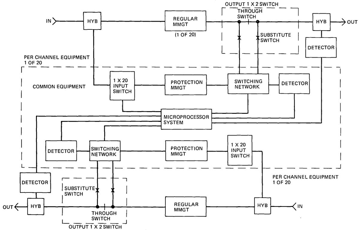
Fig. 1—TPSS block diagram.
