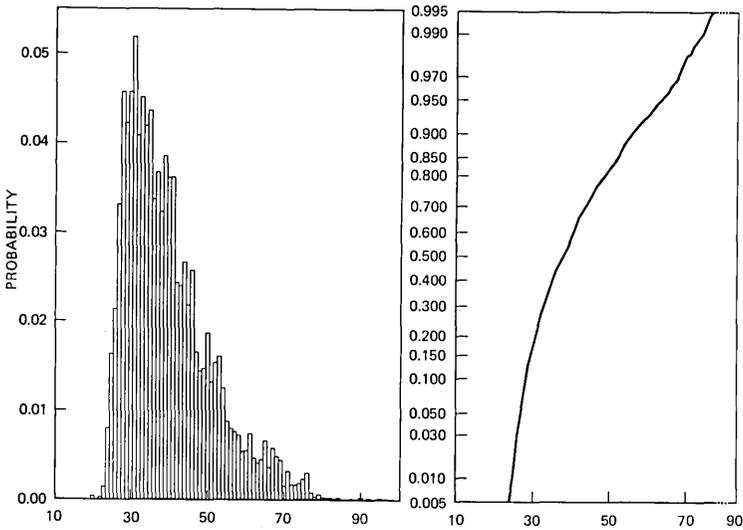
Fig. 14—Near-end loop current (mA) distribution for residential.
