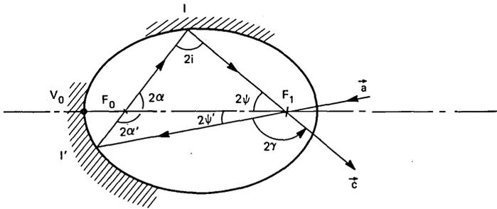
Fig. 15—Two successive reflections by a concave ellipsoid.
