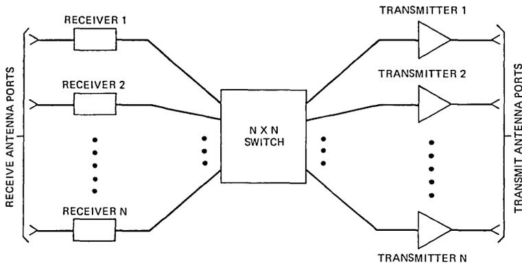
Fig. 1—Satellite transponder.
