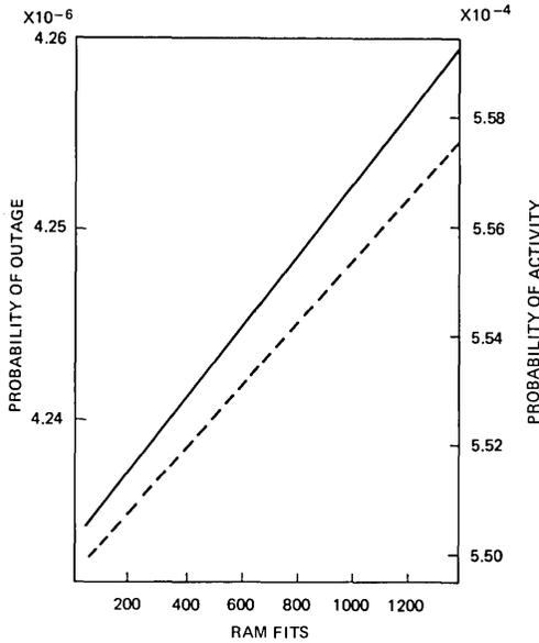
Fig. 7—Probabilities of outage and activity as functions of RAM failure rate.
