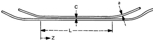
Fig. 1—Parallel waveguide directional coupler where  $a$  is guide width,  $c$  is the guide spacing, and  $L$  is the interaction length.
