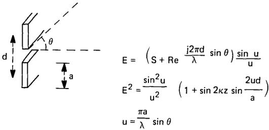
Fig. 2—Radiation field amplitudes under far-field conditions due to a pair of sources of width  $a$ , separated by a distance  $d$ .  $\theta$  is measured in the plane perpendicular to the plane containing the waveguides.
