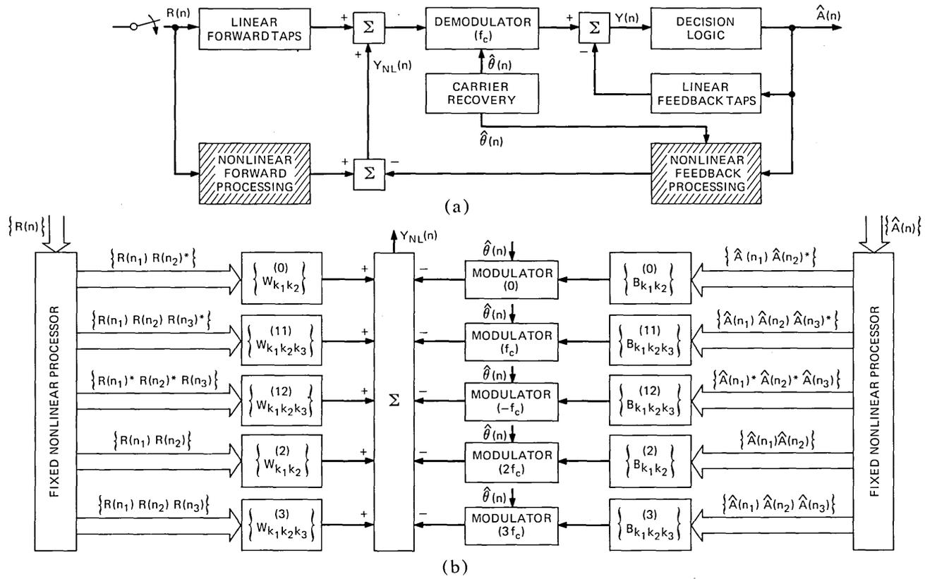
Fig. 3—(a) Basic structure of the NL receiver. (b) Details of the nonlinear signal processing.
