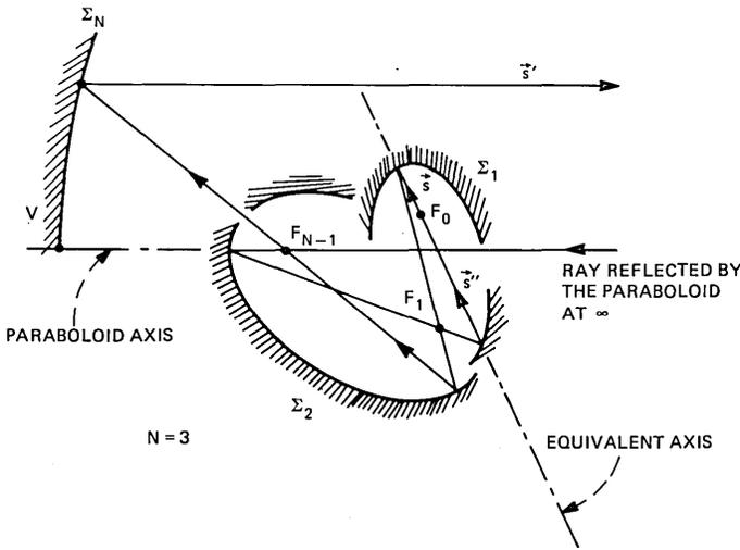
Fig. 6—By tracing from  $\infty$  the path of the ray defined by the paraboloid axis one obtains after  $N - 1$  reflections the equivalent axis through  $F_0$ . If a symmetrical feed is placed at  $F_0$ , centered around the equivalent axis, a symmetrical pattern will be reflected by the paraboloid.
