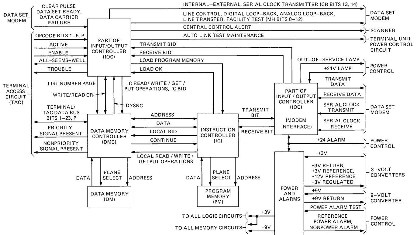
Fig. 11—Terminal unit block diagram.
