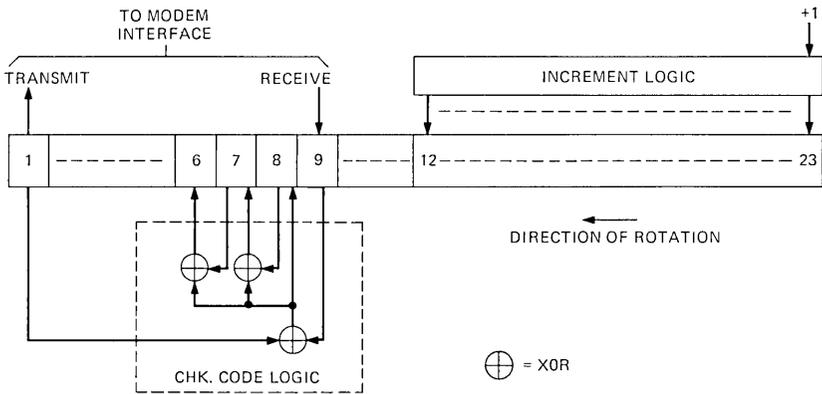
Fig. 13—Logic register layout and check code generation.
