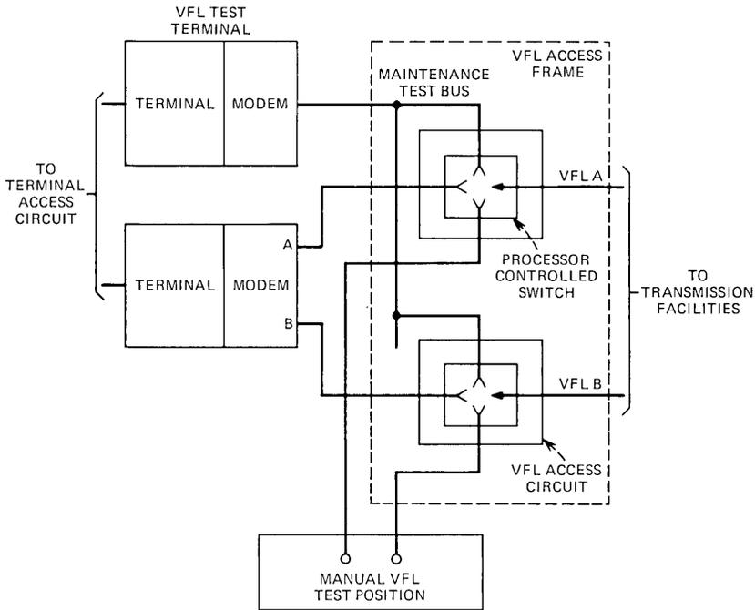
Fig. 2—STP VFL arrangement and dual VFL configuration.
