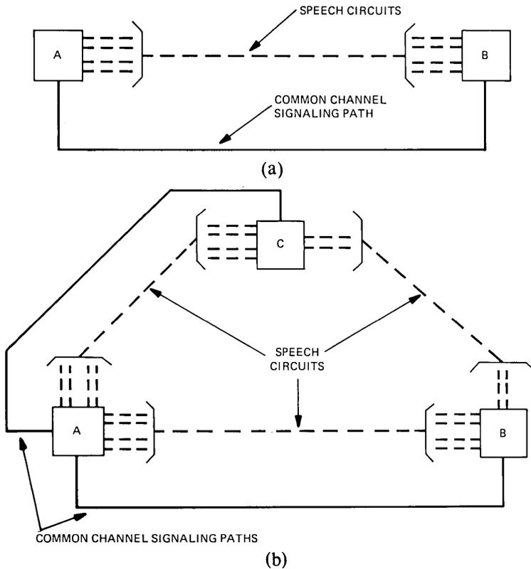
Fig. 2—(a) Associated signaling. (b) Nonassociated signaling.
