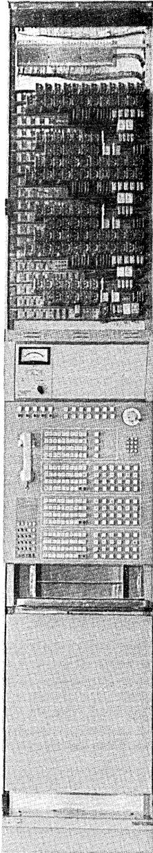
Fig. 33—CCIS intra-office trunk test frame.
