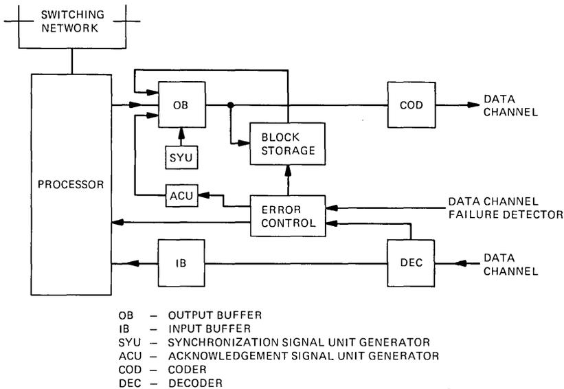
Fig. 6—Functional block diagram of a CCIS terminal.
