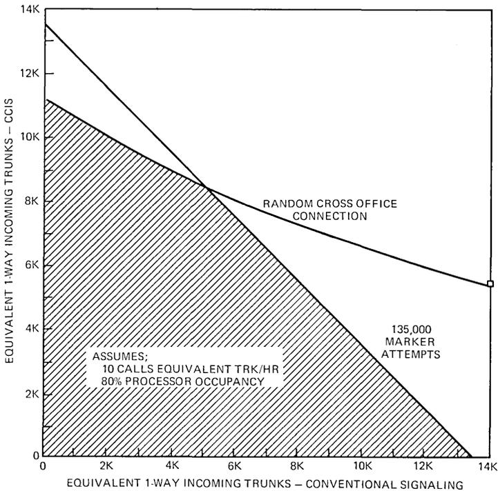
Fig. 5—4A/CCIS switching office equivalent one-way incoming trunk capacity. Cross-hatch indicates operating region.
