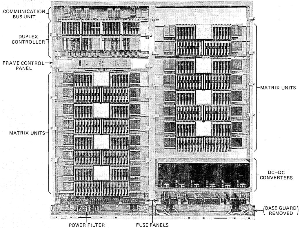
Fig. 21—Distributor and scanner frame.
