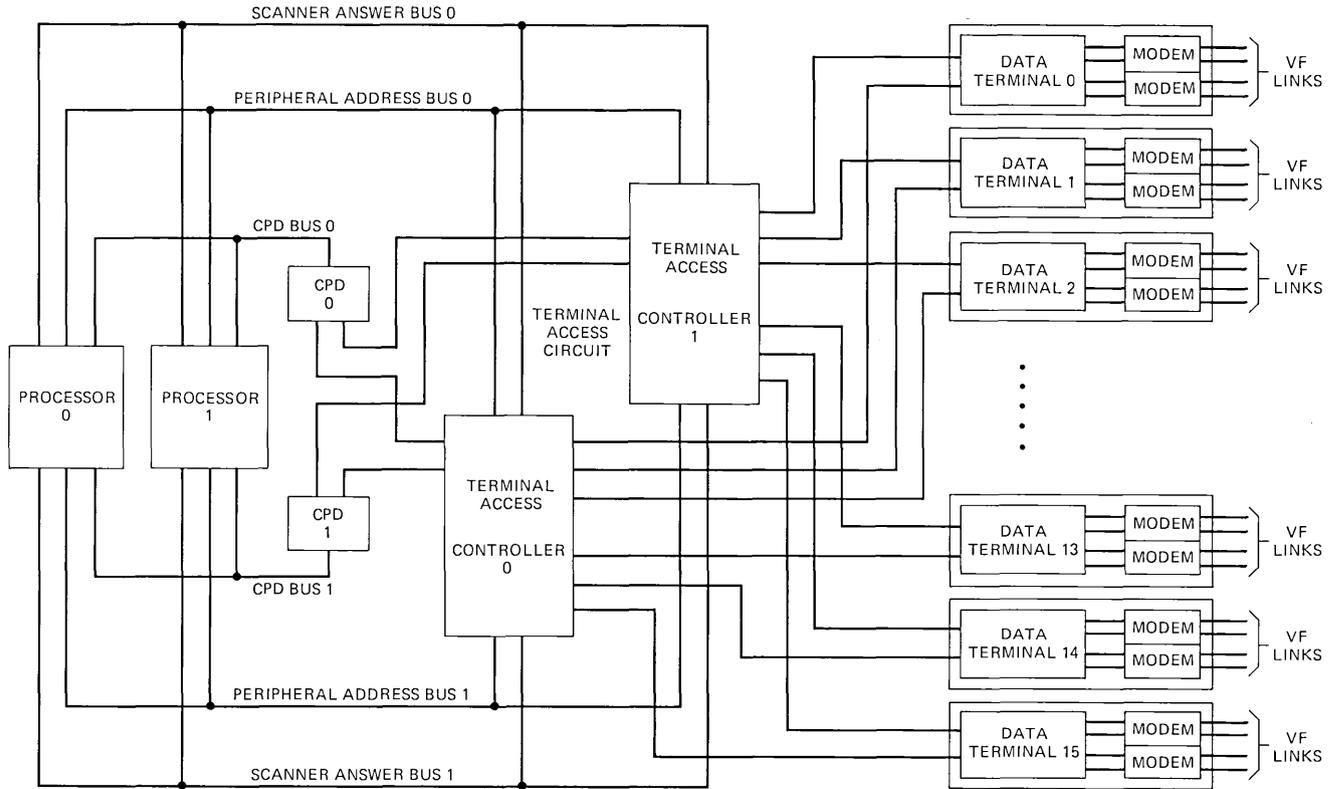
Fig. 18—No. 1 ESS terminal group block diagram.
