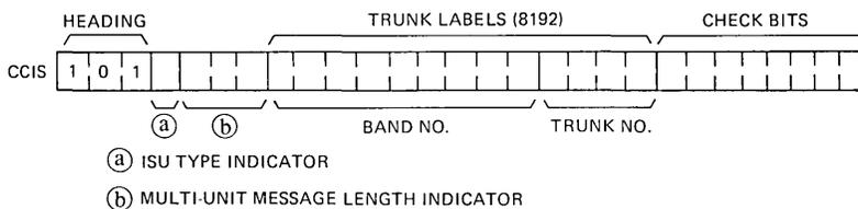
Fig. 8—Initial Signal Unit (ISU) format.
