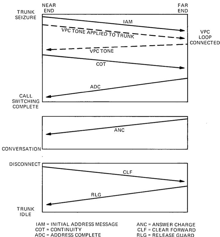
Fig. 4—Typical signal unit exchange.
