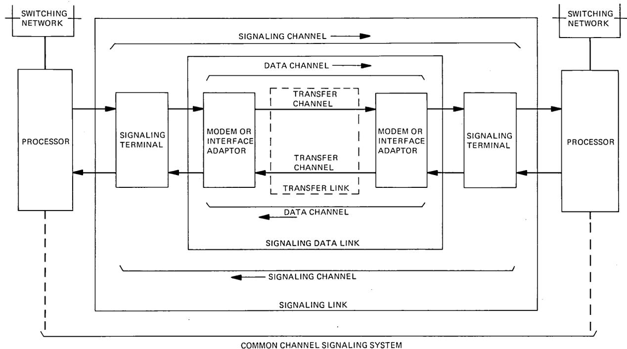
Fig. 4—Basic block diagram of the Common Channel Interoffice Signaling System.
