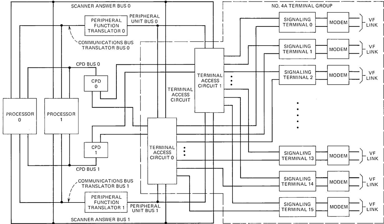
Fig. 7—No. 4A crossbar terminal group block diagram.
