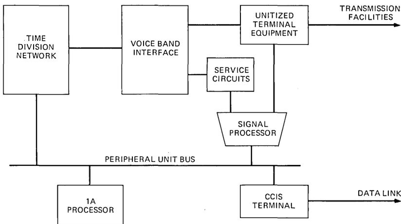
Fig. 1—No. 4 ESS system architecture.
