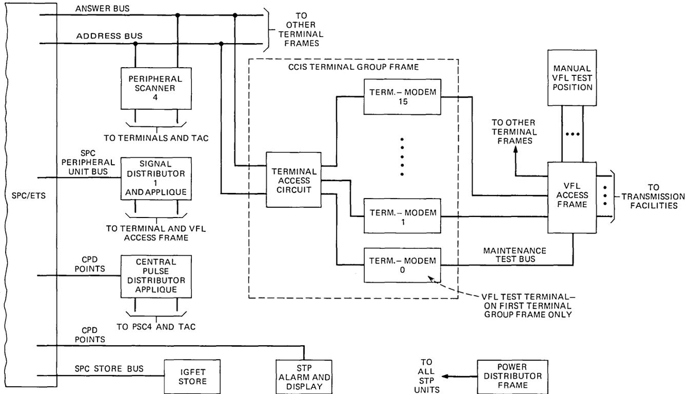
Fig. 3—ETS/STP system block diagram.
