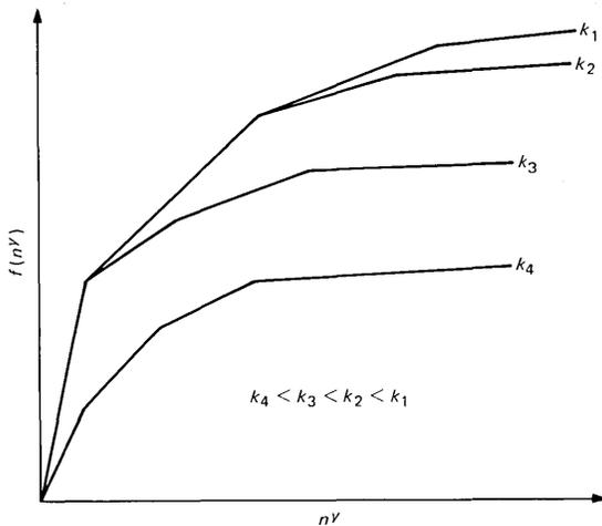
Fig. 1.—Linear programming optimal value  $[f(n^y)]$  as a function of the number of CCIS office conversions  $n^y$  and trunk group conversions  $k$ .
