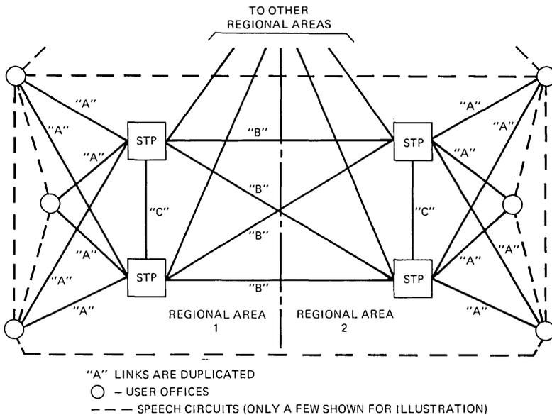
Fig. 3—User offices connected to STP quad.
