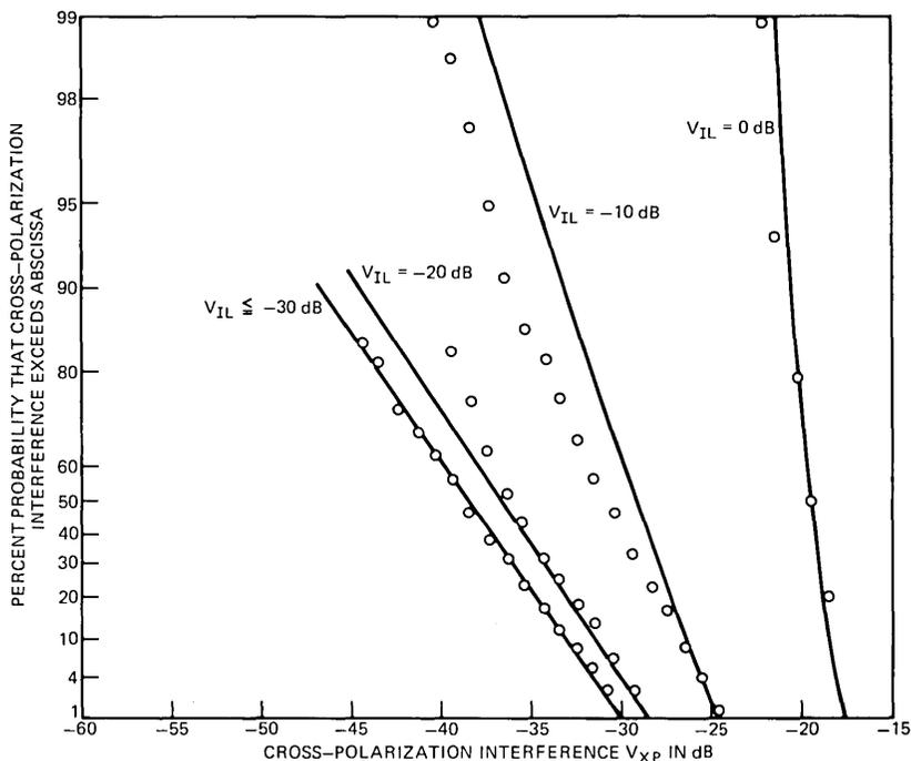
Fig. 12—Rice-Nakagami distribution (with Rayleigh probability coordinates) of cross-polarization interference,  $V_{xp}$ , conditioned to a given in-line signal level,  $V_{IL}$ , and measured on the 11-GHz 26.4-mile path (Atlanta-Palmetto). The circles are measured 6.5-month data (August 15, 1974 to February 28, 1975).
