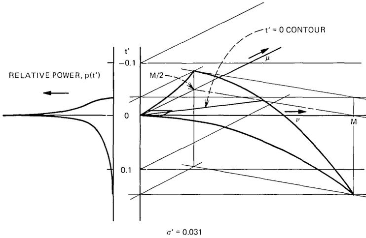
Fig. 1—Normalized time of arrival vs mode number (right) and mode count vs time of arrival (left) for  $n = n_0[1 - 2\Delta R^2 + (\frac{5}{7})(2\Delta)^2 R^4]^{1/2}$ ; i.e.,  $\delta = \frac{5}{7}\Delta$ .
