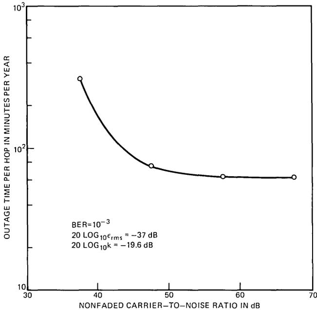
Fig. 22—Effect of reducing thermal noise level on the multipath two-way outage probability of 11-GHz dual-polarization QCPK radio—with space diversity, 50-foot antenna spacing, and 26-mile path length.
