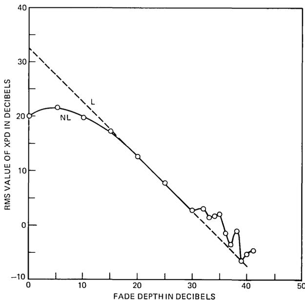
Fig. 1—RMS value of cross-polarized interference voltage as a function of fade depth. (Atlanta to Palmetto, Georgia, June 1974, 11 GHz.)
