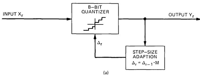
Fig. 5—Step-size adaption algorithm and quantizer characteristics of the APCM coders.
