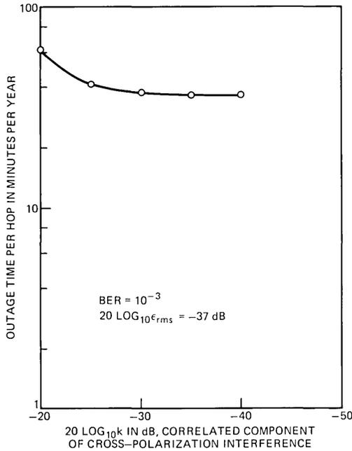
Fig. 21—Dependence of multipath two-way outage probability of 11-GHz dual-polarization QCPK radio on the correlated component,  $k_{VIL}$ , of cross-polarization interference—with space diversity, 50-foot antenna spacing, and 26.4-mile path.
