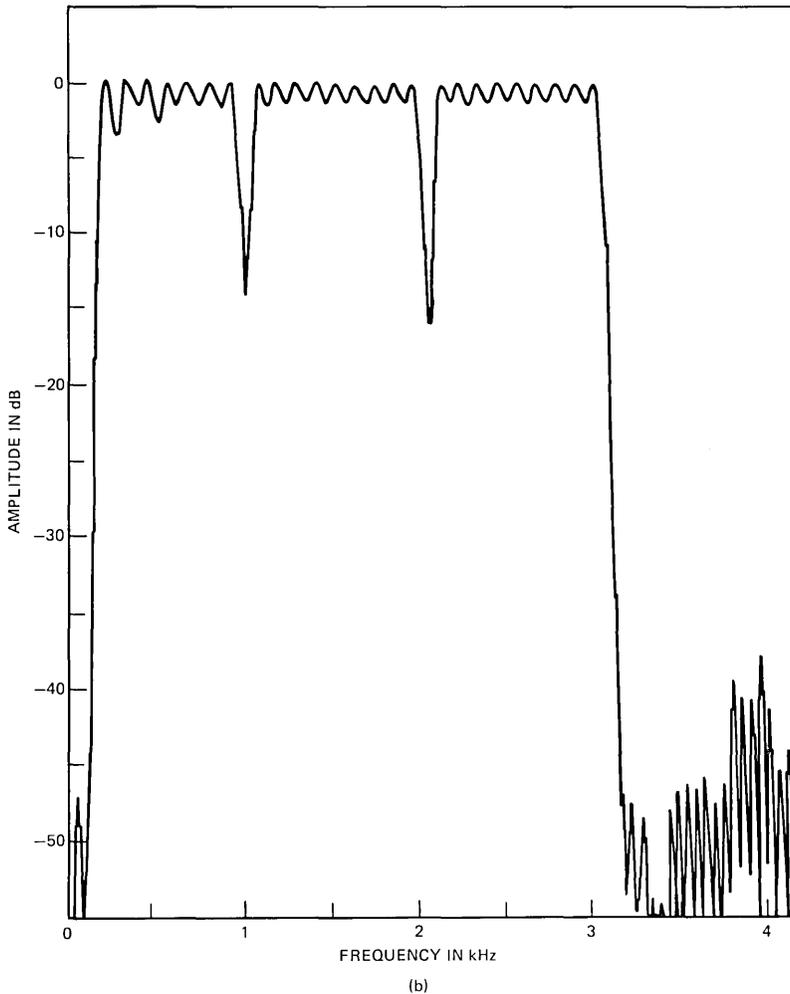
Fig. 8(b)—Measured frequency response for 16-kb/s coder.
