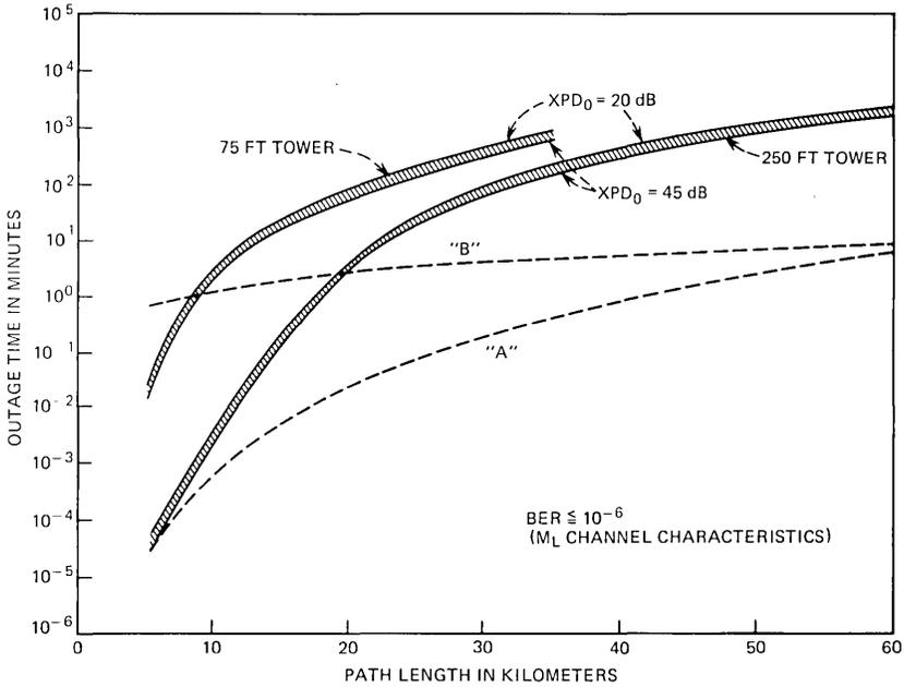
Fig. 11—Outage-time statistics for two antenna tower heights under terrain-scattering hypothesis.
