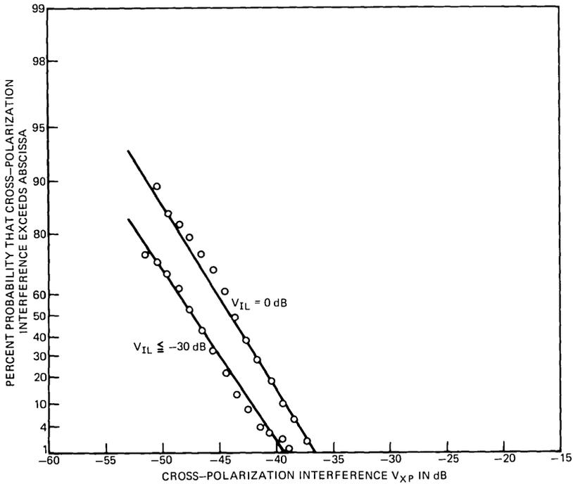
Fig. 13—Rice-Nakagami distribution (with Rayleigh probability coordinates) of cross-polarization interference,  $V_{XP}$ , conditioned to a given in-line signal level,  $V_{IL}$ , measured on the 11-GHz 15.9-mile path (Villa Rica-Palmetto). The circles are measured 6.5-month data (August 15, 1974 to February 28, 1975).
