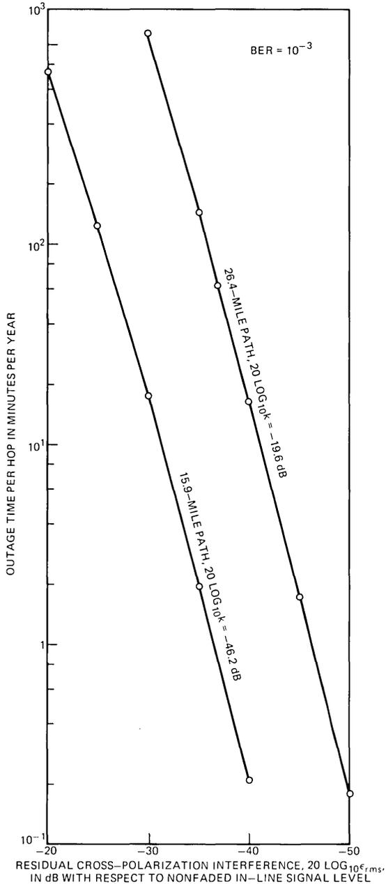
Fig. 20—Sensitivity of multipath two-way outage probability of 11-GHz dual-polarization QCPK radio on the rms value,  $\epsilon_{\text{rms}}$ , of the residual component of cross-polarization interference—with space diversity and 50-foot antenna spacing.
