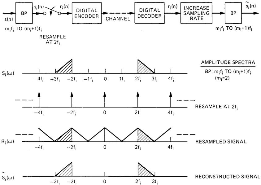
Fig. 2—Integer-band sampling technique and a frequency-domain interpretation.
