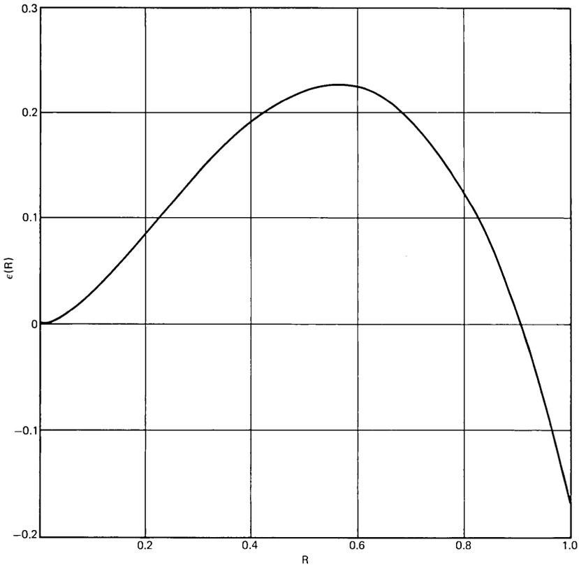
Fig. 6—Index perturbation from inverse parabola for minimum rms pulse width [see eqs. (12), (13)].
