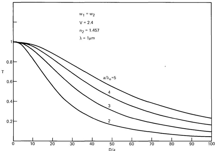
Fig. 8—Power transmission coefficient as a function of normalized longitudinal fiber displacement for identical step-index fibers. The curve parameter is the ratio  $a/\lambda$  of the core radius to free space wavelength.
