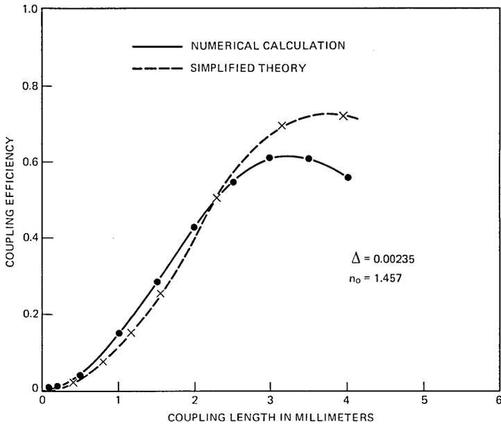
Fig. 7—Coupling efficiency vs coupling length; points indicate numerical results.
