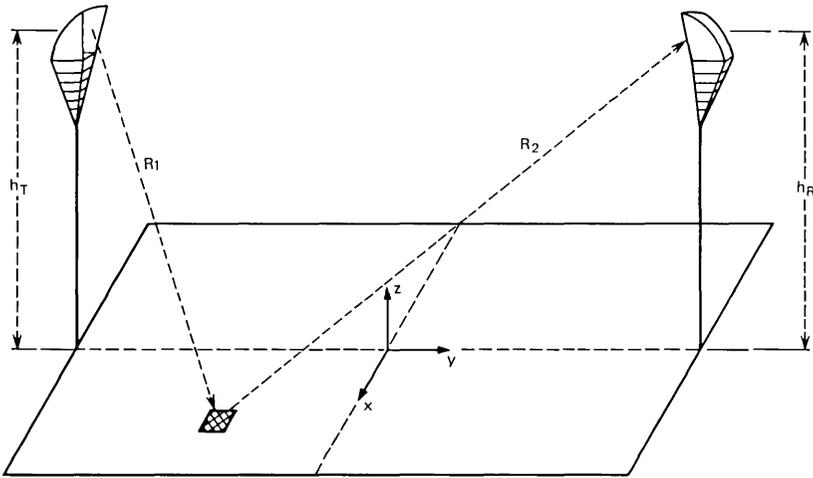
Fig. 15—Idealized radio-hop geometry used in terrain-scattering computation.
