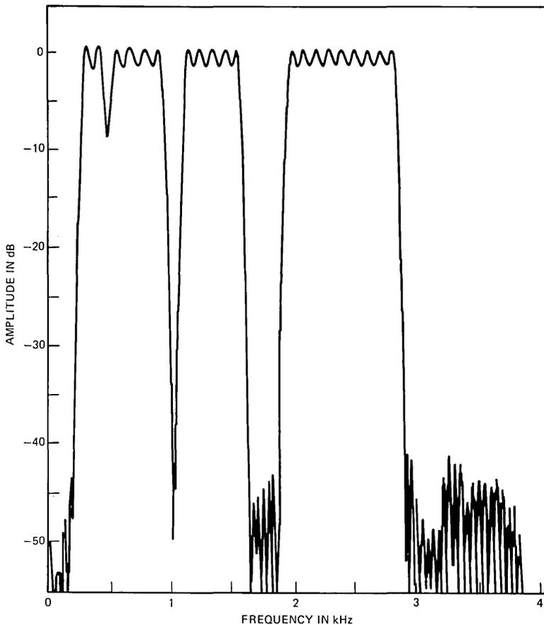
Fig. 8(a)—Measured frequency responses for 7.2- and 9.6-kb/s coders.
