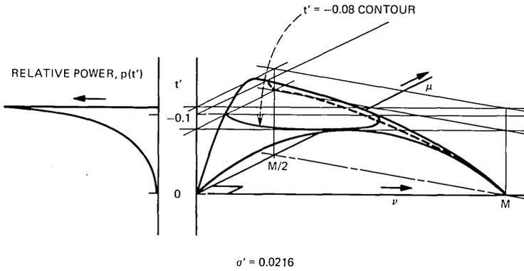
Fig. 5—Normalized time of arrival vs mode number (right), and mode count vs time of arrival (left), for  $n = n_0[1 - 2\Delta R^{2(1-2\delta/3)} + (1/3)(2\Delta)^2 R^4]^{1/2}$ ; i.e.,  $\rho = 2/3$ ,  $\delta = 1/3$ .
