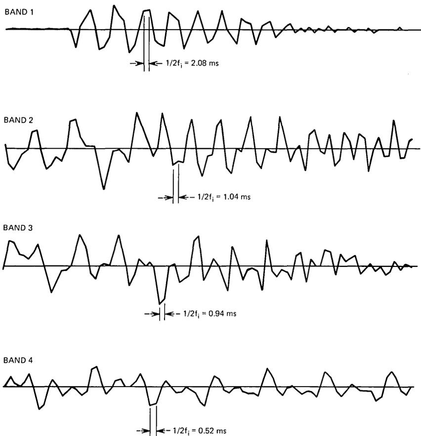
Fig. 4—Typical waveforms of uncoded sub-band signals for bands 1 to 4. Eighty samples are plotted on each line.
