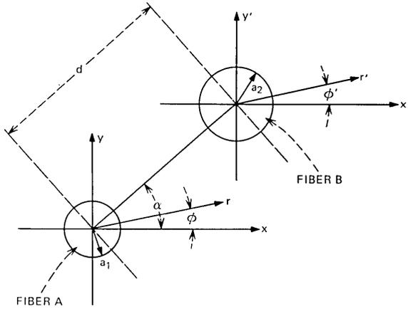
Fig. 1—Geometry used to derive the coupling coefficients.
