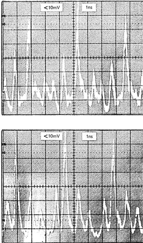
Fig. 3—Fiber output as a function of time and launching conditions.
