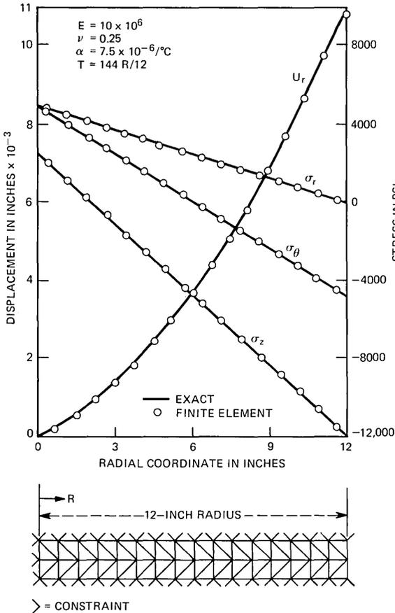
Fig. 5—Thermal stresses plane strain problem.
