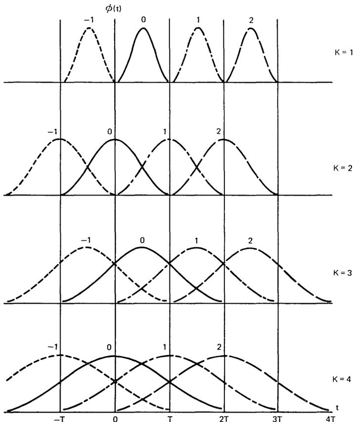
Fig. 1—Phase modulation for different signal pulse durations. Index  $k$  [eq. (42)] is shown near peak of each pulse. Also, for simplicity, same signal pulse is shown for each  $k$ .  $T$  = time slot duration or signaling period.  $KT$  = maximum signal pulse duration. Note different pulse center location for odd and even  $K$ .
