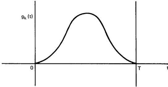
Fig. 5—Raised-cosine signaling with pulse duration  $T$ .  $K = 1$ .
