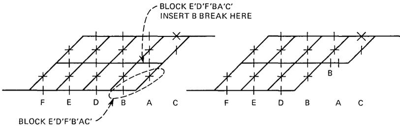
Fig. 20—Construction of circuit for  $S_2^6(55)-16-32$ .
