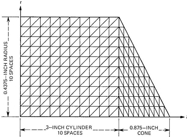
Fig. 8—Network of triangular annuli—lithium tantalate crystal—solid-of-revolution model.
