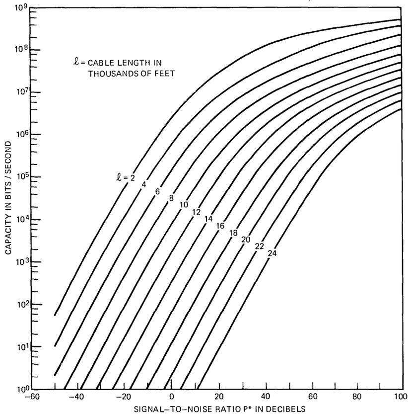
Fig. 2—Channel capacity for experimental cable. Capacity  $C$  in bits per second is plotted as a function of signal-to-noise ratio  $P^*$  for various values of cable length  $l$ . The  $C$  axis is logarithmic.
