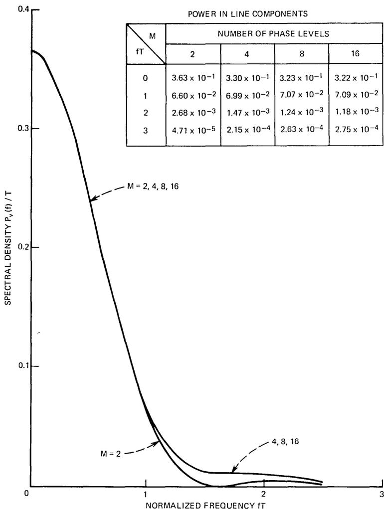
Fig. 6—Spectral density of binary, quaternary, octonary, and 16-ary PSK systems with raised-cosine signaling and pulse duration  $T$ .  $K = 1$ . Although the values of the spectral density for  $M = 2, 4, 8,$  and  $16$  are shown to be the same over certain segments of the range of  $f$ , they are usually different from each other, but this difference is not large enough to be shown on the linear scale in Fig. 6.
