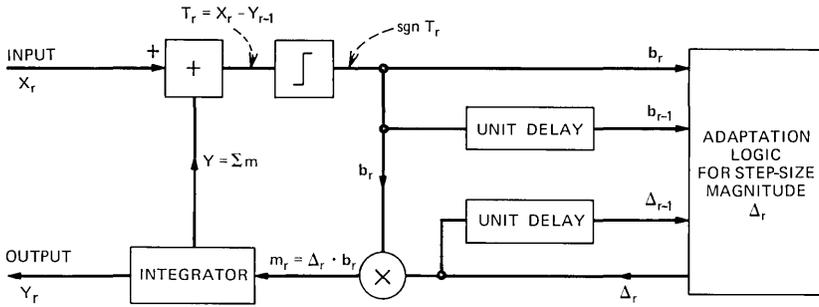
Fig. 2—Schematic diagram of an adaptive delta modulator.
