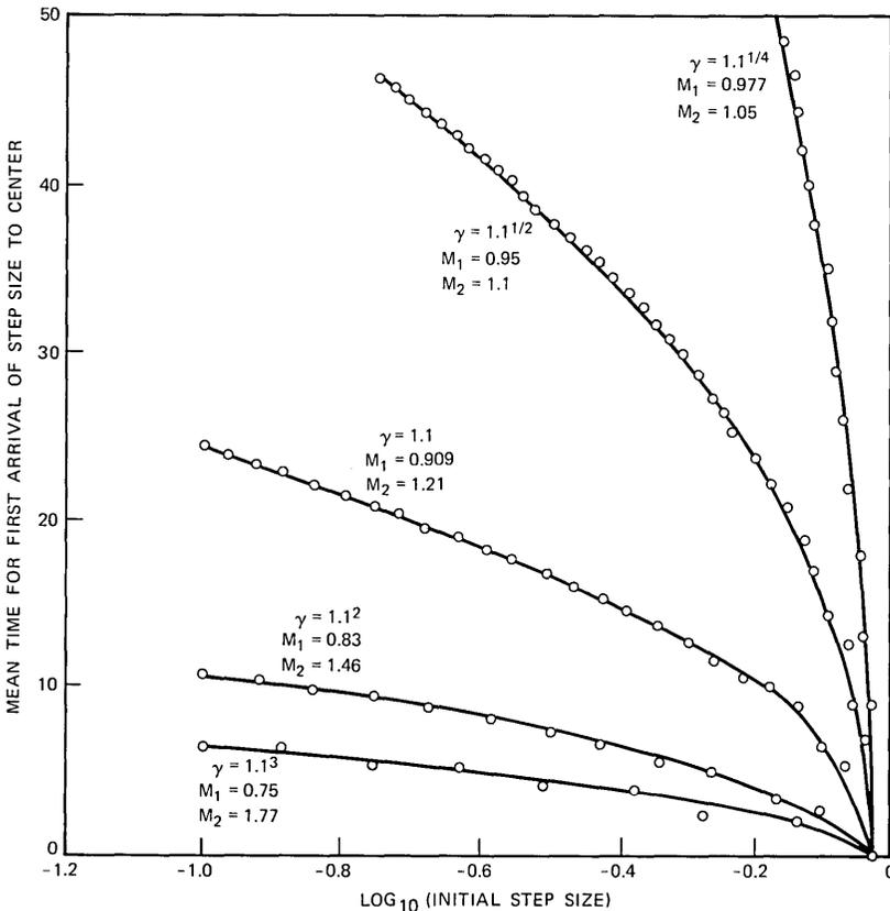
Fig. 6—Transient response of the adaptive quantizer.
