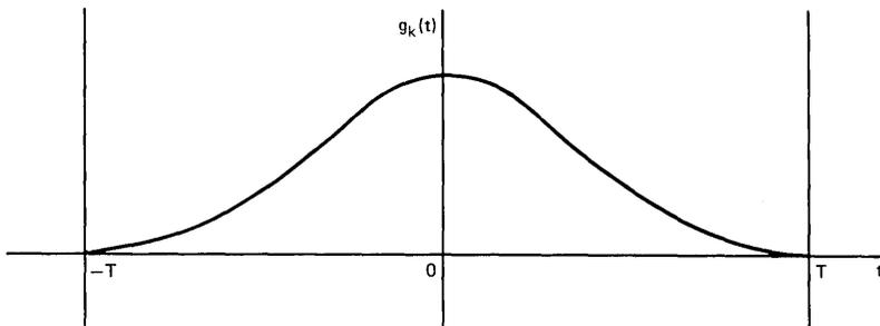
Fig. 7—Raised-cosine signaling with pulse duration  $2T$ .  $K = 2$ .
