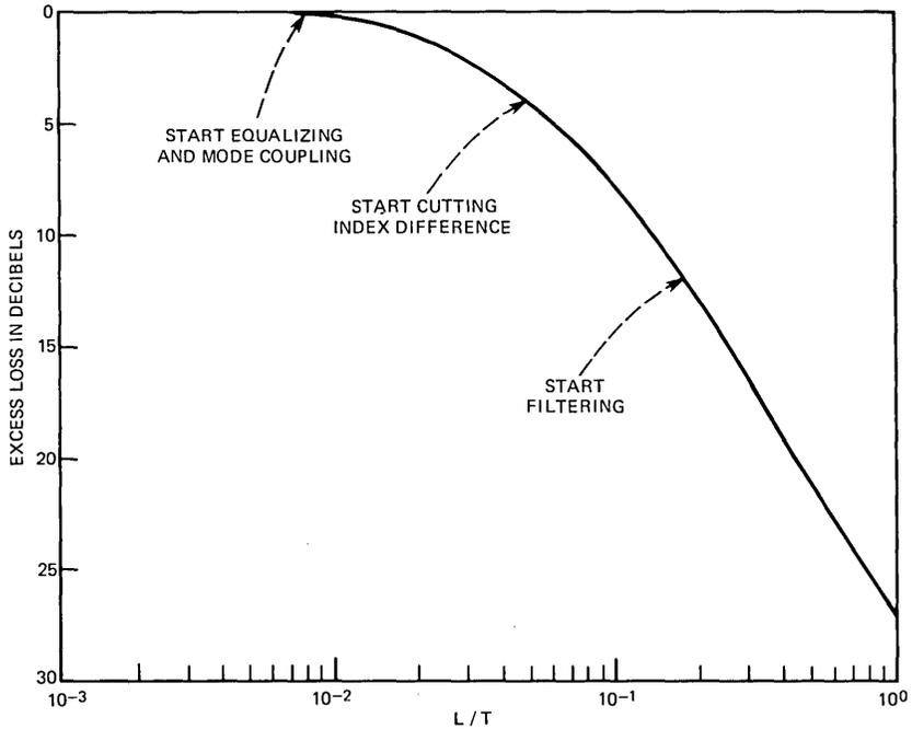
Fig. 4—Excess loss vs  $L/T$  for conventional fiber with coupling ( $\alpha_0 = 0.1$ ).
