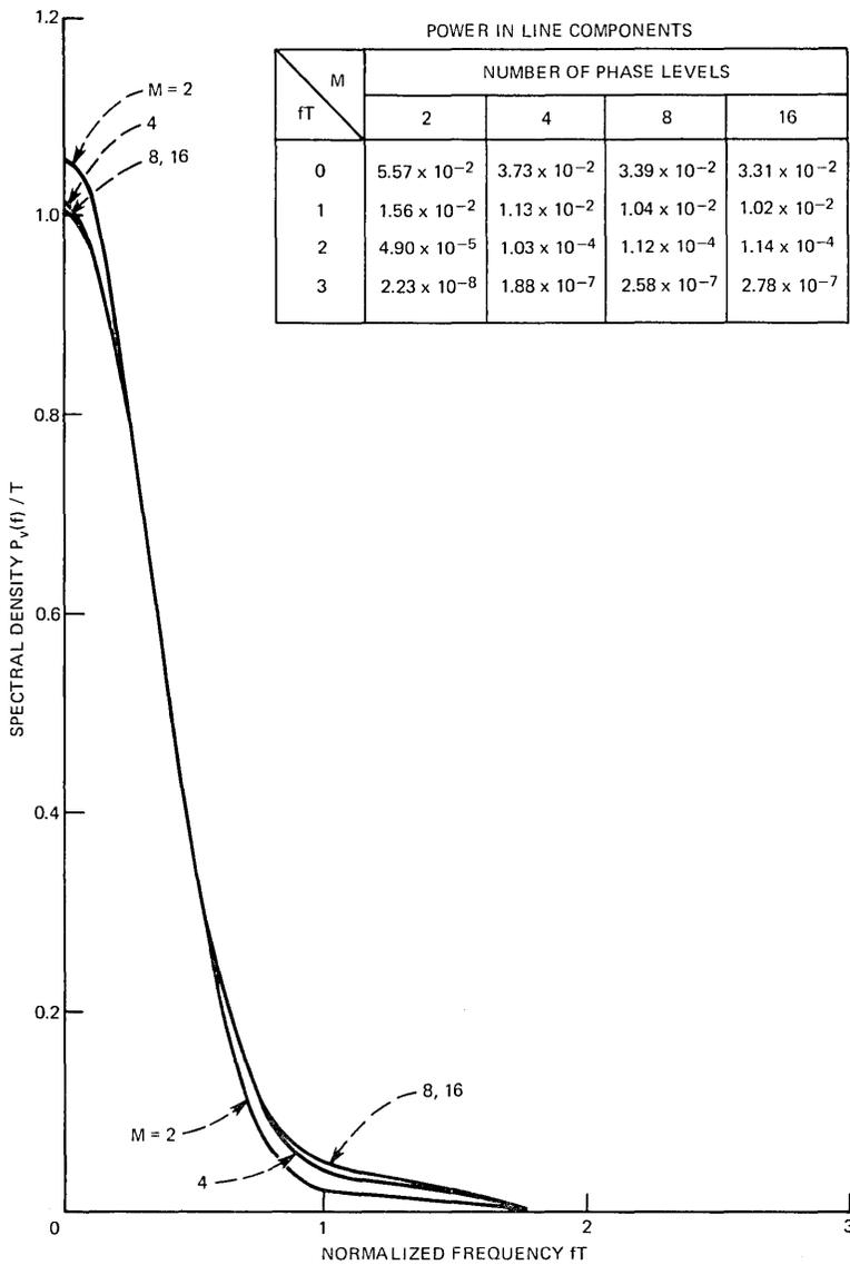
Fig. 8—Spectral density of binary, quaternary, octonary, and 16-ary PSK systems with raised-cosine signaling and pulse duration  $2T$ .  $K = 2$ . Although the values of the spectral density for  $M = 2, 4, 8,$  and  $16$  are shown to be the same over certain segments of the range of  $f$ , they are usually different from each other, but this difference is not large enough to be shown on the linear scale in Fig. 8.
