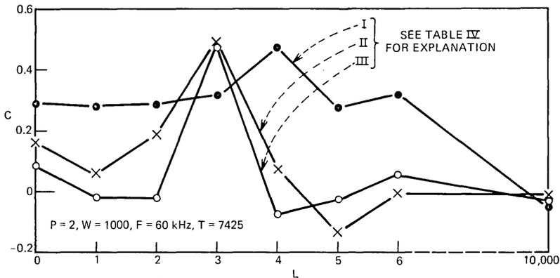
Fig. 6—Dependence of correlation  $C$  on time shift  $L$  —example of unsynchronized delta modulators.
