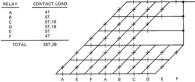
Fig. 1—Simplified circuit for Born and Scidmore problem by Born and Scidmore technique.
