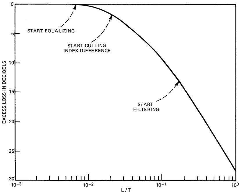
Fig. 2—Excess loss vs  $L/T$  for conventional fiber.
