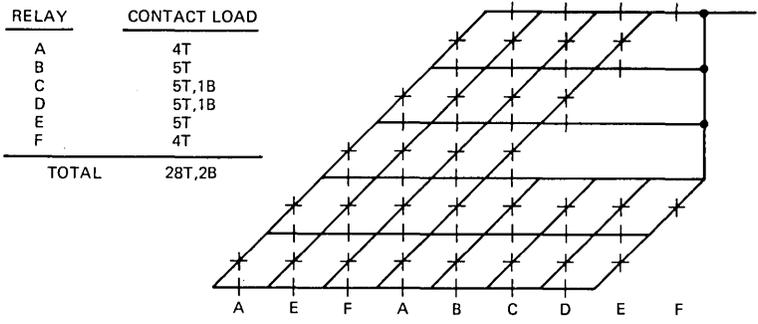
Fig. 13—Simplified symmetric for  $S_{2,3,4,5}^2$  (A, B, C, D, D, E, E, F, F).
