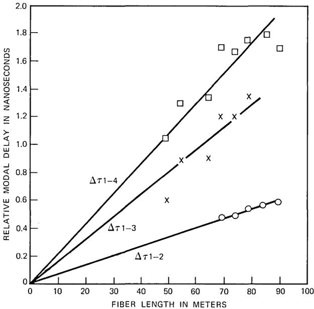
Fig. 4—Relative modal delay as a function of fiber length.
