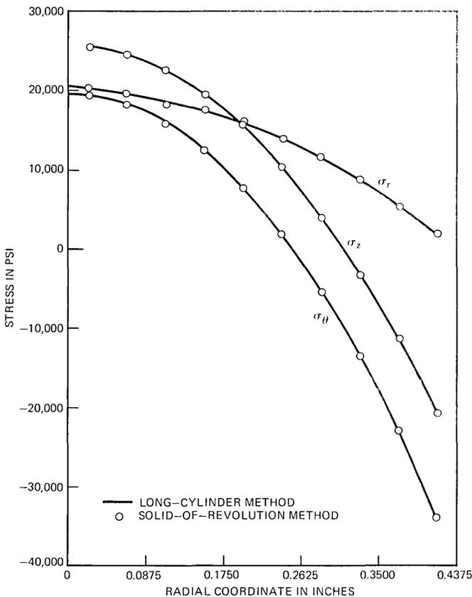
Fig. 11—Thermal stress comparison  $z$ -growth  $\text{LiTaO}_3$  crystal.
