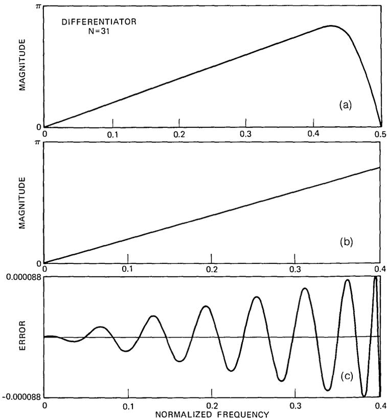
Fig. 4—The frequency response and error curve of an  $N = 31$ ,  $F_p = 0.4$  wideband differentiator.
