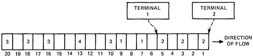
Fig. 5—Flow of data slots, alternate slot seizure.
