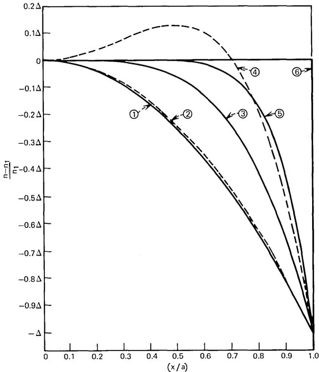
Fig. 1—Normalized index of refraction versus transverse coordinate ( $x/a$ ) for the following parameters in eqs. (1) and (25): curve ①,  $u = 2, \delta = 0$ ; curve ②,  $u = 2, r = 4, \delta = 0.05$ ; curve ③,  $u = 4, \delta = 0$ ; curve ④,  $u = 4, r = 2, \delta = -1$ ; curve ⑤,  $u = 8, \delta = 0$ ; curve ⑥,  $u = \infty, \delta = 0$ .
