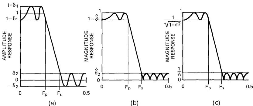
Fig. 1—Terminology used to describe low-pass filter characteristics.
