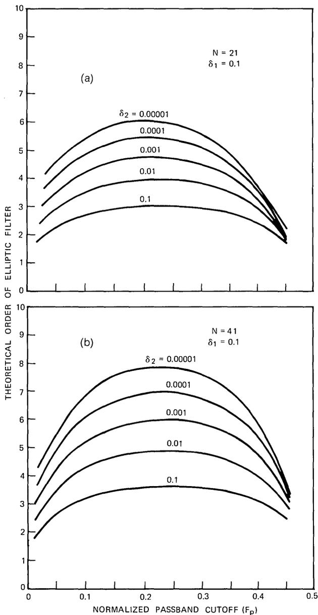
Fig. 7—Theoretical order of elliptic filters required to meet given specification on  $\delta_1$ ,  $\delta_2$ ,  $F_p$ , and  $F_s$  as a function of  $F_p$  for various values of  $\delta_2$ . Optimum FIR filters with  $N = 21$  meet the specifications for all filters of (a), whereas  $N = 41$  is required for all filters of (b).
