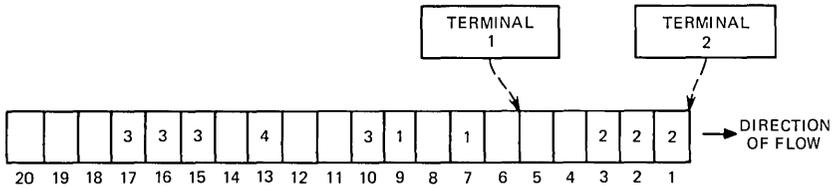
Fig. 4—Flow of data slots, adjacent slot seizure.
