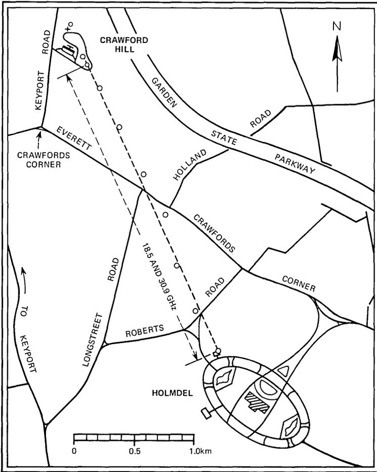
Fig. 1—The 2.6-km propagation path is indicated by the dashed line.
