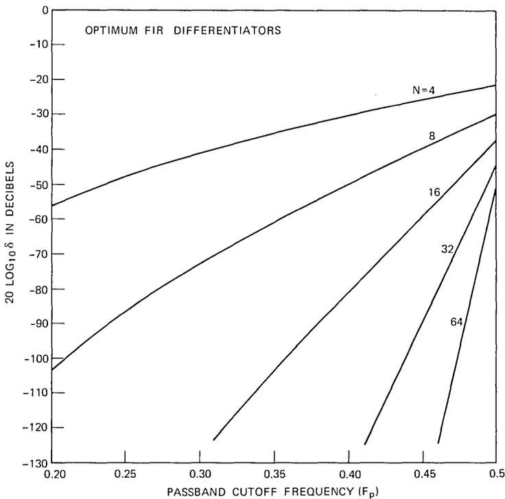
Fig. 7—The curves of  $20 \log_{10} \delta$  versus  $F_p$  for  $N = 4, 8, 16, 32,$  and  $64$ .
