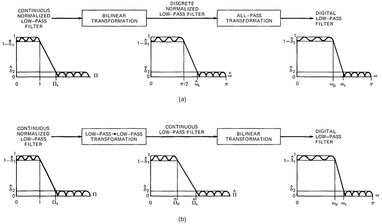
Fig. 2—Two techniques for transforming a continuous normalized low-pass filter to a digital low-pass filter.
