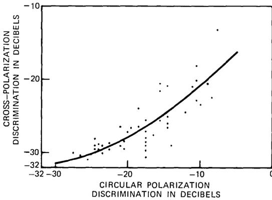
Fig. 3—Comparison of simultaneous measurements of linear polarization discrimination (XPD) and circular polarization discrimination (CPD).
