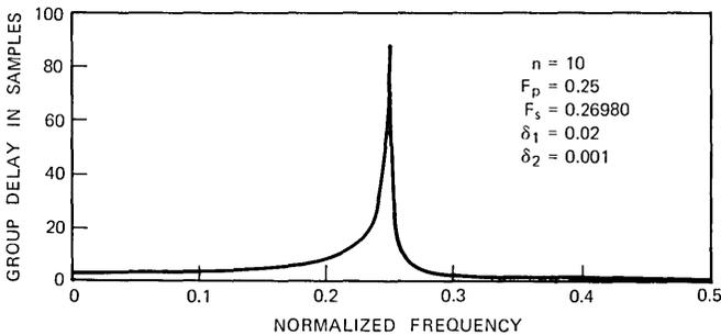
Fig. 9—The group delay of a 10th-order elliptic filter with  $F_p = 0.25$ .
