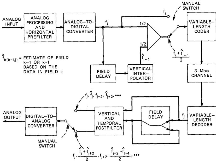
Fig. 2—Experimental system block diagram.
