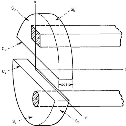
Fig. 1—Coupled dielectric waveguides.
