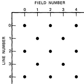
Fig. 1—Interlaced frame format.
