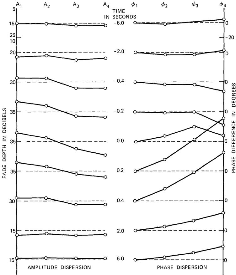
Fig. 7—Amplitude and phase dispersion during dispersive fade.
