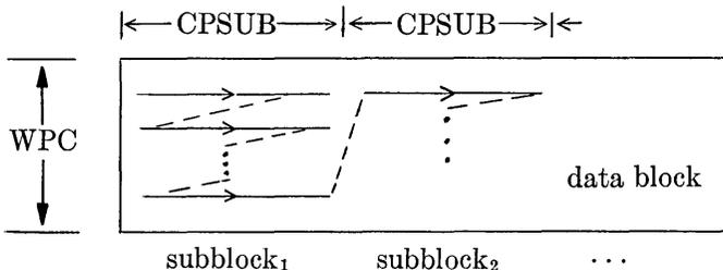
It should be noted that the subblock plays no further role except to establish an ordering. It does not correspond to a file, a record, or any other host-system concept. In fact, the mapping of block words onto stream words is performed without concern for record or file boundaries.
