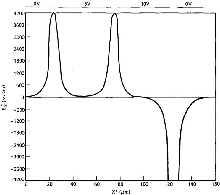
Fig. 6—The channel field  $-\partial\phi^*/\partial x^*$  plotted as a function of  $x^*$  for the CCD of Fig. 5 with  $\rho_g^*/e = 0.8 \times 10^{12} \text{ cm}^{-2}$  implanted in the gaps.
