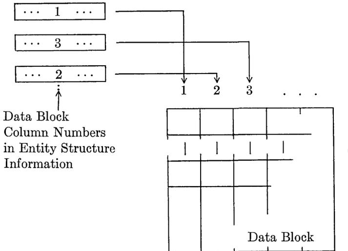
Column numbers, rather than absolute storage locations, are used to reference the data block, allowing separation of structure from data.
