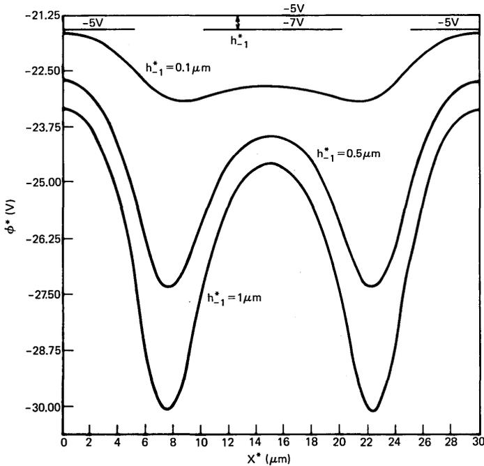
Fig. 7—The channel potential in a buried channel CCD with double-level metalization. The lower level electrodes are  $10\ \mu\text{m}$  wide with  $5\text{-}\mu\text{m}$  gaps and are at potentials of  $-5$  and  $-7$  V. The upper level is a single electrode at  $-5$  V;  $h_1^* = 0.1\ \mu\text{m}$ ;  $h_2^* - h_1^* = 5\ \mu\text{m}$ ;  $C_s^* = 4.6 \times 10^{15}\ \text{cm}^{-3}$ ; and the separation of the metalization levels is  $h_{-1}^* = 0.1, 0.5,$  and  $1.0\ \mu\text{m}$ .
