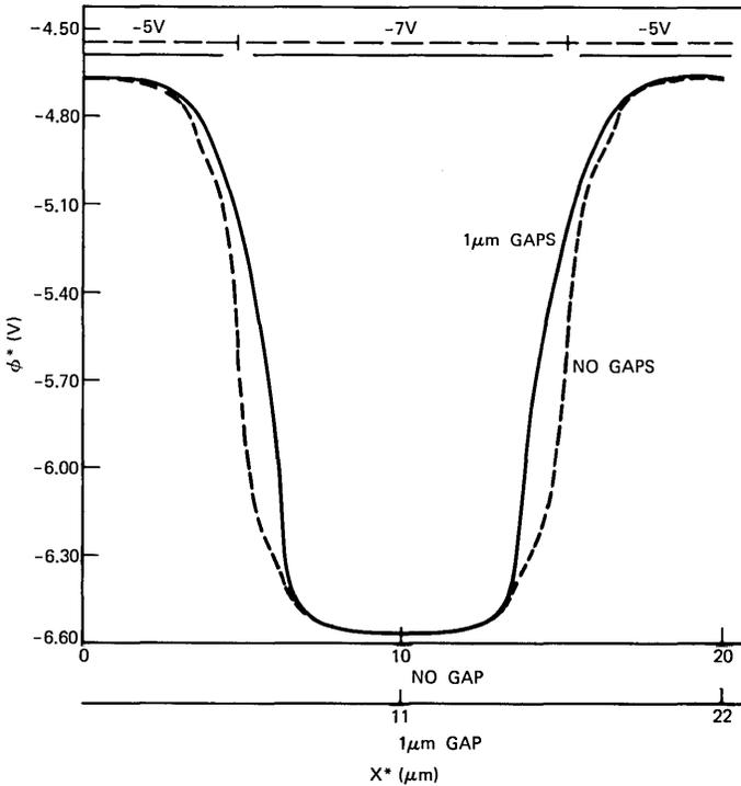
Fig. 11—The potential  $\phi^*(x^*, h_1^*)$  plotted as a function of  $x^*$  for a surface CCD with single-level metalization;  $h_1^* = 0.1 \mu\text{m}$ ; 10- $\mu\text{m}$ -wide electrodes held at  $-5$  and  $-7$  V; and with gaps between electrodes of 1 and 0  $\mu\text{m}$ .
