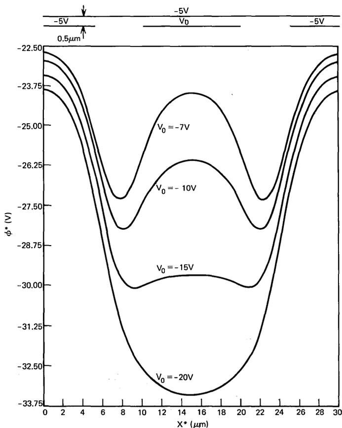
Fig. 8—The channel potential in the CCD of Fig. 7 with the separation of the metalization levels held fixed at  $h_{-1}^* = 0.5 \mu\text{m}$  and the potential of the center, lower-level electrode taking the values  $-7$ ,  $-10$ ,  $-15$ , and  $-20$  V.
