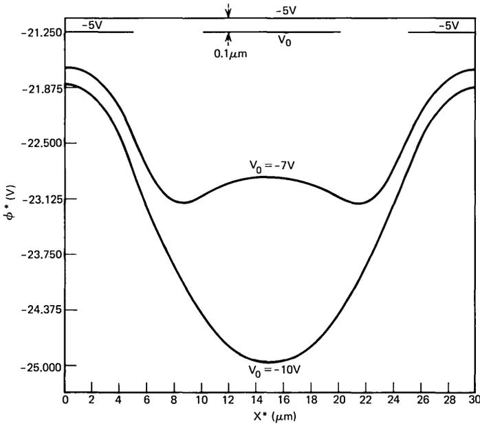
Fig. 9—The channel potential in the CCD of Fig. 7 with the separation of the metalization levels held fixed at  $h_{-1}^* = 0.1 \mu\text{m}$  and the potential of the center, lower-level electrode taking the values  $-7$  and  $-10$  V.
