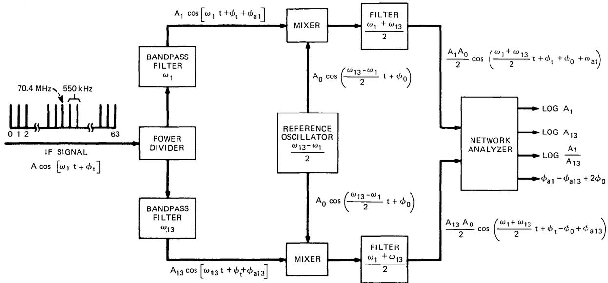
Fig. 1—Basic schematic of two-channel phase and amplitude comparator.
