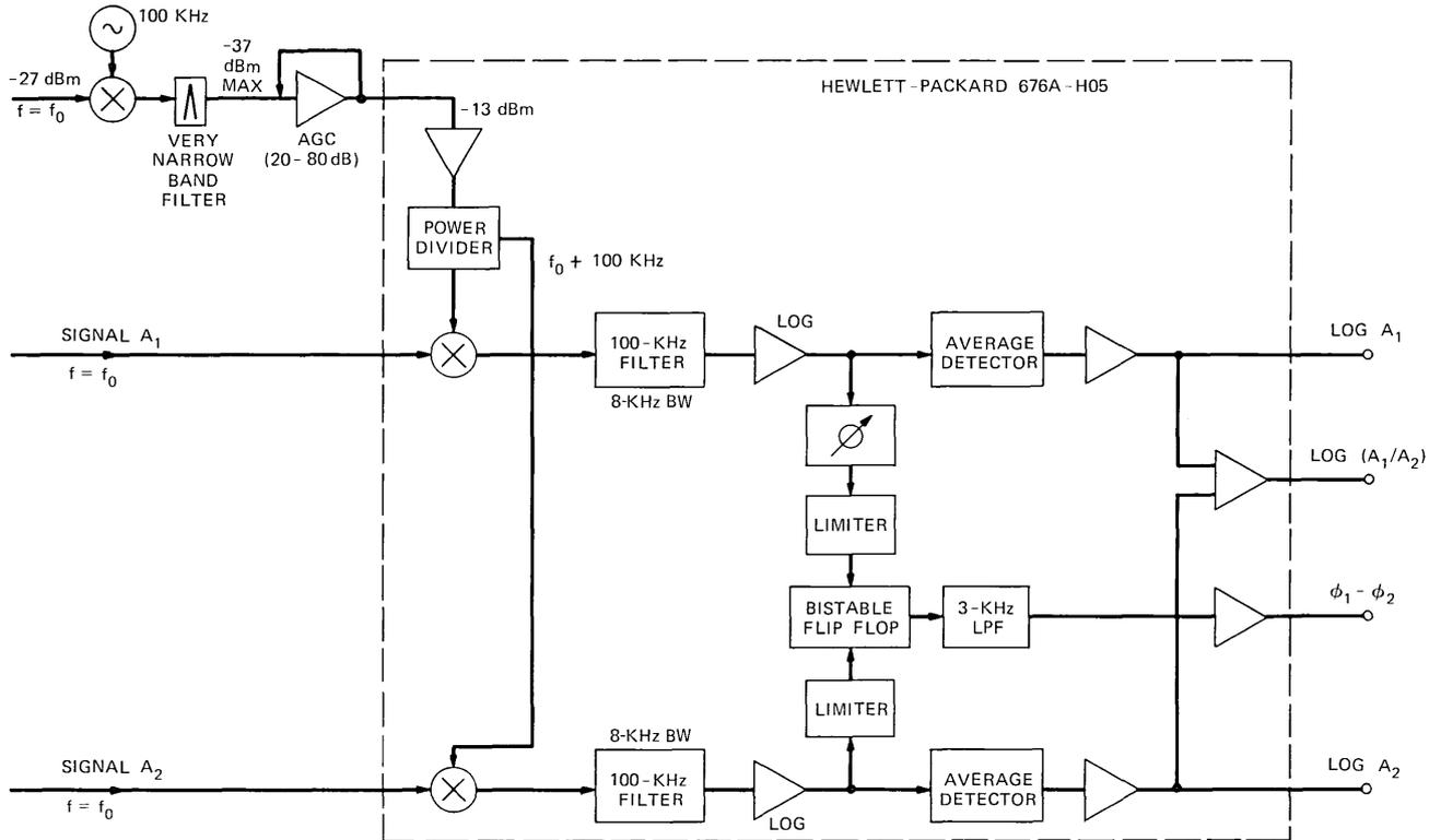
Fig. 3—Network analyzer.
