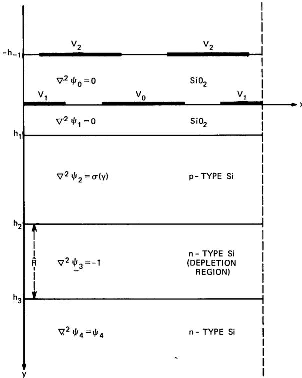
Fig. 3—A schematic diagram of the depletion layer approximation for one cell of a buried channel CCD with double-level metalization.
