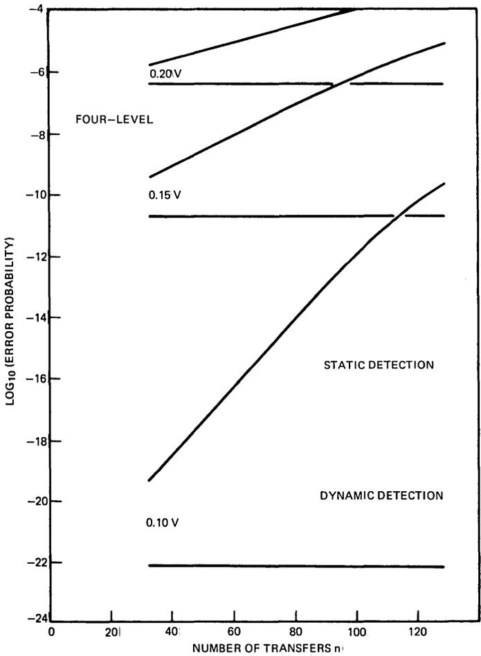
Fig. 3—Error probability as a function of the number of transfers  $n$  for static and dynamic detection of four-level coding for three values of root-mean-square detection voltage fluctuation (0.10, 0.15, and 0.20 V). For given  $n$ , the corresponding device is an  $n$ -bit device.
