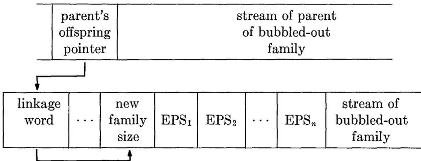
The linkage word is a single word connecting the new family description to the previously existing structure.
