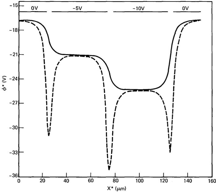
Fig. 5—The channel potential  $\phi^*$  plotted as a function of  $x^*$  for a three-phase buried channel CCD. The 45- $\mu\text{m}$ -wide electrodes are at 0, -5, and -10 V; the gaps are 5  $\mu\text{m}$  wide;  $h_1^* = 0.1 \mu\text{m}$ ;  $h_2^* - h_1^* = 5 \mu\text{m}$ ; and  $C_s^* = 4.6 \times 10^{15} \text{ cm}^{-3}$ . The dashed curve is for no surface charge implanted in the gaps; the solid curve is for  $\rho_s^*/e = 0.8 \times 10^{12} \text{ cm}^{-2}$  implanted in the gaps.
