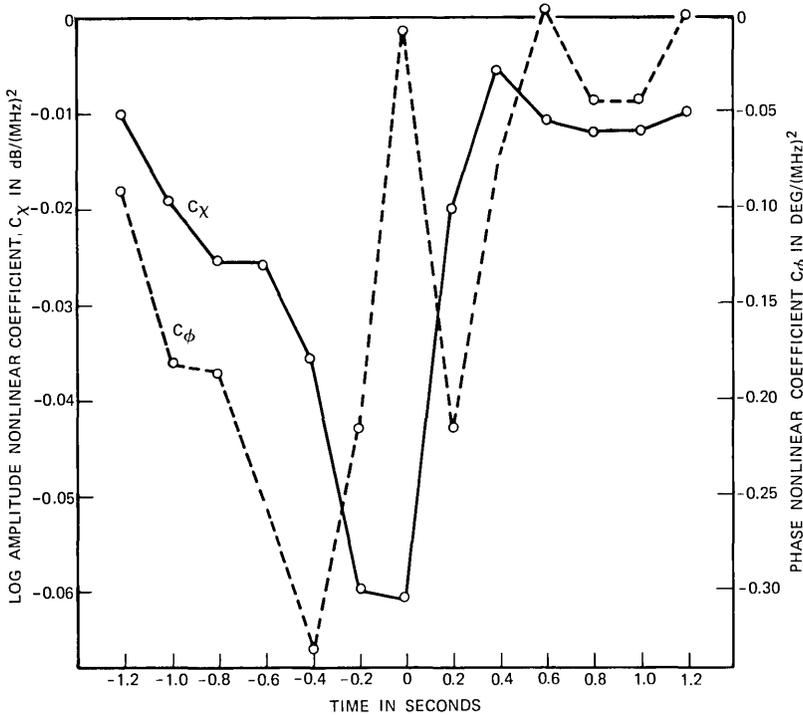
Fig. 8—Temporal behavior of log-amplitude and phase nonlinearities ( $c_x$ ,  $c_\phi$ ).
