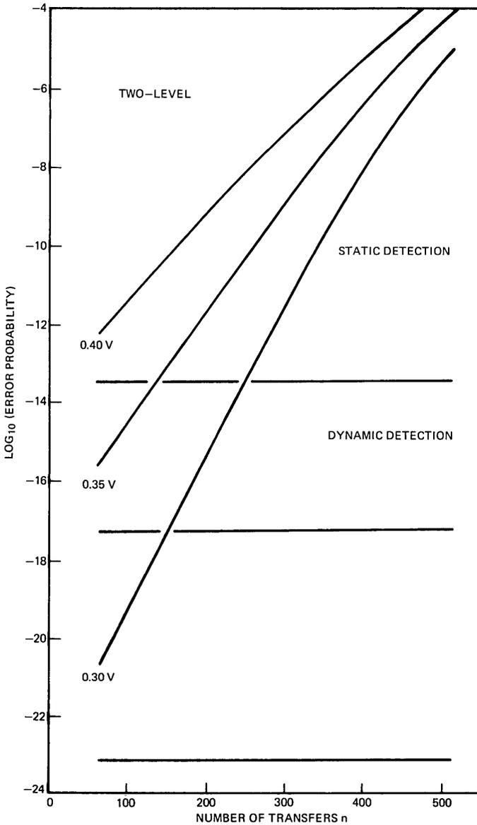
Fig. 2—Error probability as a function of the number of transfers  $n$  for static and dynamic detection of two-level coding for three values of root-mean-square detection voltage fluctuation (0.30, 0.35, and 0.40 V). For given  $n$ , the corresponding device is an  $n/2$ -bit device.
