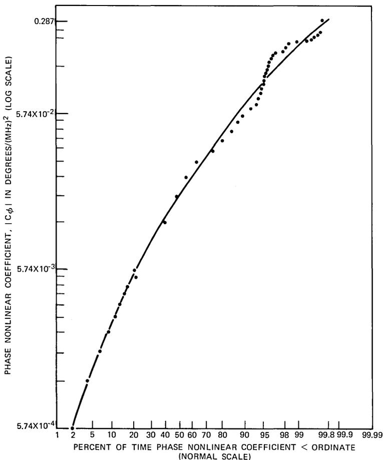
Fig. 10—Distribution curve for  $|c_\phi|$ : log-normal plot.
