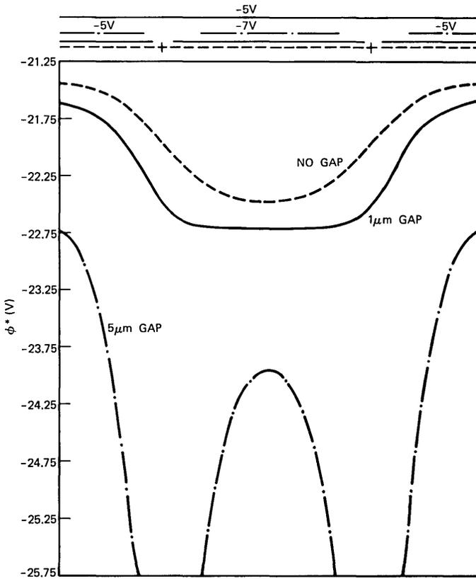
Fig. 10—The channel potential in the CCD of Fig. 7 with the separation of the metalization levels held fixed at  $h_{-1}^* = 0.5 \mu\text{m}$ , and the gap width taking the values 5, 1, and 0  $\mu\text{m}$ .
