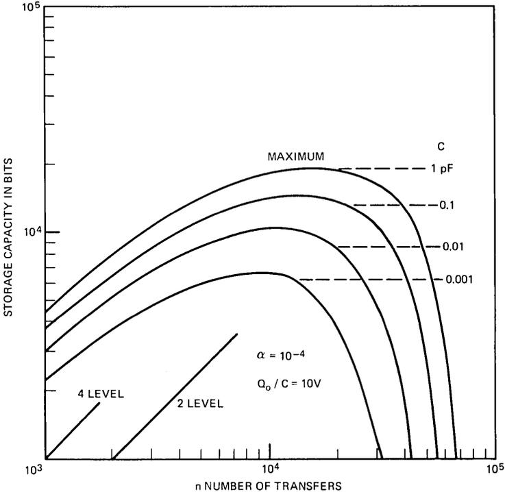
Fig. 9—Storage capacity  $C_s$  versus  $n$ , the number of charge transfers, for  $\alpha = 10^{-4}$ ,  $Q/C = 10$  volts,  $C = 1, 0.1, 0.01, 0.001$  pF. Shown for comparison is  $C_s$  for 2- and 4-level digital codes.
