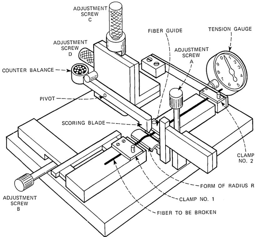
Fig. 3—A semi-schematic view of the fiber breaking machine.
