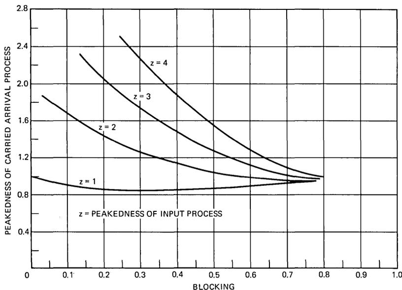
Fig. 10—Peakedness of CAP versus blocking (5 trunks).
