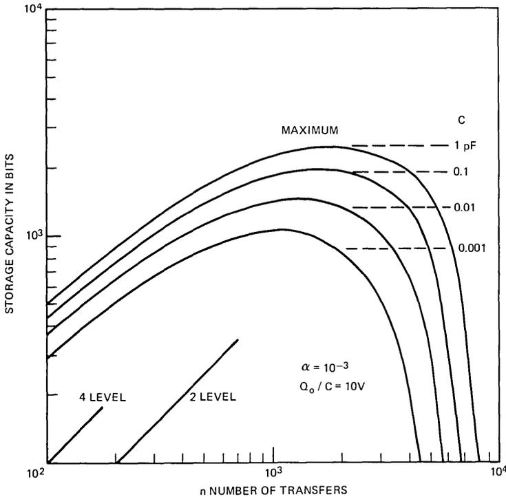
Fig. 8—Storage capacity  $C_s$  versus  $n$ , the number of charge transfers, for  $\alpha = 10^{-3}$ ,  $Q/C = 10$  volts,  $C = 1, 0.1, 0.01, 0.001$  pF. Shown for comparison is  $C_s$  for 2- and 4-level digital codes.
