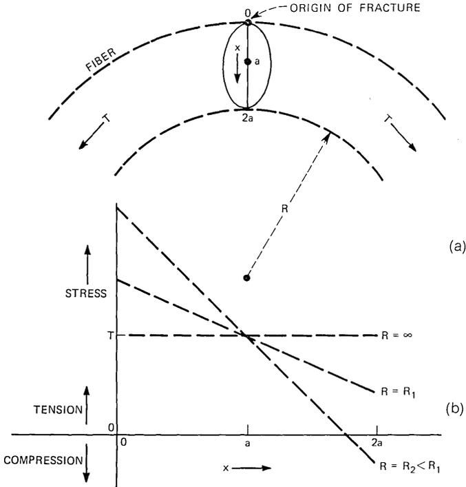
Fig. 2—(a) A glass fiber bent over a form of radius  $R$  and subjected to a tension  $T$ . (b) The stress as a function of position in the fiber for various bending radii  $R$ .
