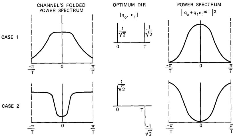
Fig. 4—Optimum desired impulse response of length two.
