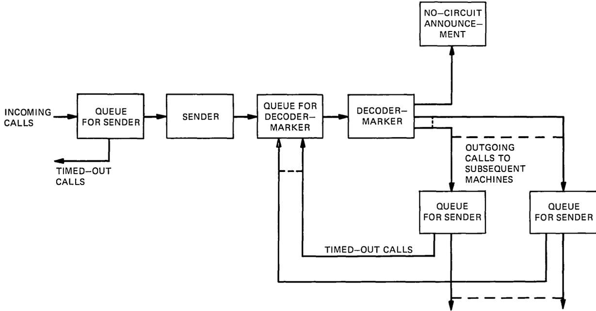
Fig. 2—Switching machine block diagram.
