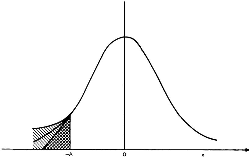
Fig. 10—Approximating the area under a portion of Gaussian curve by bounding the area between that of a right triangle (whose hypotenuse is tangent to the Gaussian at  $x = -A$ ) and by the area under an exponential (also tangent to the Gaussian at  $x = -A$ ).
