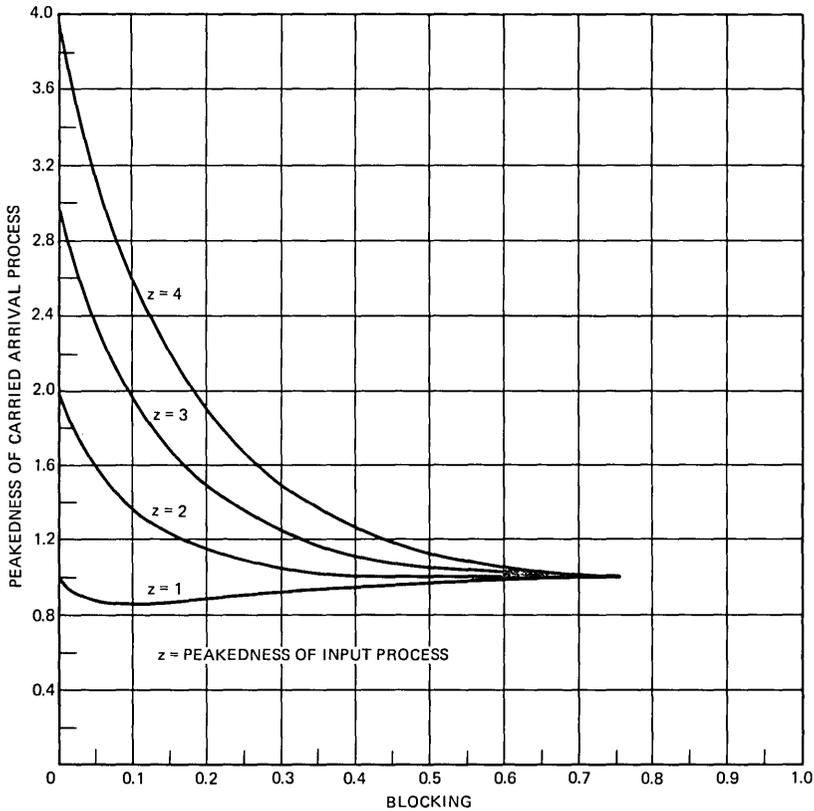
Fig. 13—Peakedness of CAP versus blocking (50 trunks).
