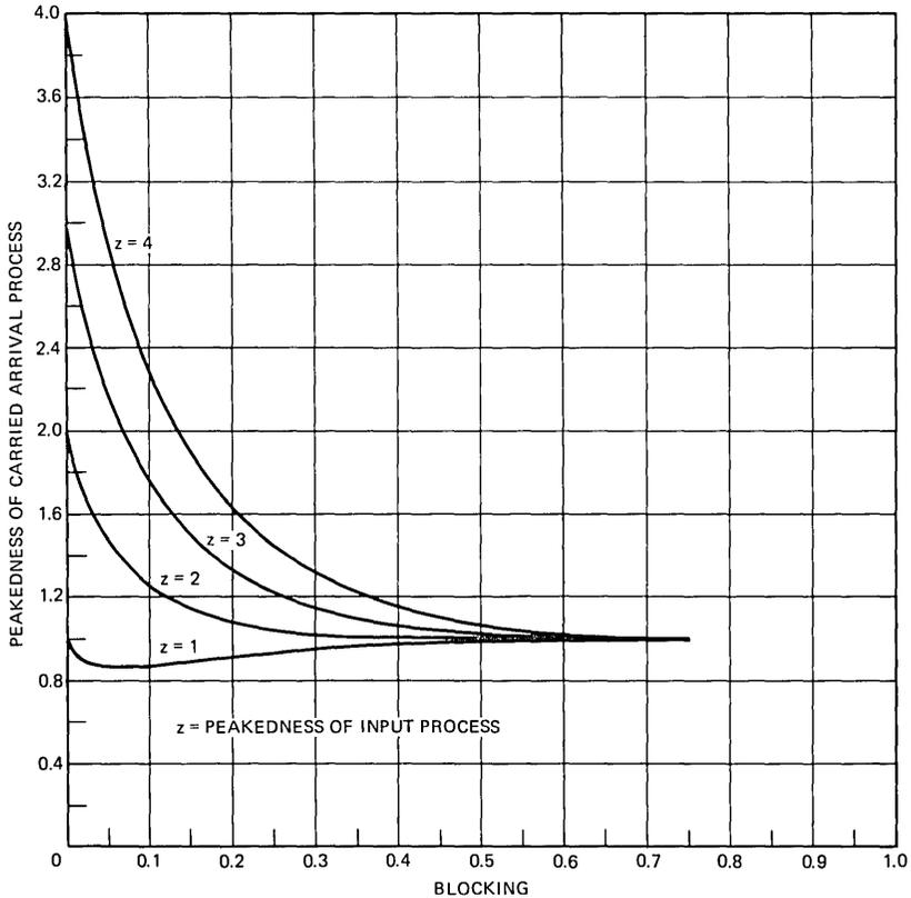
Fig. 14—Peakedness of CAP versus blocking (100 trunks).
