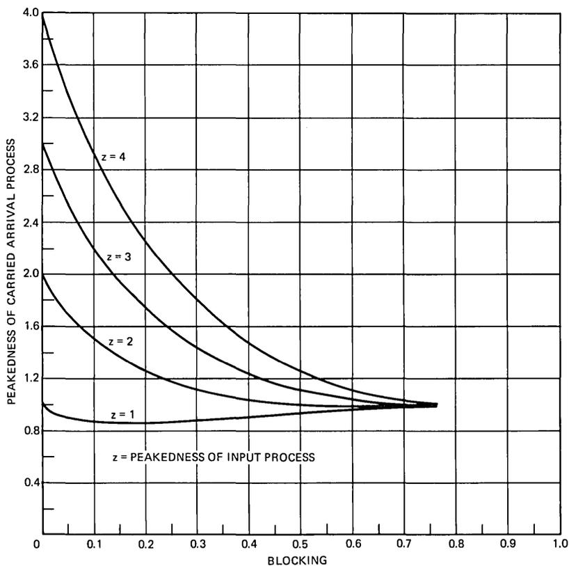
Fig. 12—Peakedness of CAP versus blocking (20 trunks).
