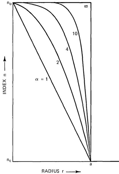
Fig. 5—A few of the index profiles defined by  $n = n_0[1 - 2\Delta(r/a)^\alpha]^{\frac{1}{2}}$  for small  $\Delta$ .
