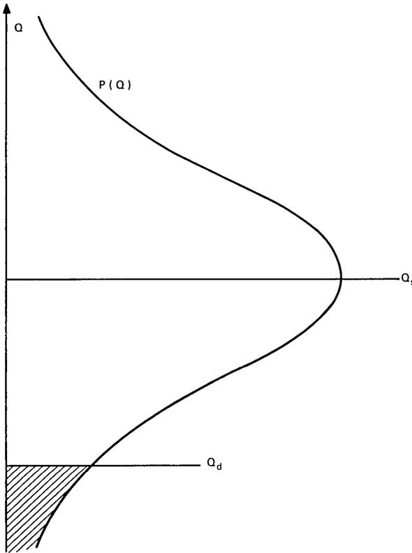
Fig 7.—A charge packet of size  $Q_s$  under noiseless conditions has a probability distribution of  $P(Q)$  in the presence of noise. The probability that  $Q < Q_d$  (that an error is made in detection) is the area “under”  $P(Q)$  for  $Q < Q_d$ .
