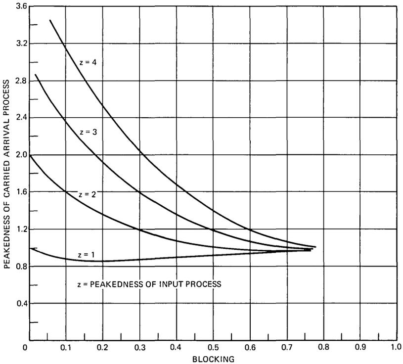
Fig. 11—Peakedness of CAP versus blocking (10 trunks).
