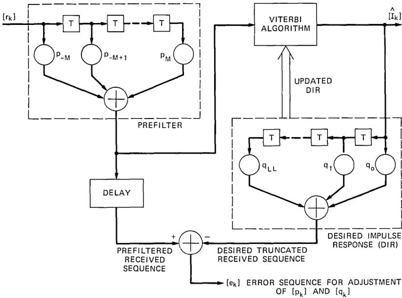
Fig. 3—Receiver structure.
