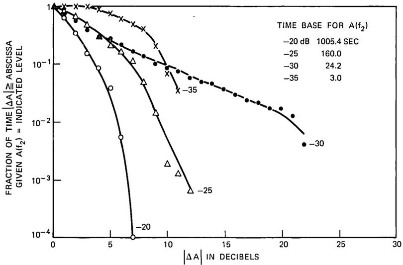
Fig. 17—Conditional linear distortion distributions for the 19.8-MHz, -30-dB threshold diversity channel.
