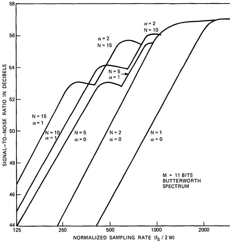
Fig. 5—Performance characteristics,  $M = 11$  bits, Butterworth spectrum.
