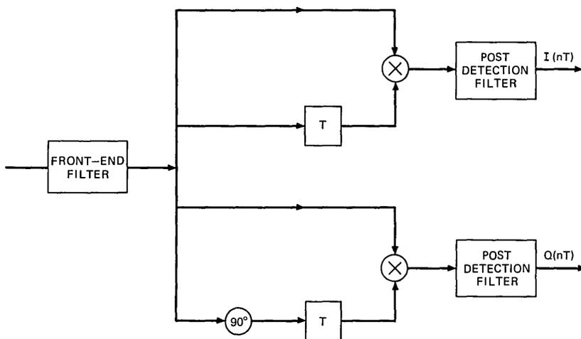
Fig. 1—Comparison (differential) detector.
