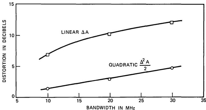
Fig. 16—Growth of linear and quadratic distortion with bandwidth for the non-diversity channel and the  $-30$ -dB threshold diversity channel for a fixed  $10^{-5}$  fraction of the time.
