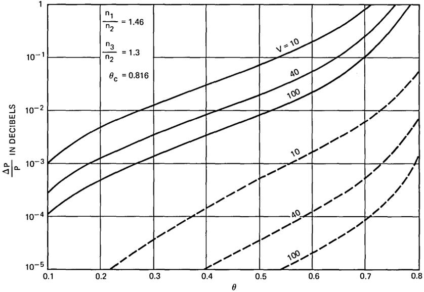
Fig. 3—Relative scattered power (solid lines) as a function of mode angle  $\theta$ . The waveguide core and the supports are in an air environment. The dotted lines represent the reflection loss of each mode.
