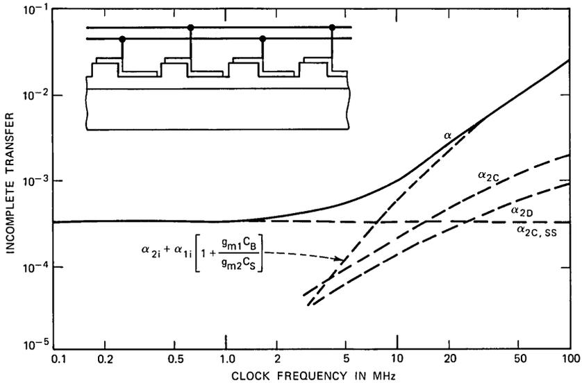
Fig. 10—Contributions to  $\alpha$  (incomplete transfer) for the stepped-oxide, two-phase CCD.
