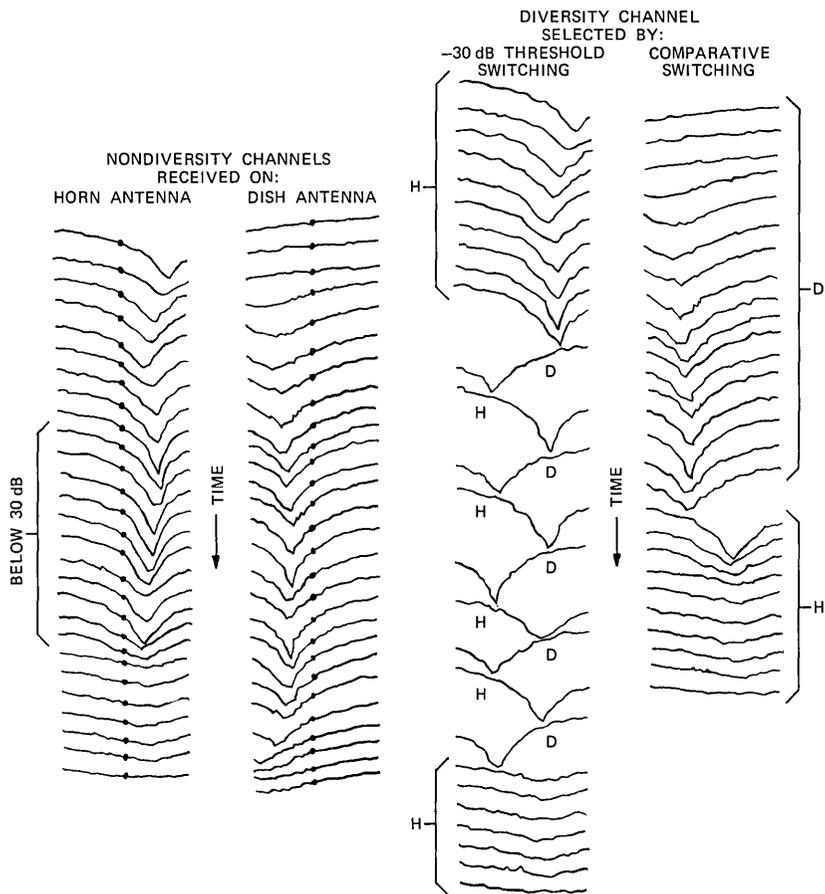
Fig. 14—Time sequential plots of the nondiversity and diversity channel transmission losses.
