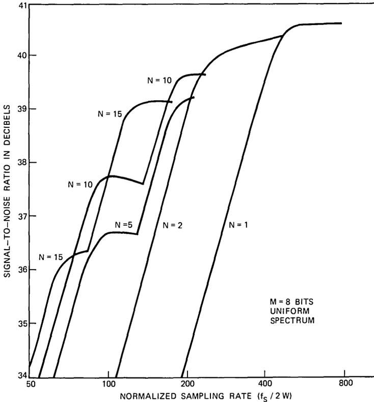
Fig. 8—Performance characteristics,  $M = 8$  bits, uniform spectrum.
