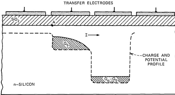
Fig. 2—Transfer of charge in a standard CCD cell with symbols defined in the text.
