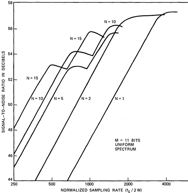
Fig. 7—Performance characteristics,  $M = 11$  bits, uniform spectrum.
