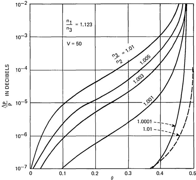
Fig. 4—Scattering losses as a function of mode angle  $\theta$ . The core index is assumed to be  $n_1 = 1.46$ , the support index is  $n_3 = 1.3$ . Core and supports are immersed in an index matching liquid. The dotted line is the reflection loss for  $n_3/n_2 = 1.01$ .
