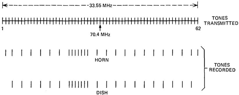
Fig. 2—Subset of tones transmitted and recorded serially on the horn reflector and dish antennas at Palmetto.
