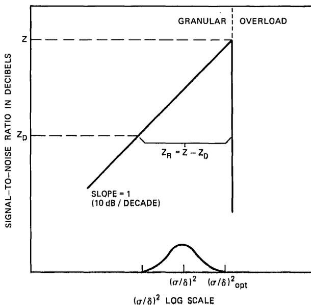
Fig. 4—Relationship of design objectives ( $Z_D, Z_R$ ) to figure of merit ( $Z$ ).
