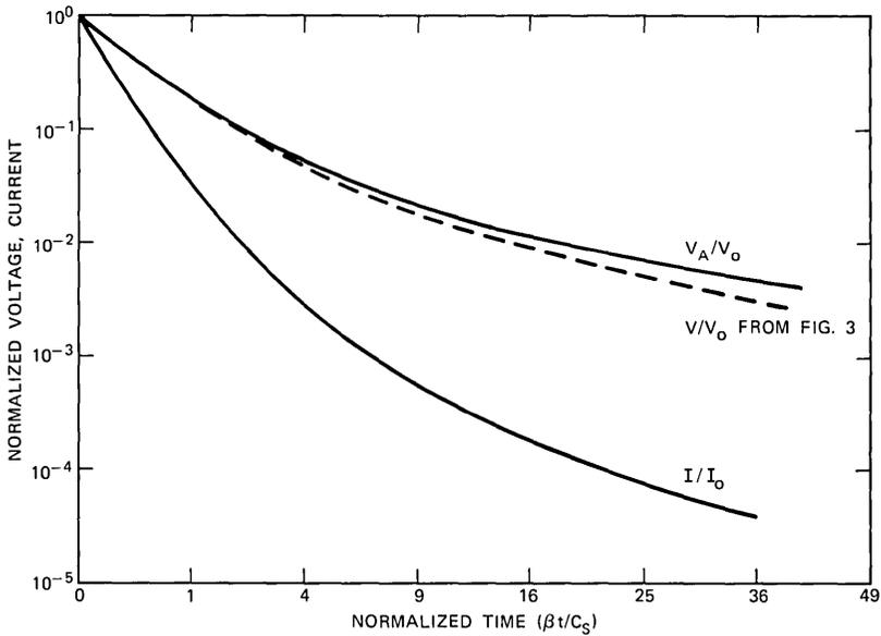
Fig. 5—Normalized voltage and current plotted as a function of normalized time for the transfer of charge from one  $p$ -region to the next in a standard IGFET bucket-brigade cell.  $V/V_o$  from Fig. 3 is shown for comparison.
