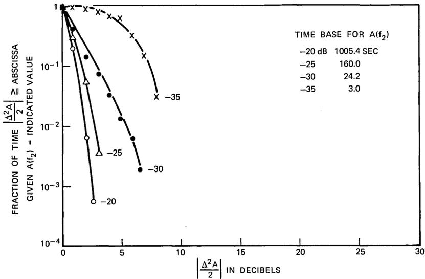
Fig. 18—Conditional quadratic distortion distributions for the 19.8-MHz, -30-dB threshold diversity channel.
