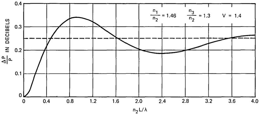
Fig. 2—Relative scattered power as a function of support thickness  $L$ . The dotted line represents eq. (16), which holds approximately for  $L \rightarrow \infty$ .
