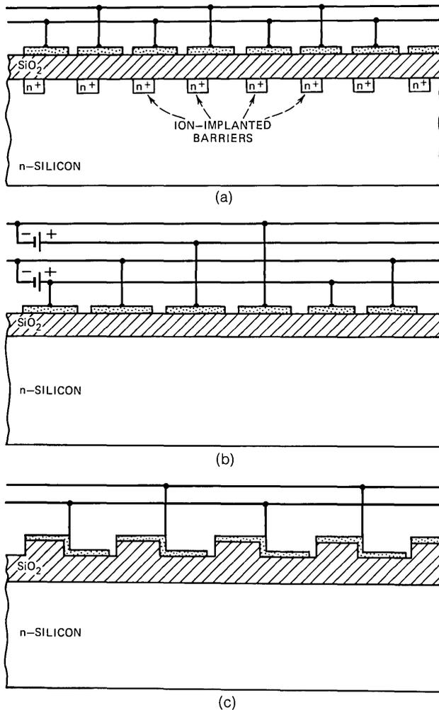
Fig. 9—Several examples of two-phase CCD device structures: (a) Ion-implanted barrier. (b) Standard four-phase run two phase. (c) Stepped-oxide.
