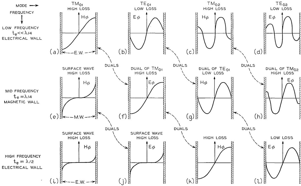
Fig. 3—Field distributions of the circular symmetric modes in unlined and lined waveguide.
