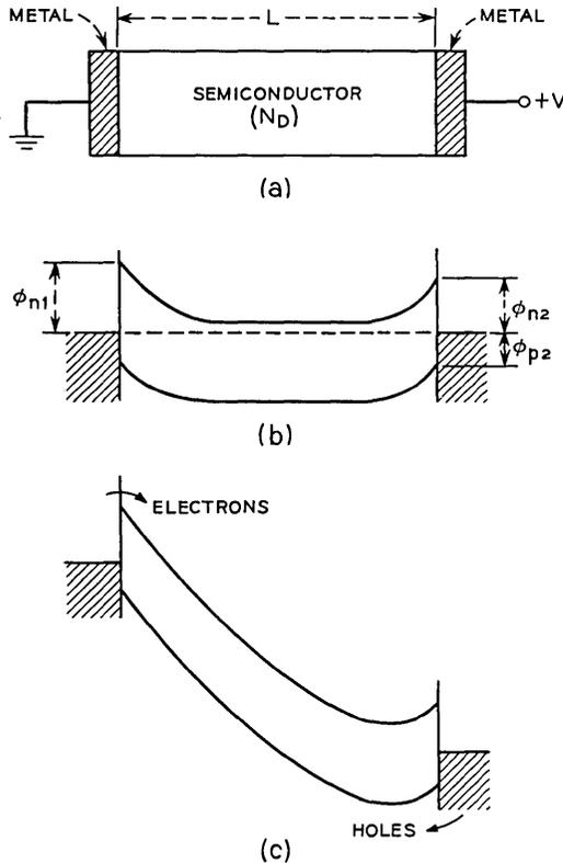
Fig. 1—(a) Schematic diagram of a metal-semiconductor-metal (MSM) structure. (b) Energy band diagram of an MSM structure in thermal equilibrium. (c) Energy band diagram of an MSM structure under biasing condition.
