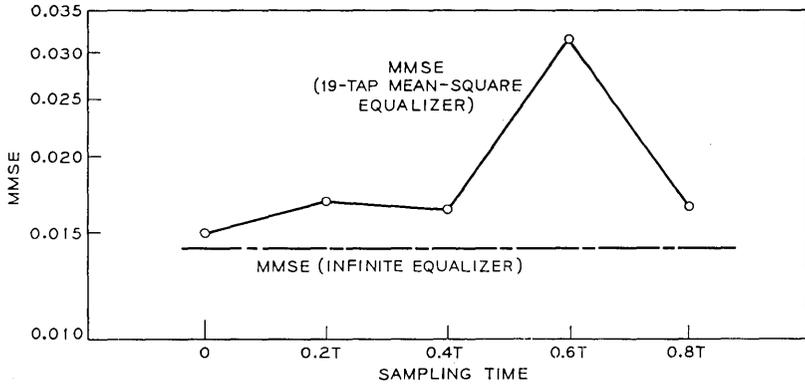
Fig. 9—M.M.S.E. versus sampling time; SSB class IV partial-response system; baseband equivalent channel transfer function,  $\{1 - 0.1 [|\omega|/(\pi/T)]\} \exp - j(\omega^3 \beta_m T^3/3\pi^2)$ ; demodulating carrier phase,  $\theta = 60^\circ$ ,  $(S/N)_{\text{input}} = 21$  dB.
