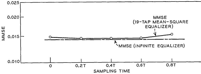
Fig. 5—M.M.S.E. versus sampling time; SSB class IV partial-response system; baseband equivalent channel transfer function,  $\{1 - 0.1 [|\omega|/(\pi/T)]\} \exp - j(\omega^3 \beta_m T^3/3\pi^2)$ ; demodulating carrier phase,  $\theta = -15^\circ$ ,  $(S/N)_{input} = 21$  dB.
