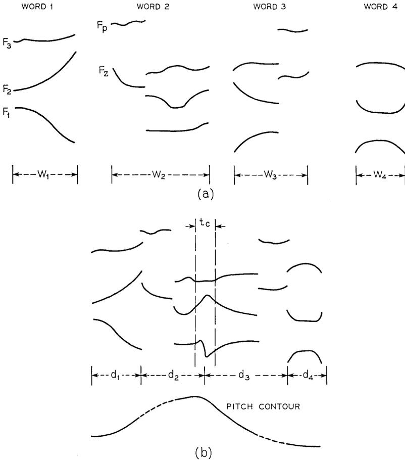
Fig. 4—Typical example of how control parameters are generated from the word library store. A message composed of four words is illustrated. All parameters are functions of time.
