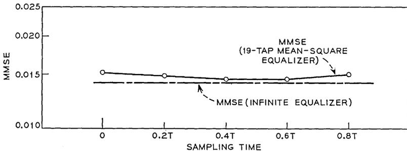
Fig. 4—M.M.S.E. versus sampling time; SSB class IV partial-response system; baseband equivalent channel transfer function,  $\{1 - 0.1 [|\omega|/(\pi/T)]\} \exp - j(\omega^3 \beta_m T^3/3\pi^2)$ ; demodulating carrier phase,  $\theta = -30^\circ$ ,  $(S/N)_{input} = 21$  dB.
