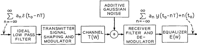
Fig. 1—Digital data system, simplified block diagram.
