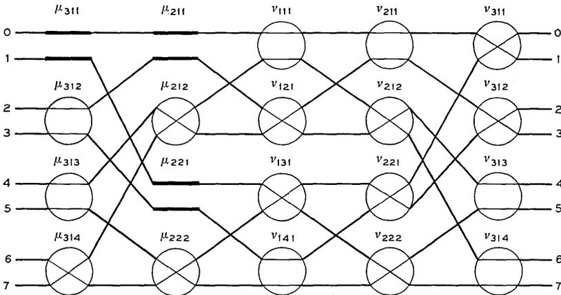
Fig. 2— $\beta$ -element setting for  $P = \begin{pmatrix} 01234567 \\ 17403526 \end{pmatrix}$ .
