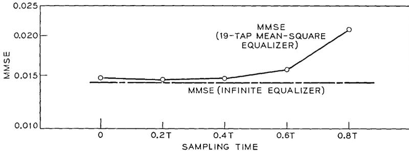
Fig. 7—M.M.S.E. versus sampling time; SSB class IV partial-response system; baseband equivalent channel transfer function,  $\{1 - 0.1 [|\omega|/(\pi/T)]\} \exp - j(\omega^3\beta_m T^3/3\pi^2)$ ; demodulating carrier phase,  $\theta = 15^\circ$ ,  $(S/N)_{input} = 21$  dB.
