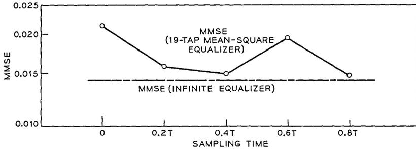
Fig. 3—M.M.S.E. versus sampling time; SSB class IV partial-response system; baseband equivalent channel transfer function,  $\{1 - 0.1 [|\omega|/(\pi/T)]\} \exp - j(\omega^3 \beta_m T^3/3\pi^2)$ ; demodulating carrier phase,  $\theta = -60^\circ$ ,  $(S/N)_{input} = 21$  dB.
