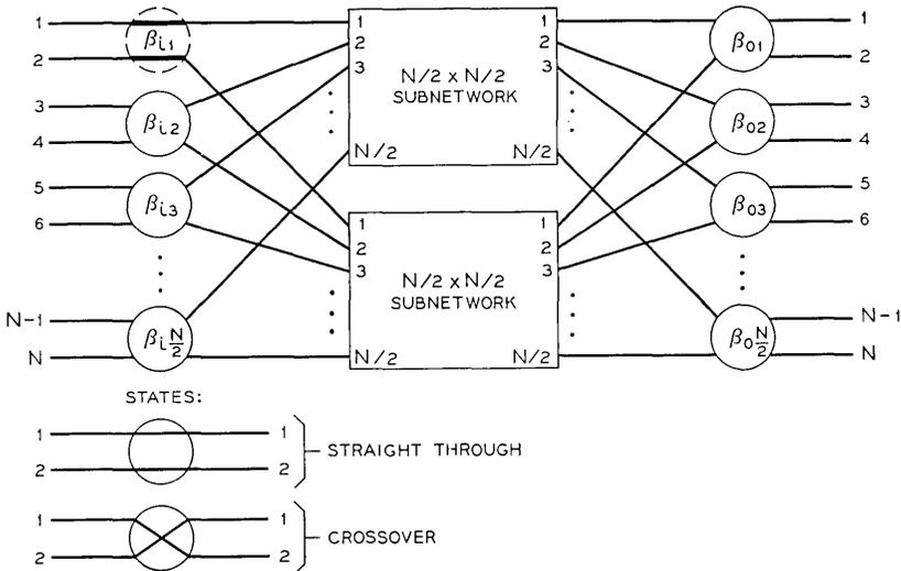
Fig. 5—Base-2  $(N \times N)$  rearrangeable switching network.
