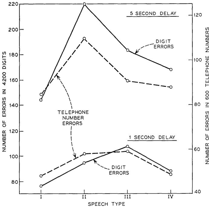
Fig. 7—Experimental results showing the total number of digit errors and telephone number errors. Four types of speech are tested: I, natural digits; II, natural, abutted digits; III, synthetic abutted digits; IV, concatenated digits. Response delays of 1 and 5 seconds are tested.
