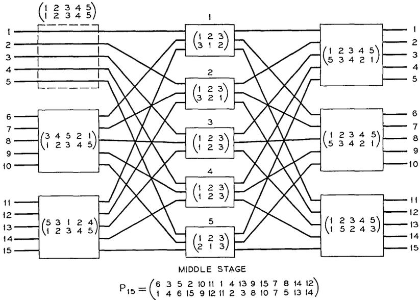
Fig. 4—A (15 × 15) network with permutations assignment.
