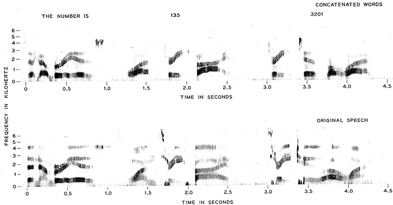
Fig. 5—Spectrogram comparison between synthetic and natural versions of a typical telephone number.
