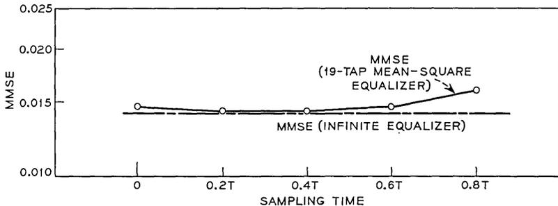
Fig. 6—M.M.S.E. versus sampling time; SSB class IV partial-response system; baseband equivalent channel transfer function,  $\{1 - 0.1 [|\omega|/(\pi/T)]\} \exp - j(\omega^3 \beta_m T^3/3\pi^2)$ ; demodulating carrier phase,  $\theta = 0^\circ$ ,  $(S/N)_{input} = 21$  dB.
