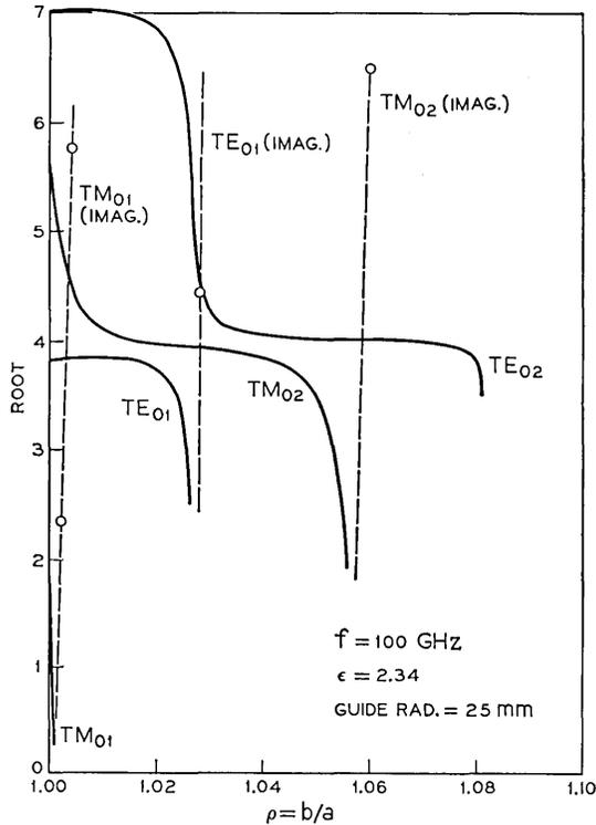
Fig. 5—Eigenvalues for circular symmetric modes in lined waveguide.
