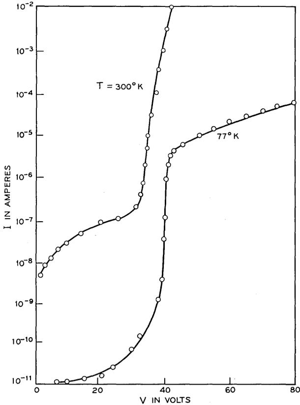
Fig. 2—Measured current vs voltage of a silicon MSM structure (PtSi-Si-PtSi) at two temperatures. The device parameters are  $L = 10 \mu\text{m}$ ,  $N_D = 4 \times 10^{14} \text{ cm}^{-3}$ ,  $\phi_{n1} = \phi_{n2} = 0.85 \text{ eV}$ , and with an area of  $5 \times 10^{-4} \text{ cm}^2$ .
