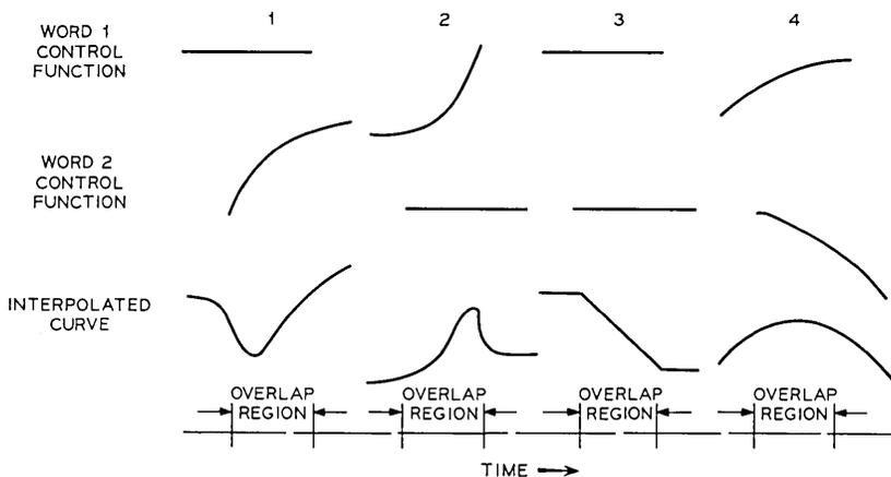
Fig. 3—Interpolation of control parameter contours for four typical cases.
