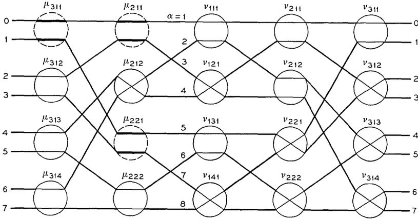
Fig. 3— $\beta$ -element setting for  $T(8) = \begin{pmatrix} 01234567 \\ 02743651 \end{pmatrix}$ .
