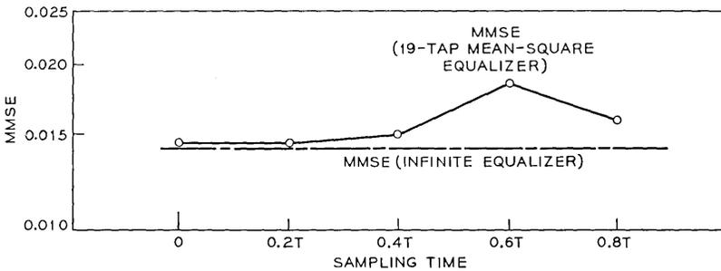
Fig. 8—M.M.S.E. versus sampling time; SSB class IV partial-response system; baseband equivalent channel transfer function,  $\{1 - 0.1 [|\omega|/(\pi/T)]\} \exp - j(\omega^3\beta_m T^3/3\pi^2)$ ; demodulating carrier phase,  $\theta = 30^\circ$ ,  $(S/N)_{input} = 21$  dB.
