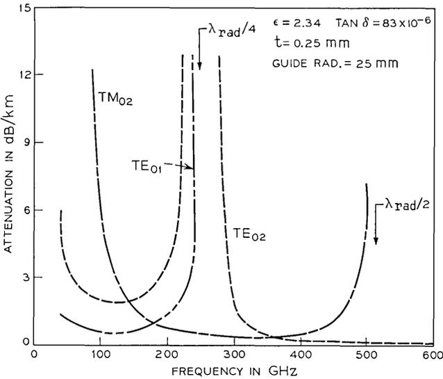
Fig. 2—Loss characteristics of circular symmetric modes in lined waveguide (wall impedance model).
