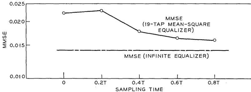
Fig. 10—M.M.S.E. versus sampling time; SSB class IV partial-response system; baseband equivalent channel transfer function,  $\{1 - 0.1 [|\omega|/(\pi/T)]\} \exp - j(\omega^3 \beta_m T^3/3\pi^2)$ ; demodulating carrier phase,  $\theta = 90^\circ$ ,  $(S/N)_{\text{input}} = 21$  dB.
