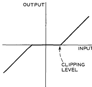
Fig. 5—Center-clipping transfer function implemented in analogue circuits.
