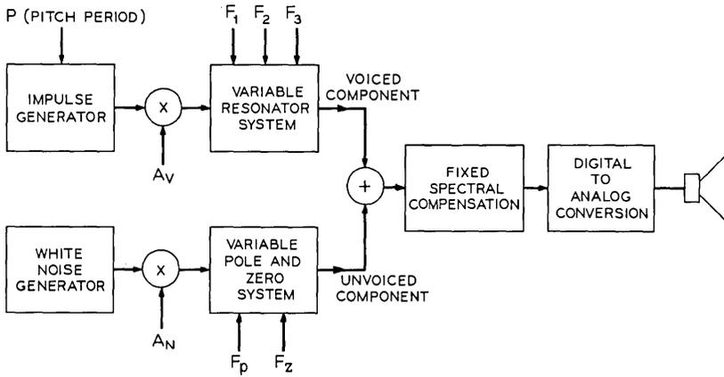
Fig. 1—Digital formant synthesizer, block diagram.
