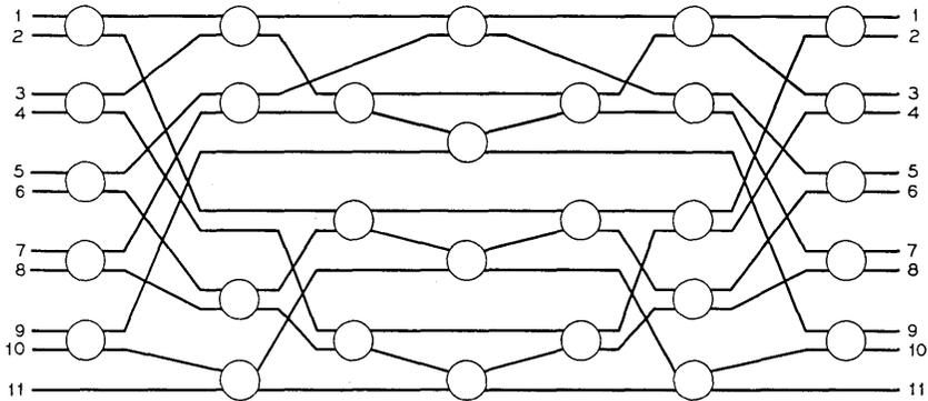
Fig. 3—An  $(11 \times 11)$  network with base-2 structure.
