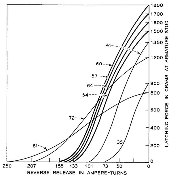
Fig. 7 — Magnetic latching characteristics of additional hold magnets with cores of different physical hardness.
