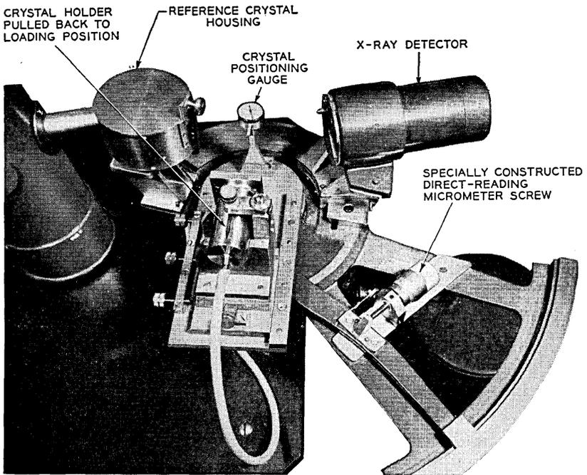
Fig. 5 — Double-crystal goniometer used for orientation measurements.
