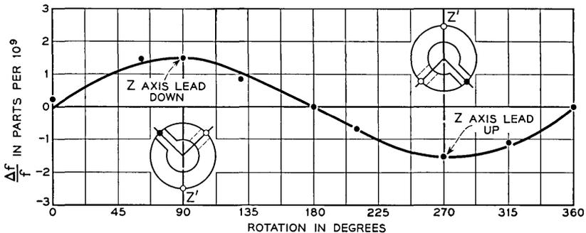
Fig. 15 — Effect of gravity-induced strains on frequency at 2.5 mc.
