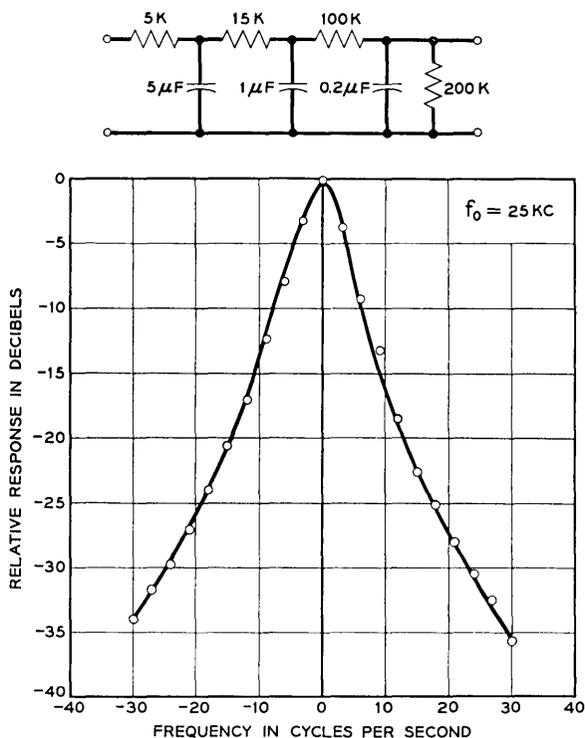
Fig. 12 — Frequency response and one of the constituent equivalent low-pass networks for sampled-data filter.
