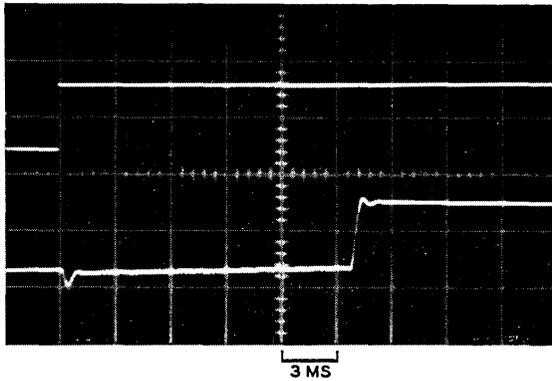
Fig. 9 — Measured step response of delay network.
