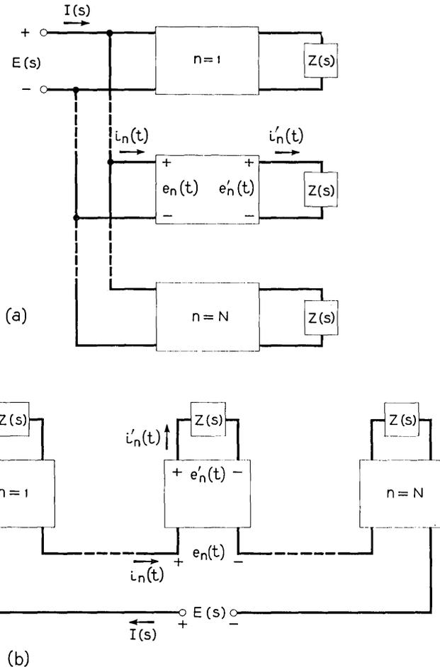
Fig. 3 — Forms taken by network when  $U(s)$  and  $V(s)$  are interpreted as corresponding to transforms of voltage and current at same port.
