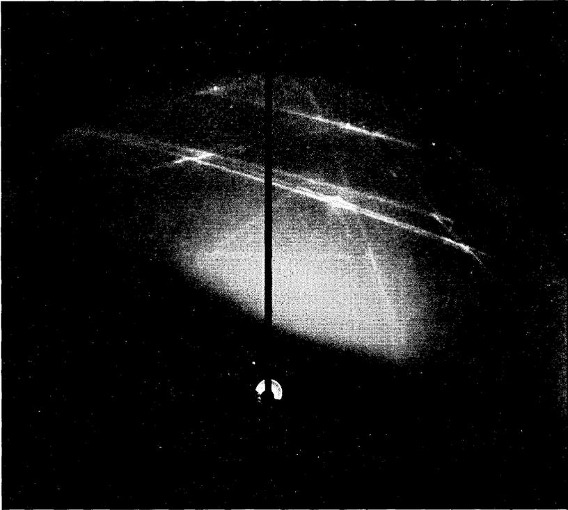
Fig. 7 — Electron diffraction pattern, showing Kikuchi lines.
