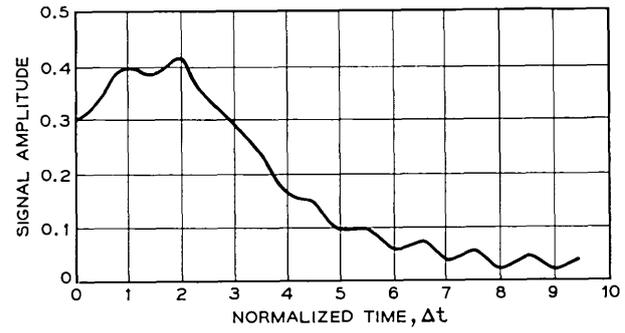
Fig. 36 — Quadratic phase distortion effects, unweighted pulse,  $\varphi = 2\pi$ .
