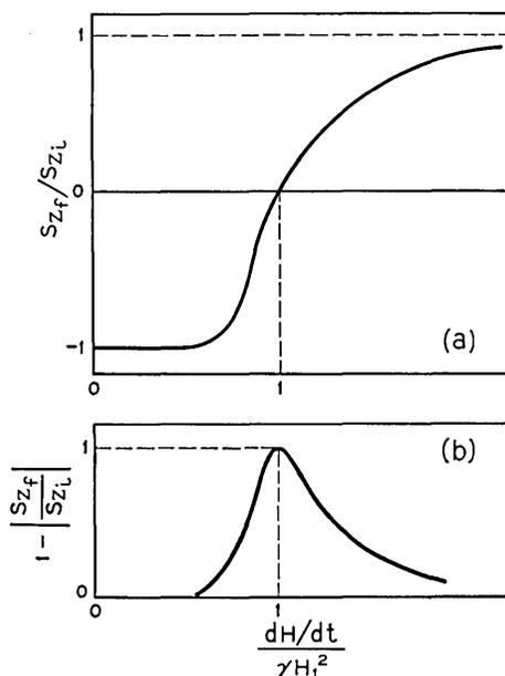
Fig. 11 — Loss of magnetization per passage due to nonadiabaticity (or non-suddenness), qualitative only. In an adiabatic transition,  $S_z \rightarrow -S_z$ ; in a sudden transition,  $S_z \rightarrow S_z$ ; in both cases, there is no loss of  $|S_z|$ . In an intermediate transition, there is a loss in  $|S_z|$ ;  $S_{zi}$  and  $S_{zf}$  are the initial and final values of  $S_z$ , respectively.
