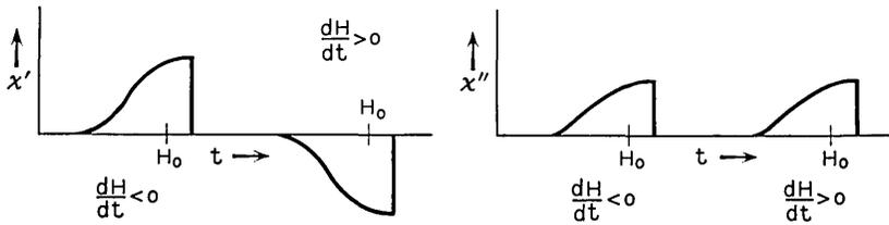
Fig. 1 — Symbolic indication of the parities of  $\chi'$  and  $\chi''$  signals of systems obeying the Bloch equations. Under  $dH/dt \rightarrow -dH/dt$ , we have:  $\chi'(H - H_0) \rightarrow -\chi'(H_0 - H)$ ;  $\chi''(H - H_0) \rightarrow \chi''(H_0 - H)$ .
