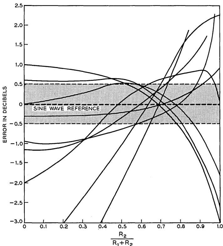
Fig. 11 — “Quasi-rms” detector error for several functions.
