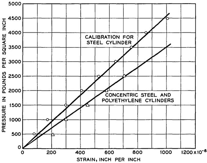
Fig. 5 — Pressure vs. strain from gage 1.
