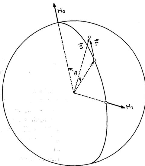
Fig. 46 — Position of magnetization vector in space.
