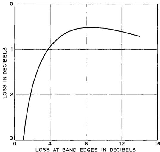
Fig. 9 — Degradation in S/N from ideal maximum when the rectangular Chirp signal passes through the delay equalizer and a smooth, gaussian-taper filter, which introduces a loss of  $L$  db at the band edges.
