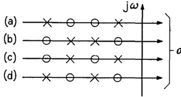
Fig. 10 — Permissible pole-zero patterns for  $Z_3/Z_4$ .
