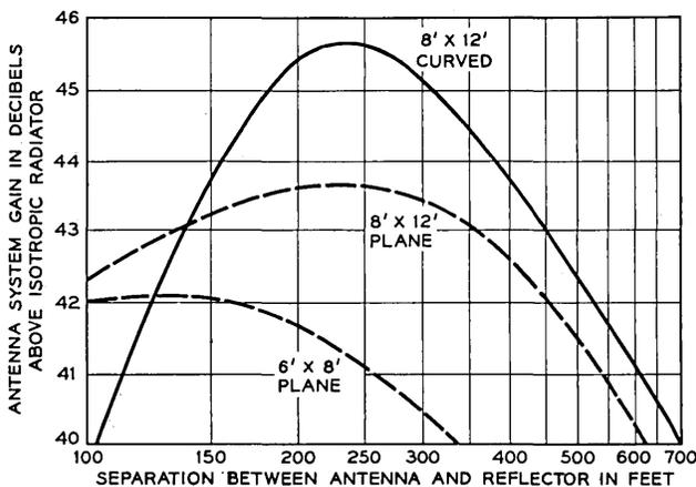
Fig. 30 — Gain of periscope antenna system.
