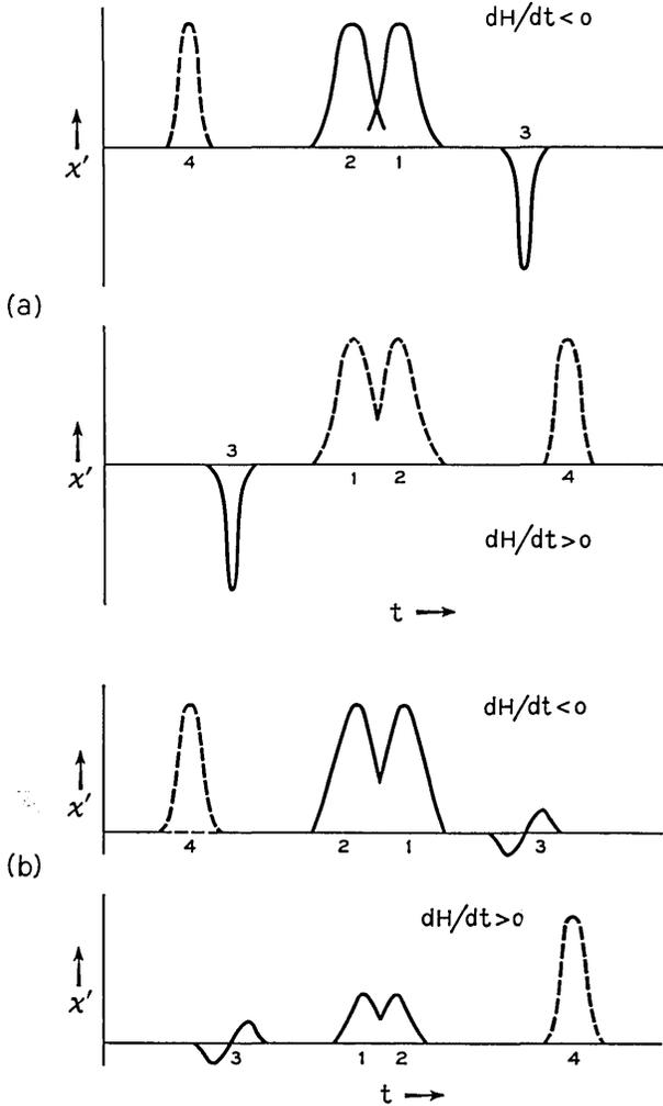
Fig. 7 — (a) The  $x'$  signal expected from the system with energy levels shown in Fig. 5 when *all* transitions (including those of the forbidden lines), are adiabatic; line 4 is assumed to be *strictly* forbidden, while line 3 is not; there is *no* simple symmetry under  $dH/dt \rightarrow -dH/dt$ . (b) The  $x'$  signal from the system with the energy level diagram shown in Fig. 5, when line 3 is *not* passed adiabatically.
