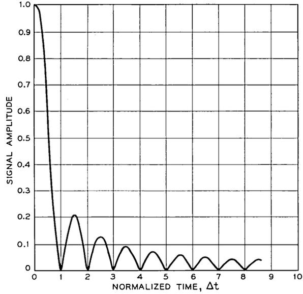
Fig. 33—Quadratic phase distortion effects, unweighted pulse,  $\varphi = 0$ .
