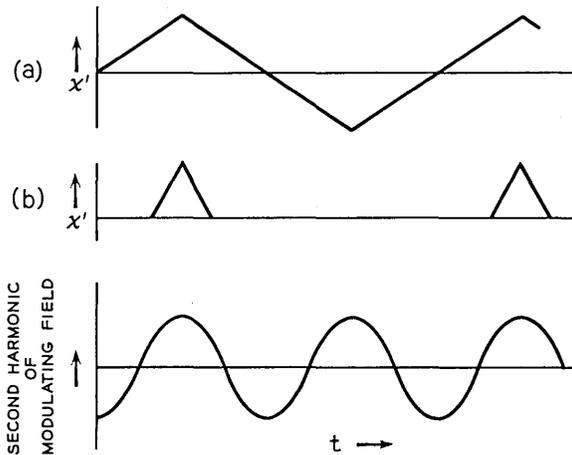
Fig. 44 — Demonstration of the strong harmonic content of "fresh" signals: (a)  $\chi'$  of case 7 (stale); (b)  $\chi'$  of case 8 (fresh). Note that the "stale" signal possesses only odd harmonics of the magnetic field modulation frequency, while the "fresh" signal possesses a strong second harmonic component.
