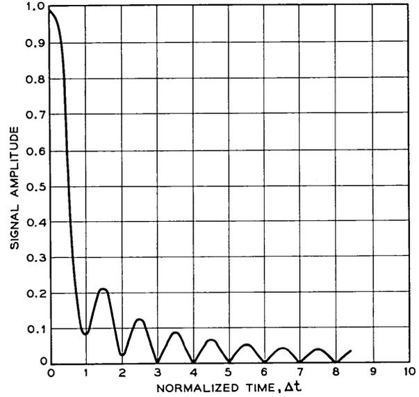
Fig. 34—Quadratic phase distortion effects, unweighted pulse,  $\varphi = \pi/8$ .
