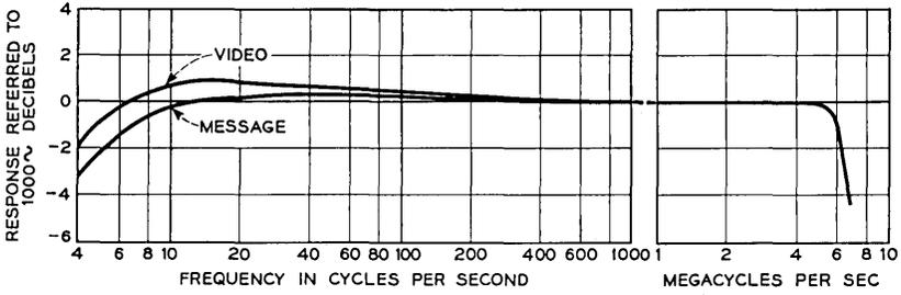
Fig. 17 — Gain-frequency characteristic of a TJ repeater.
