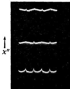
Fig. 23 —  $\chi''$  scope traces under the same conditions as those of Fig. 21. We observe slow passage signals, with some component proportional to the derivative of the line shape, due probably to incomplete saturation. ( $\gamma H_1 T_1 \approx 2$ .)
