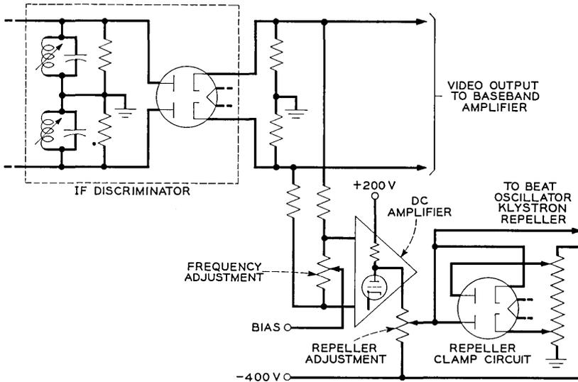
Fig. 15 — Functional schematic of the receiver AFC circuit.
