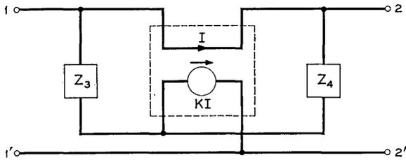
Fig. 3 — Idealized realization of the required converter.
