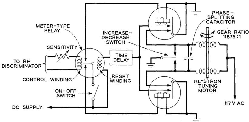
Fig. 14 — Functional schematic of the transmitter AFC circuit.
