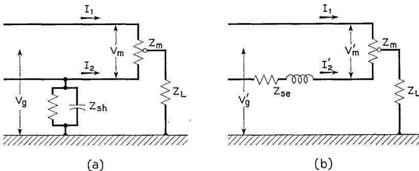
Fig. 10 — Equivalent circuit representations for (a) shunt and (b) series unbalance. For shunt unbalance,  $20 \log_{10}(V_m/V_g) = 20 \log_{10}(Z_m/4Z_{sh}) =$  balance ratio in decibels; for series unbalance,  $20 \log_{10}(V_m/V'_g) = 20 \log_{10}(Z_{se}/4Z_L) =$  balance ratio in decibels.
