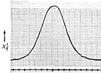
Fig. 25 — The component of  $\chi'$  in-phase with the modulating field, with higher microwave power than that used to obtain Fig. 24(a); the higher power yields a “cleaner” trace [compare with Fig. 19(a)].
