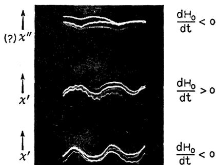
Fig. 39 — Experimental scope traces corresponding to case 8 (compare with Fig. 36): the  $\chi''$  trace is probably a spurious  $\chi'$  signal; the signal here is weak, so the signal-to-noise ratio is not good.
