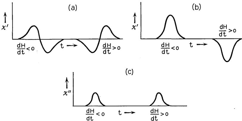
Fig. 2 — The most commonly observed  $\chi'$  signals of systems obeying the Bloch equations, for (a) slow passage and (b) rapid passage; note the symmetry under  $dH/dt \rightarrow -dH/dt$ . (c) The most commonly observed  $\chi''$  signals of a system obeying the Bloch equations, slow passage.
