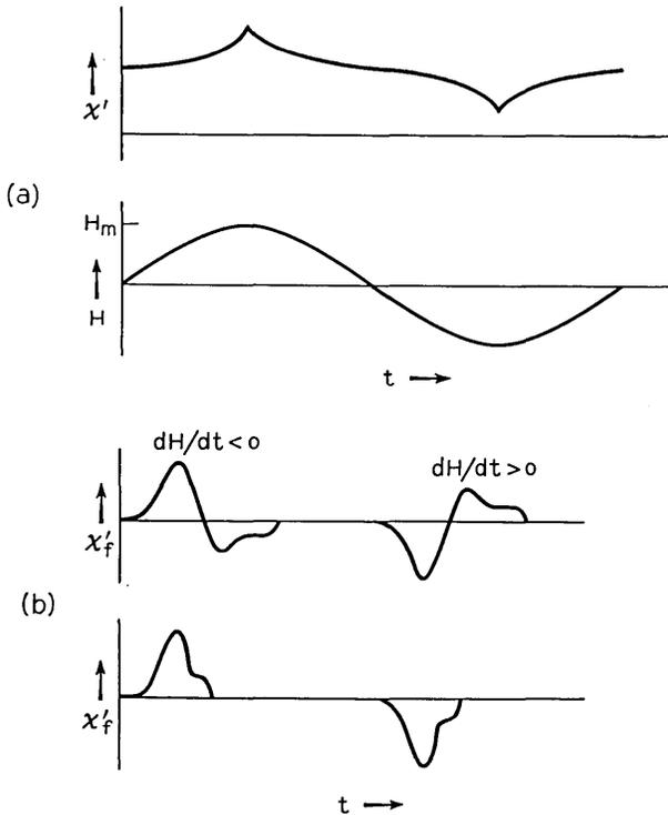
Fig. 32 — (a) Expected scope trace of case 6: spin packets just commence to “burn out”;  $\chi'$  is large, but its component at the field modulation frequency is small. (b) Expected recorder traces of hybrids of case 5 with cases 6, 7, or 8.
