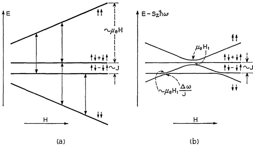
Fig. 8 — Energy levels of a system of two electrons, with a difference in hyperfine interactions of  $\hbar\Delta\omega$ , and an exchange integral  $J$  strong compared with the difference in hyperfine interactions: (a) energy levels in a fixed frame; (b) energy levels in a rotating frame. Again, an asymmetry in behavior under  $dH/dt < 0$  and  $dH/dt > 0$  is expected.
