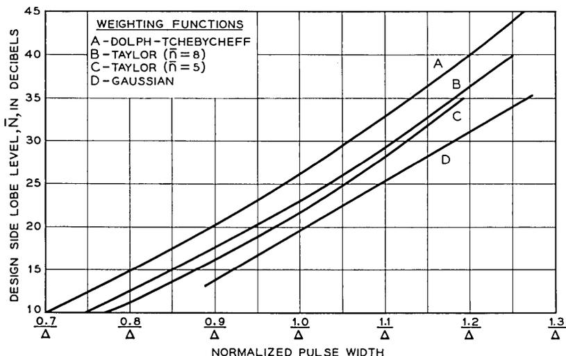
Fig. 16 — Pulse widening due to weighting.
