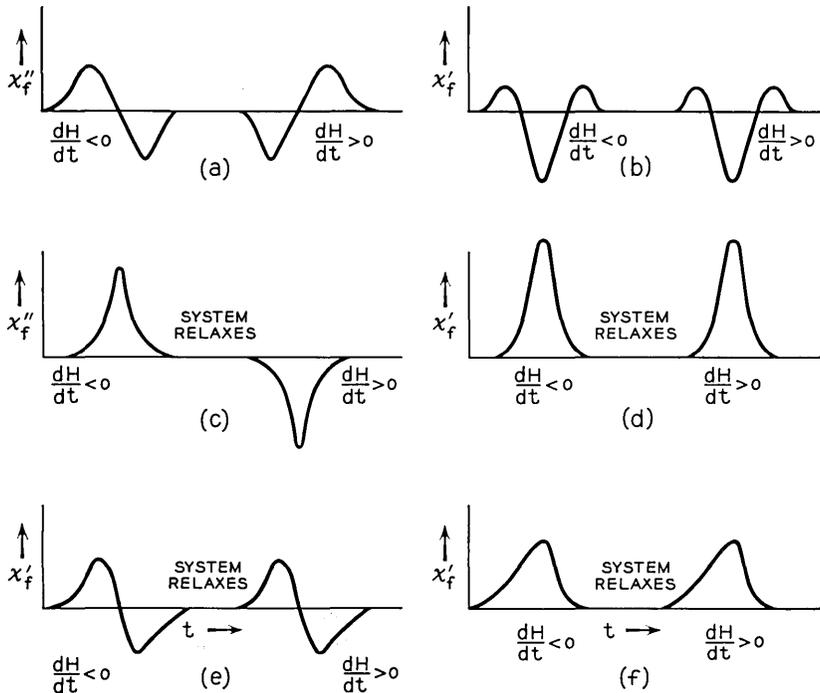
Fig. 3 — Typical traces observed when field modulation and a phase sensitive detector is used: (a)  $\chi''_f$ , slow passage; (b)  $\chi'_f$ , slow passage; (c)  $\chi''_f$ , rapid (non-adiabatic) passage; (d)  $\chi'_f$ , rapid (adiabatic) passage; (e)  $\chi'_f$ , rapid passage, very fast weep; (f)  $\chi'_f$ , a line with spin diffusion (a system *not* obeying the Bloch equations). Note the symmetry under  $dH/dt \rightarrow -dH/dt$ .
