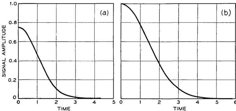
Fig. 2 — (a) Envelope of the transmitted signal when the parameter  $n = 0$ ; in this case the curve is gaussian. (b) Envelope of the “rotationally invariant” matched-filter response when  $n = 0$ ; here the curve is also gaussian.
