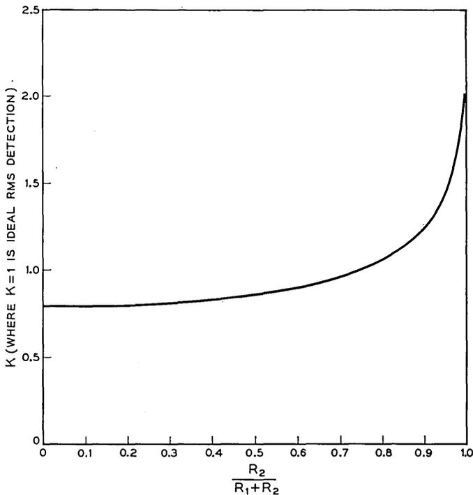
Fig. 10 — Response of the detector to gaussian-distributed noise.
