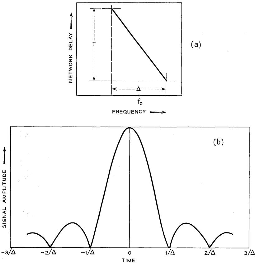
Fig. 3 — (a) Network delay vs. frequency characteristic suitable for phase equalization of the Chirp signal in Fig. 2; ideally, this network is chosen to have a flat loss characteristic. (b) Envelope of output response from the network in (a); this pulse now has a pulse width about  $1/\Delta$  and an amplitude increase given by  $\sqrt{D}$ , where  $D = T\Delta$  is called the dispersion factor.
