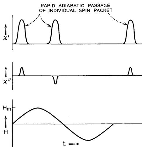
Fig. 27 — Signals from one spin packet, case 5; the spins do *not* relax between consecutive field modulation cycles, so  $\chi'$  does not change sign, while  $\chi''$ , which is due to nonperfect adiabaticity, changes sign.
