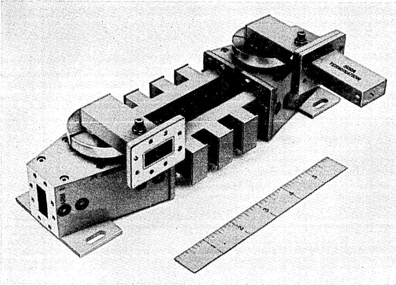
Fig. 4 — Channel separation-combining network.
