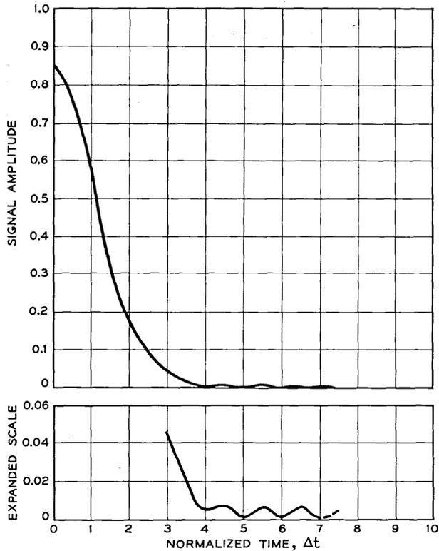
Fig. 31 — Quadratic phase distortion effects, weighted pulse,  $\varphi = \pi$ .
