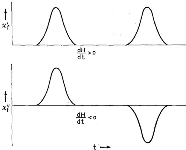
Fig. 55 — Expected recorder traces of case 11 (system relaxes between sweeps); the true line shape may be observed, sometimes even if  $H_m$  is *not* small compared with  $\Delta H$  (the width of the nonburnt region must then be small). Compare with Figs. 42(a) and (b).
