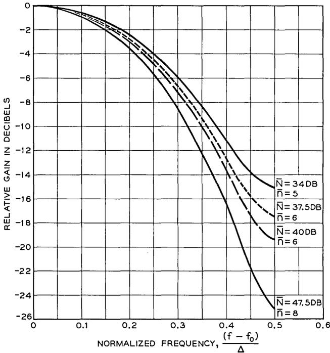
Fig. 20 — Taylor weighting characteristics for various side-lobe levels.
