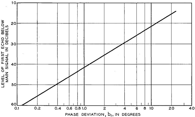
Fig. 13 — Amplitude of echo with phase distortion.
