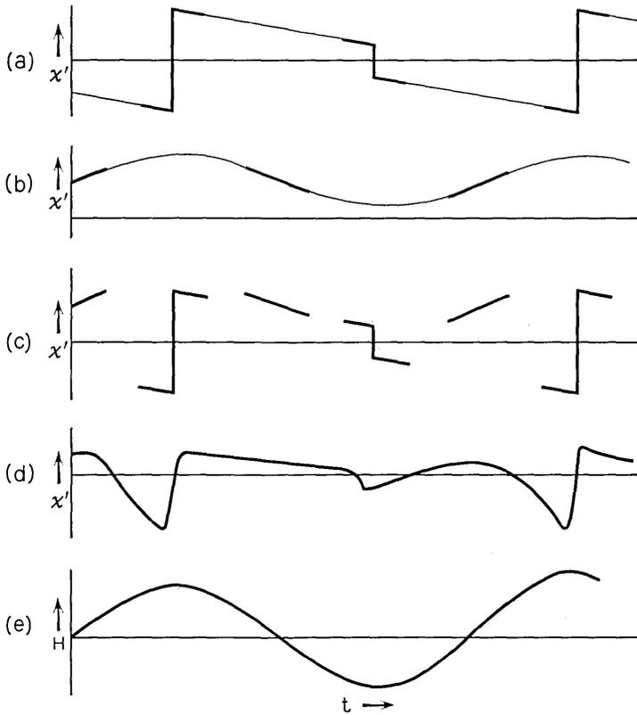
Fig. 22 — Synthesis of the  $\chi'$  trace observed in Fig. 21: (a) a case 2 signal (adiabatic rapid passage, slow modulation), on the *shoulders* of the line; (b) a case 4 signal (nonadiabatic); (c) synthesis of (a) for the portions of the modulation cycle for which  $dH/dt$  is small, and (b) for those for which  $dH/dt$  is large; (d) rough shape of the trace expected experimentally; (e) the modulating field.
