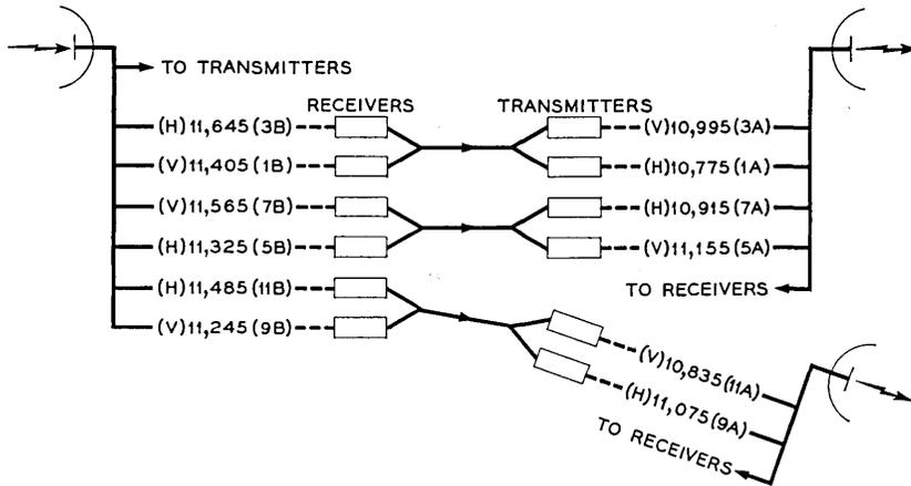
Fig. 43 — Typical frequency assignments at TJ branching point.
