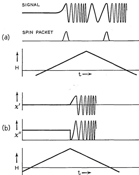
Fig. 52 — Illustration of the signal resulting from a triangular field modulation (almost sudden passage): (a) individual spin packet; (b) inhomogeneously broadened line.
