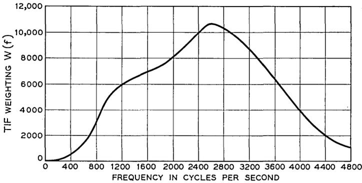
Fig. 8 — Proposed new TIF weighting curve,  $W(f) = Kw(f)M(f)$ , where  $K$  is such that  $W(1000 \text{ cycles}) = 5000$ ;  $w(f) = 10^{0.46(f)/10}$  is the C-message weighting and  $M(f) = f/1000$  to approximate the coupling distortion between power and telephone circuits.
