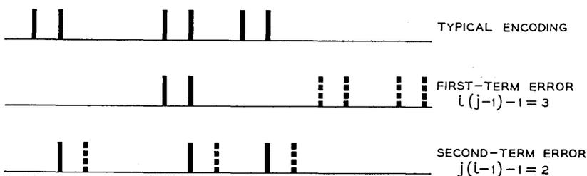
Fig. 2 — First- and second-term error for 2 | 3 code.
