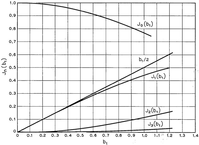
Fig. 11 — Bessel functions.
