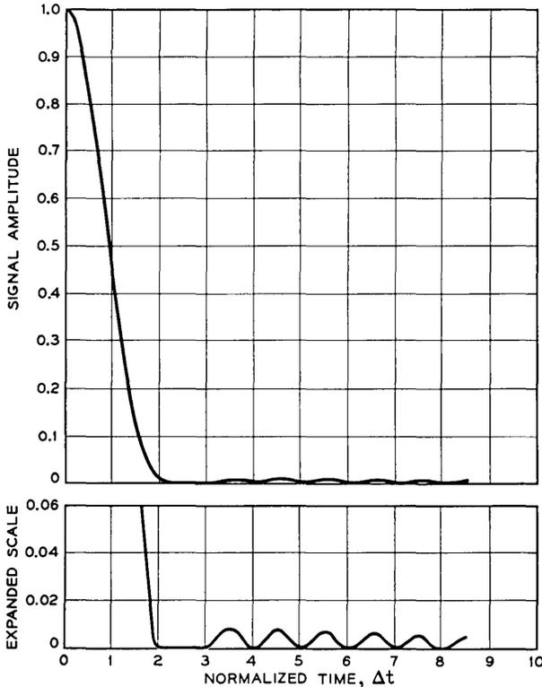
Fig. 26 — Quadratic phase distortion effects, weighted pulse,  $\varphi = 0$ .
