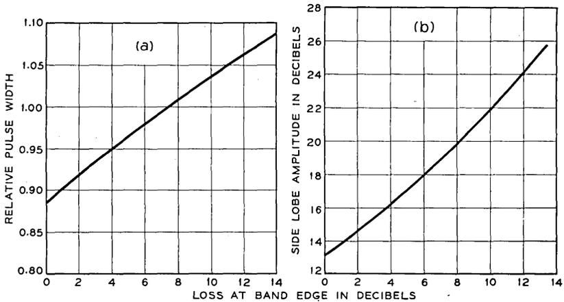
Fig. 10 — (a) Half-power pulse width increase vs.  $L$ , the gaussian filter band edge loss. (b) The relative amplitude between the maximum of the first adjacent side lobe and the central maximum of the output signal following shaping by a gaussian filter.
