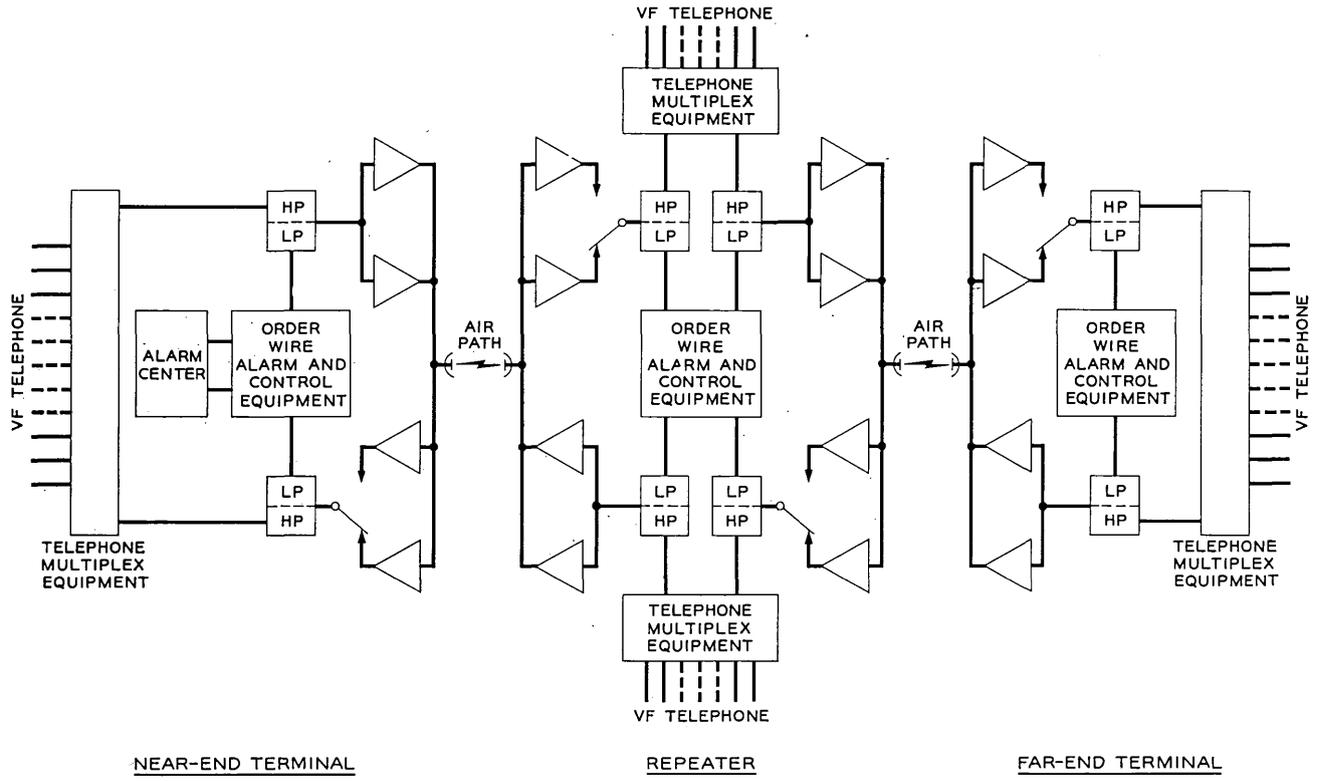
Fig. 1 — Block schematic of a two-section TJ system.
