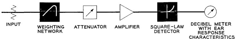
Fig. 7 — Schematic of 2A Noise Measuring Set.
