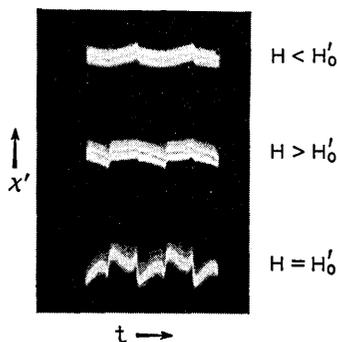
Fig. 21 —  $\chi'$  scope traces of rapid, nonadiabatic passage of a line, when  $T_1$  is very short compared with the field modulation cycle, at the center of the line (bottom trace), and on both sides of it (top and center traces).
