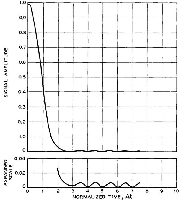
Fig. 28 — Quadratic phase distortion effects, weighted pulse,  $\varphi = \pi/6$ .
