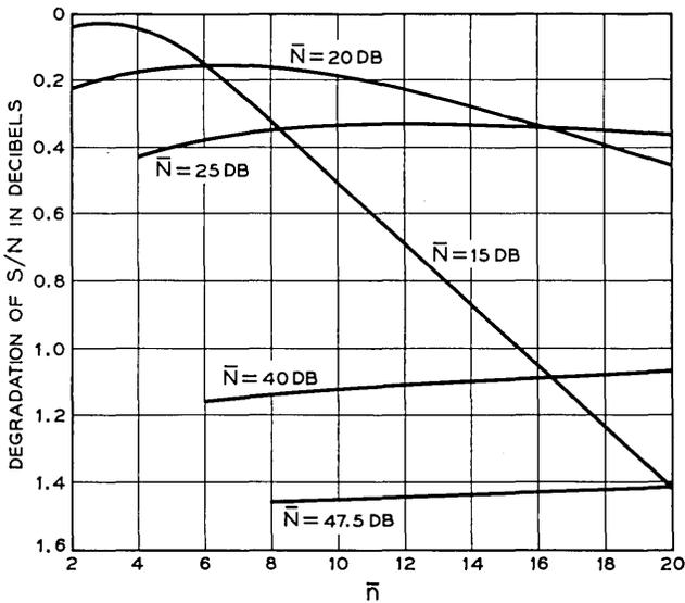
Fig. 25 — Signal-to-noise effects.
