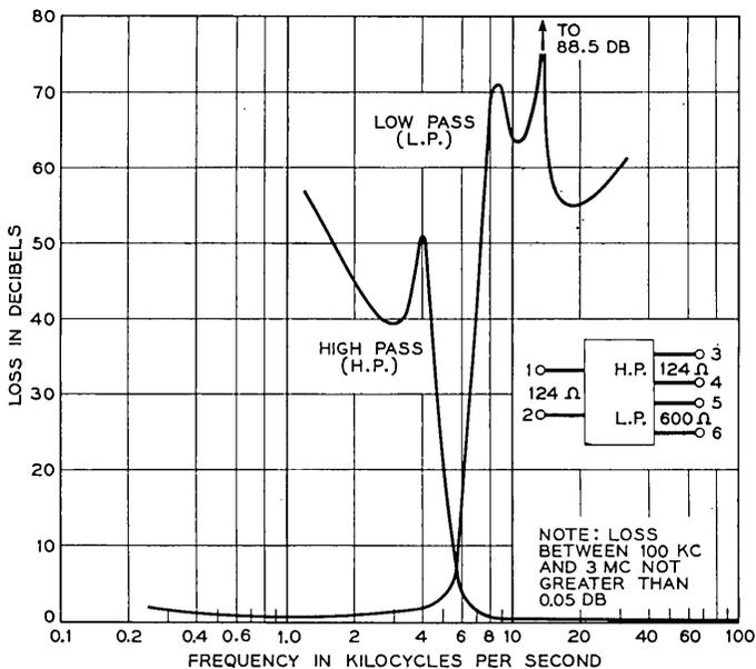
Fig. 21 — Typical loss-frequency characteristics of baseband split-apart filters.
