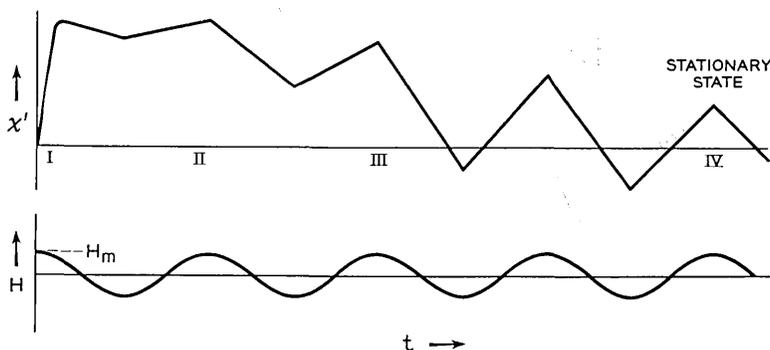
Fig. 31 — Transient  $\chi'$  trace, for illustration of case 6:  $\chi'$  is first large and constant; eventually, spin packets "burn out";  $\chi'$  decreases, but its component at the field modulation frequency may increase.
