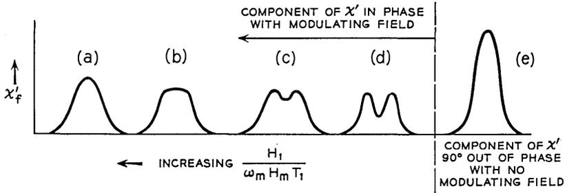
Fig. 19 — Expected recorder traces for rapid (adiabatic or nonadiabatic) passage, with a field modulation period long compared with, or of the same order, as  $T_1$ : (a) large  $H_1$ , small  $H_m$ ; (b) and (c) intermediate values of  $H_1$ ,  $H_m$ ; (d) Small  $H_1$ , large  $H_m$ . (These four are the component of  $\chi'_f$  in-phase with the field modulation.) (e) Component of  $\chi'_f$  90° out-of-phase with the field modulation.
