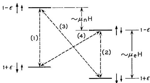
Fig. 5 — Energy-level diagram of an electron-nucleus system in a magnetic field (the nuclear spin is supposed to be  $\frac{1}{2}$ ). Lines (1) and (2) are “allowed,” while lines (3), (4) are “forbidden,” but not strictly.
