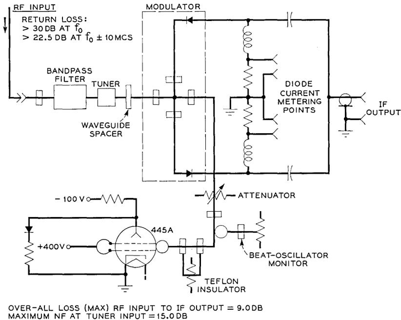
Fig. 12 — Schematic of the balanced receiving modulator.
