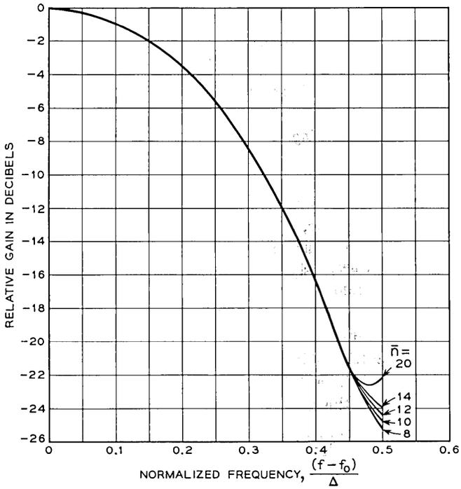
Fig. 19 — Taylor weighting characteristics for  $\bar{N} = 47.5$  db.
