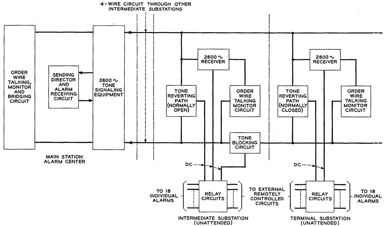
Fig. 24 — Block diagram of D2 alarm and control system.
