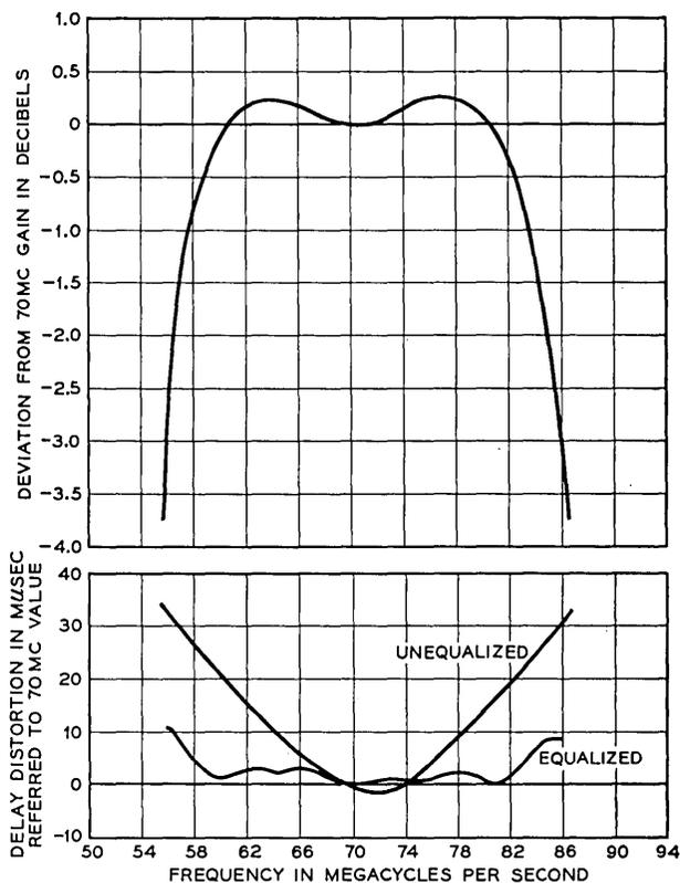
Fig. 13 — IF gain and delay characteristics.
