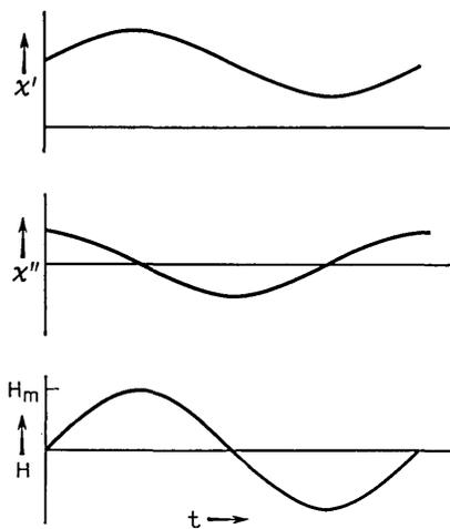
Fig. 28 — Scope traces of signal of case 5 (combination of the signals due to the individual spin packets, Fig. 27). Although  $\chi'$  is large, its component at the field modulation frequency is small, and due to the derivative of the line shape.
