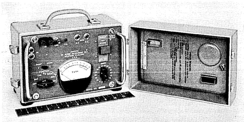
Fig. 6 — The 3A Noise Measuring Set.
