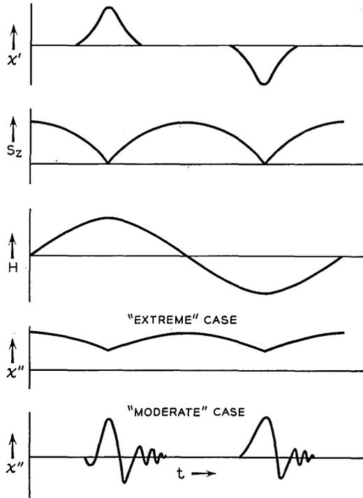
Fig. 40 — Expected scope traces of case 10:  $\chi'$  depends critically upon variations of  $S_z$ ; these may be due to "burnout," or the derivative of the line shape; here, variations due to burnout are postulated.
