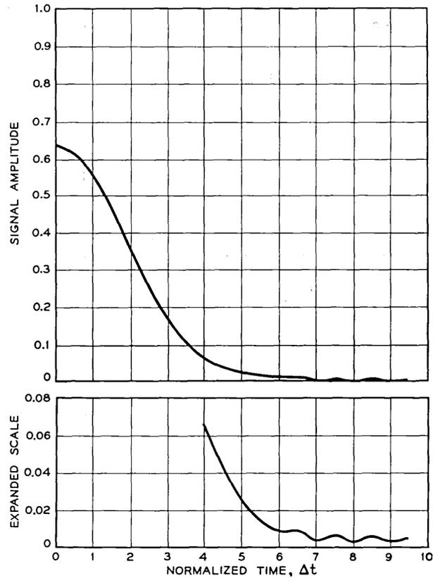
Fig. 32 — Quadratic phase distortion effects, weighted pulse,  $\varphi = 2\pi$ .
