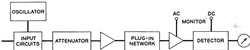
Fig. 5 — Block schematic of 3A Noise Measuring Set.
