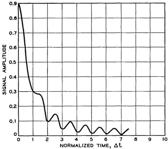
Fig. 35 — Quadratic phase distortion effects, unweighted pulse,  $\varphi = \pi/2$ .
