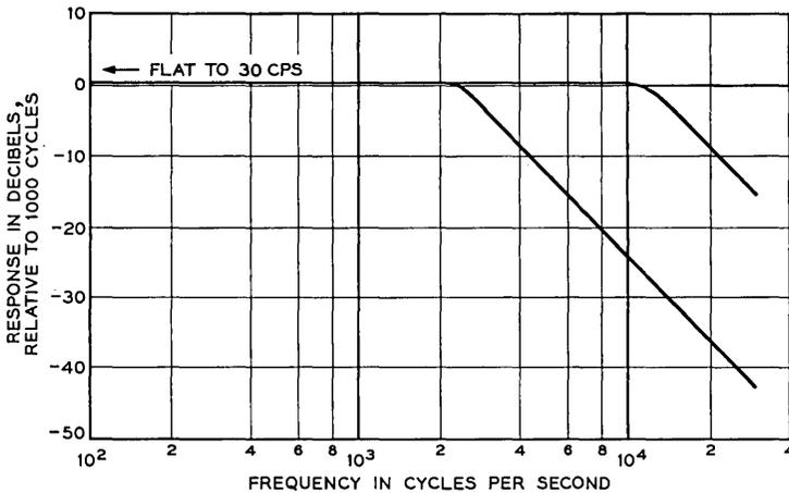
Fig. 4—Response vs. frequency of 3-ke flat and 15-ke flat weighting characteristics.
