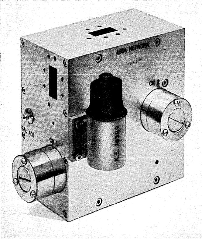
Fig. 35 — Transmitter AFC discriminator and power monitoring network.
