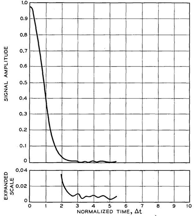
Fig. 29 — Quadratic phase distortion effects, weighted pulse,  $\varphi = \pi/4$ .
