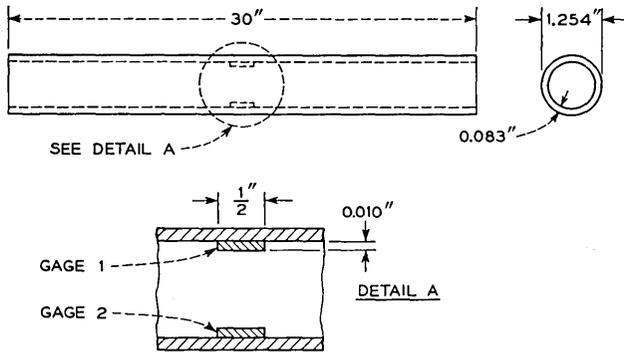
Fig. 1 — Steel tubing, showing location of strain gages.
