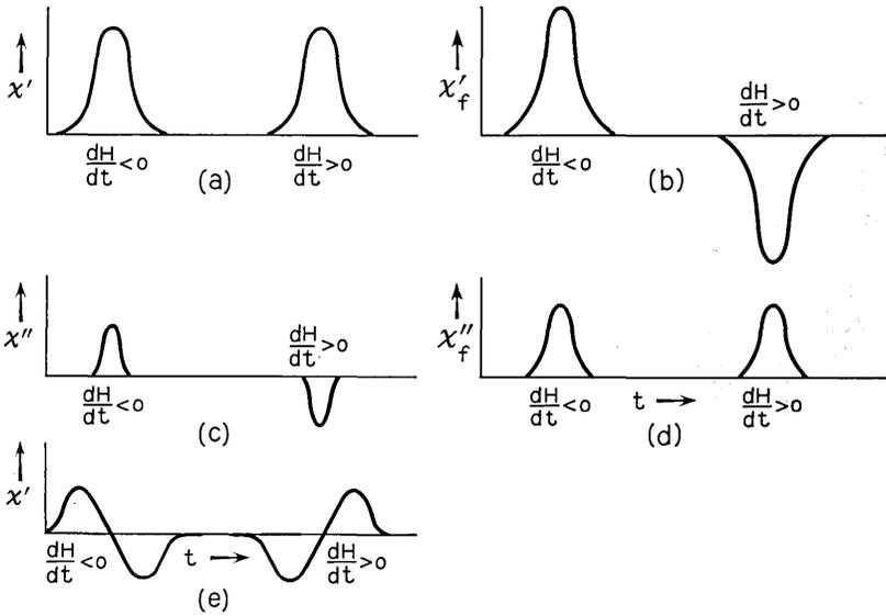
Fig. 4 — Some typical traces observed when the system does *not* relax between consecutive sweeps: (a)  $x'$ , no phase sensitive detector; (b)  $x'_f$ , with P.S.D.; (c)  $x''$ , no P.S.D. (rapid, not perfectly adiabatic, passage); (d)  $x''_f$ , with P.S.D.; (e)  $x'$ , with P.S.D., very rapid sweep. Again, notice the symmetry properties which are *different* from those occurring when the system relaxes between sweeps.
