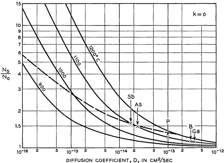
Fig. 4 — Calculated ratios of impurity surface concentration to body concentration ( $N_s/N_0$ ) produced by parabolic oxidation of silicon with zero segregation coefficient. The arrows indicate the surface concentrations predicted for the impurities indicated at 1100°C. The dashed line corresponds to the surface concentrations predicted for antimony at various temperatures.
