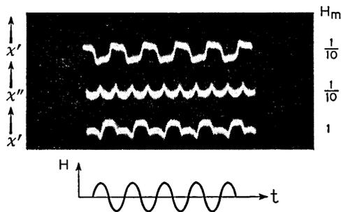
Fig. 16 — Experimental scope traces for case 2. Top trace,  $\chi'$  signal, almost ideal case "2"; center trace,  $\chi''$  signal due to slow passage near the extrema of the modulation cycle; bottom trace,  $\chi'$  signal, when the adiabatic condition is slightly violated.
