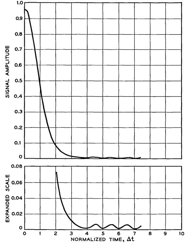
Fig. 30 — Quadratic phase distortion effects, weighted pulse,  $\varphi = \pi/2$ .
