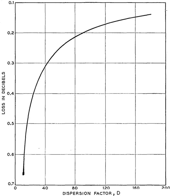
Fig. 8 — Degradation in S/N from ideal maximum when the rectangular Chirp signal passes through a delay equalizer and a sharp cutoff filter of width  $\Delta$ . The loss decreases rapidly as the dispersion factor,  $D$ , increases.
