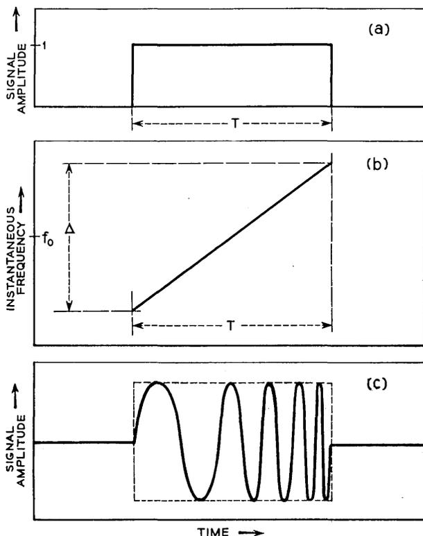
Fig. 2 — (a) Ideal envelope of actual Chirp signal, of  $T$  seconds duration and chosen to be of unit amplitude. (b) Instantaneous frequency vs. time characteristic of Chirp signal; a band of frequencies,  $\Delta$ , centered at  $f_0$  is linearly swept during the pulse duration. (c) Schematic diagram of a signal having the properties indicated in (a) and (b).
