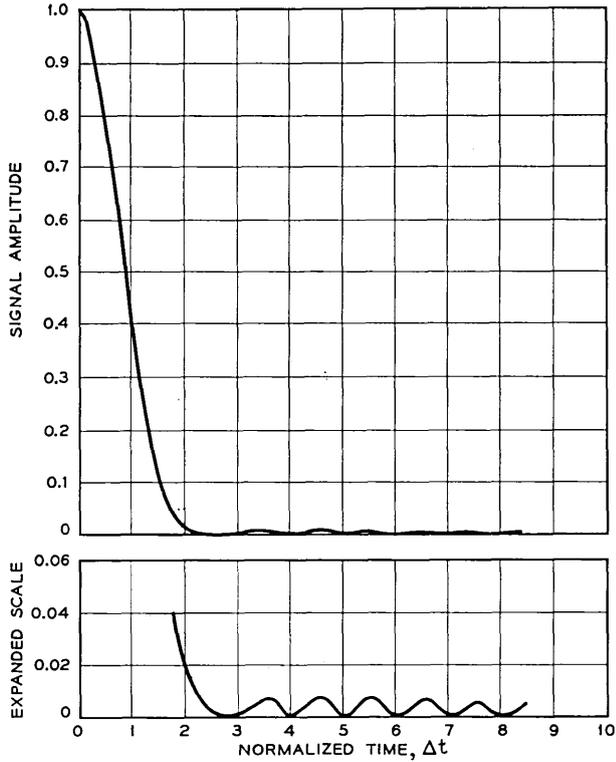
Fig. 27 — Quadratic phase distortion effects, weighted pulse,  $\varphi = \pi/8$ .
