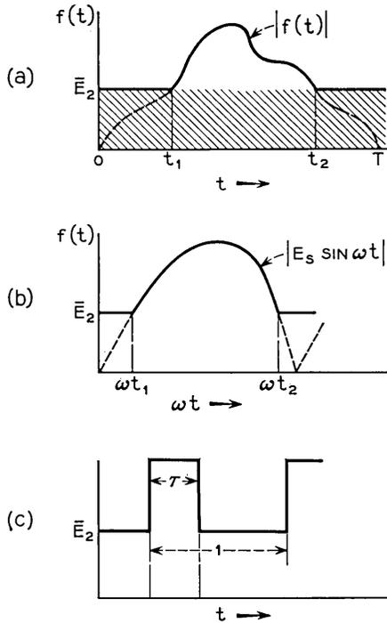
Fig. 8 — (a) Voltage across  $R_1$  and  $R_2$  with  $f(t)$  into the detector; (b) sine wave into the detector; (c) rectangular wave into the detector.
