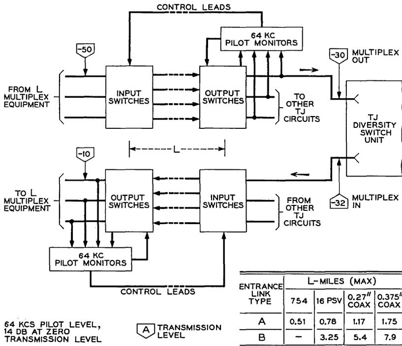
Fig. 32 — L-carrier to TJ radio entrance link.
