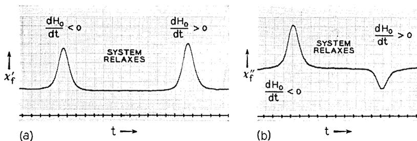
Fig. 42 — (a)  $\chi'_f$  for case 11, with P.S.D. (compare with Fig. 37); the magnetization was completely burnt out after one passage, so the sample was completely relaxed between consecutive sweeps. (b)  $\chi''_f$  for case 11, with P.S.D. Note the different parity of the  $\chi'$  and  $\chi''$  traces.
