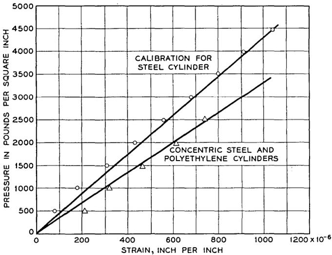
Fig. 6 — Pressure vs. strain from gage 2.
