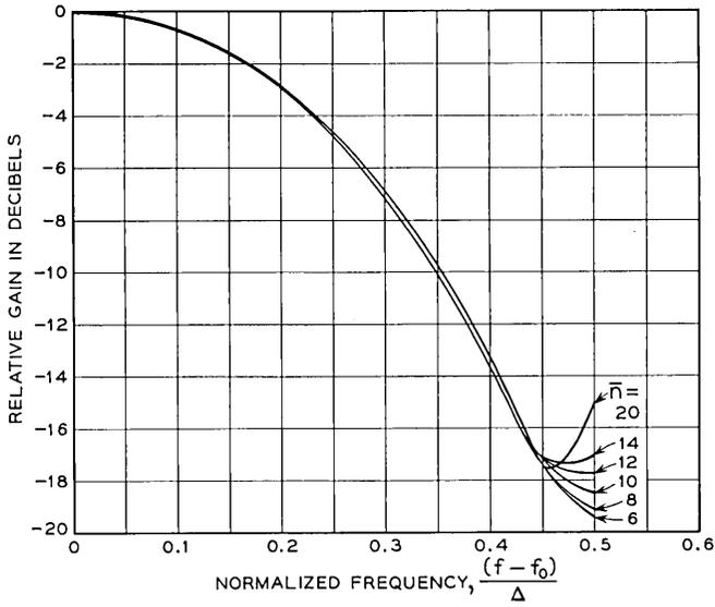
Fig. 18 — Taylor weighting characteristics for  $\bar{N} = 40$  db.
