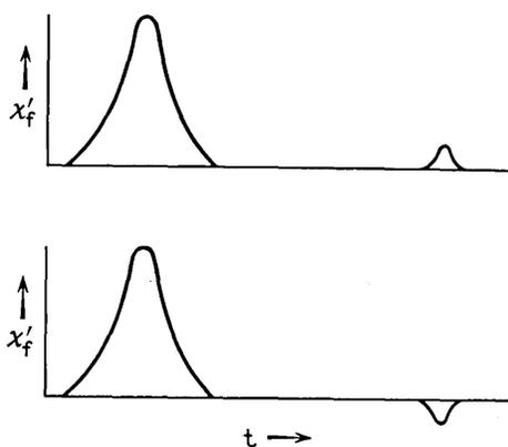
Fig. 37 — Expected recorder traces of case 8 signals: the line is burnt while sweeping through, consecutive sweeps yield weaker lines; their sign depends upon  $T_1$ , the time between consecutive sweeps, and the extent to which the line is “burnt out.”
