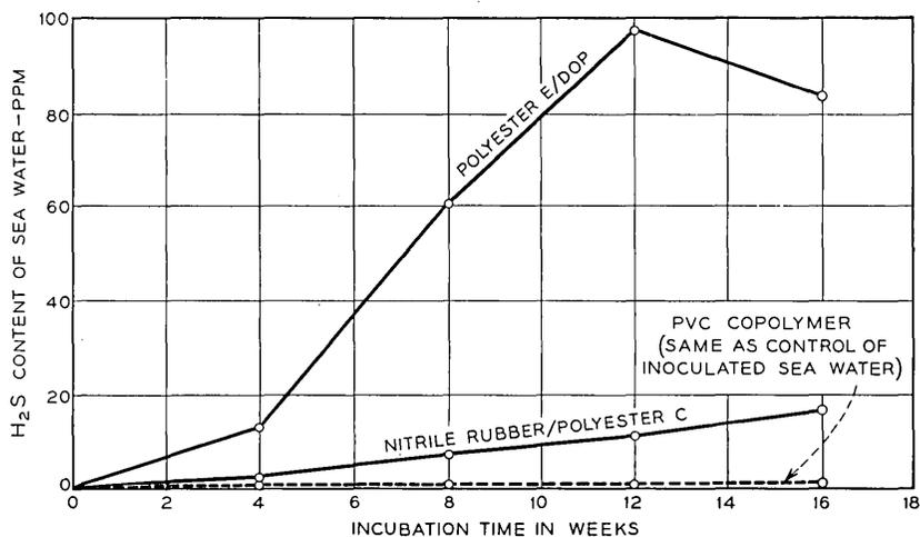
Fig. 4 — Examples of H<sub>2</sub>S production by marine bacteria in anaerobic sea water test with Poly(Vinyl Chloride) plastics as carbon source.
