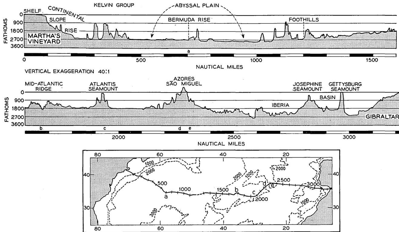
Fig. 5 — Transatlantic topographic profile, Massachusetts to Gibraltar. Vertical exaggeration 40:1.
