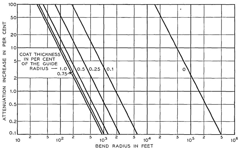
Fig. 4 — Increase in  $TE_{01}$  attenuation of a dielectric-coated guide in a uniform bend.  $2a = 2$  inches;  $\epsilon = 2.5$ ;  $\lambda = 5.4$  mm.
