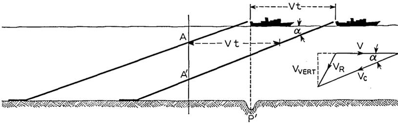
Fig. 7 — Illustration of vertical cable sinking rates.
