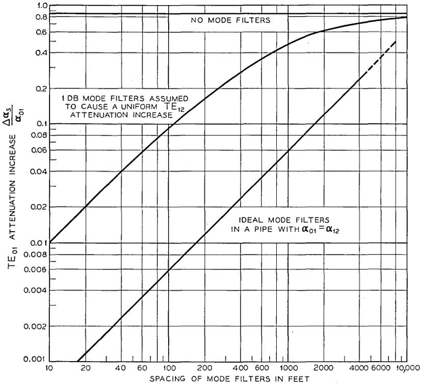
Fig. 2 — TE<sub>01</sub> attenuation increase of TE<sub>01</sub>-TE<sub>12</sub> coupling in serpentine bends with mode filters; 2-inch I.D. 2 $\frac{3}{8}$ -inch O.D.,  $\lambda = 5.4$  mm. Serpentine bends are caused by equally spaced supports and the elasticity of the copper pipe. The supporting distance is a multiple of the beat-wavelength between TE<sub>01</sub> and TE<sub>12</sub>.
