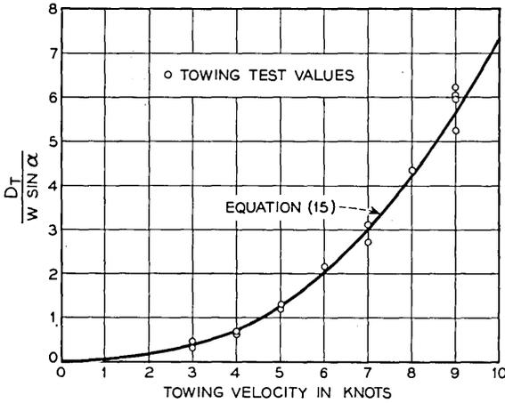
Fig. 6 — Experimental values of the tangential drag force for cable No. 2 compared with those obtained by equation (15).
