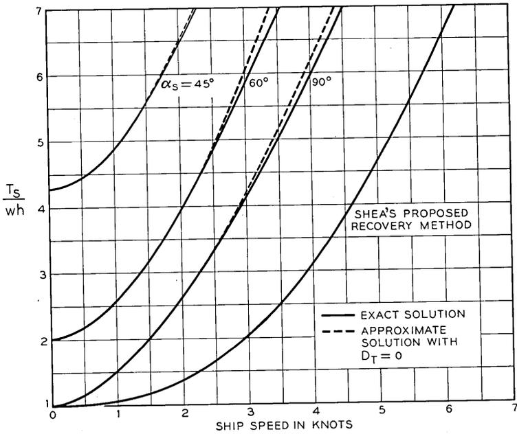
Fig. 13 — Variation of exact and approximate tension factors for recovery of cable No. 2.
