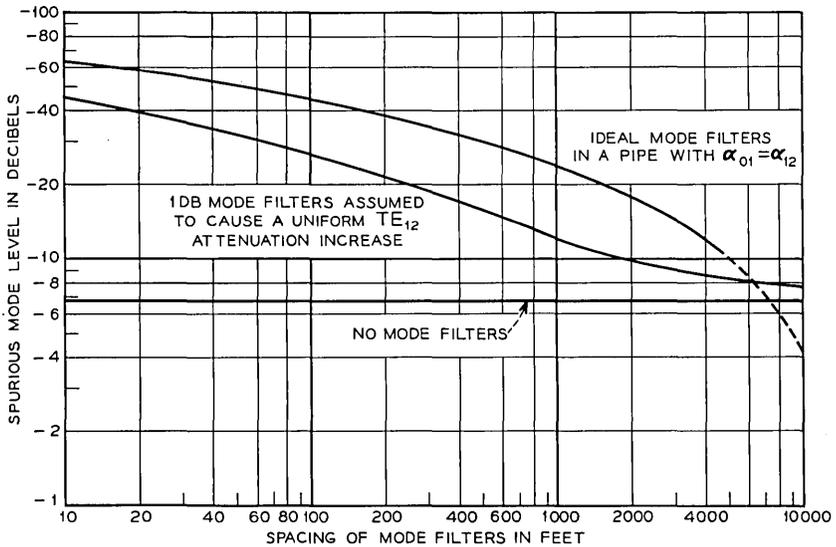
Fig. 3 — Spurious mode level of  $TE_{01}$ - $TE_{12}$  coupling in serpentine bends with mode filters; 2-inch I.D.  $2\frac{3}{8}$ -inch O.D.,  $\lambda = 5.4$  mm. Serpentine bends are caused by equally spaced supports and the elasticity of the copper pipe. The supporting distance is a multiple of the beat-wavelength between  $TE_{01}$  and  $TE_{12}$ .
