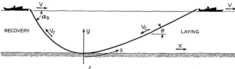
Fig. 8 — Definition of coordinates for the two-dimensional stationary model.
