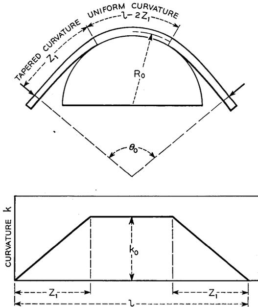
Fig. 1 — Normal mode bend with linear curvature taper.
