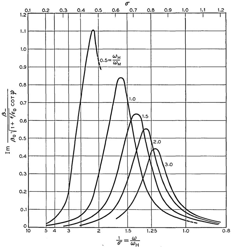
Fig. 8 — Attenuation of reverse wave versus frequency at a fixed magnetic field and saturation magnetization for various values of  $\omega_H/\omega_M = (\mu_0 H)/M$ . The curves for 0.5 and 1 are discontinued when  $p$  reaches unity.
