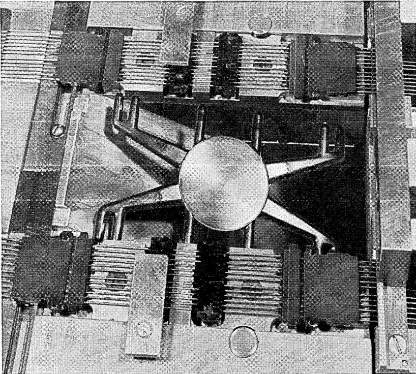
Fig. 16 — Cooling and culling section of automatic die.
