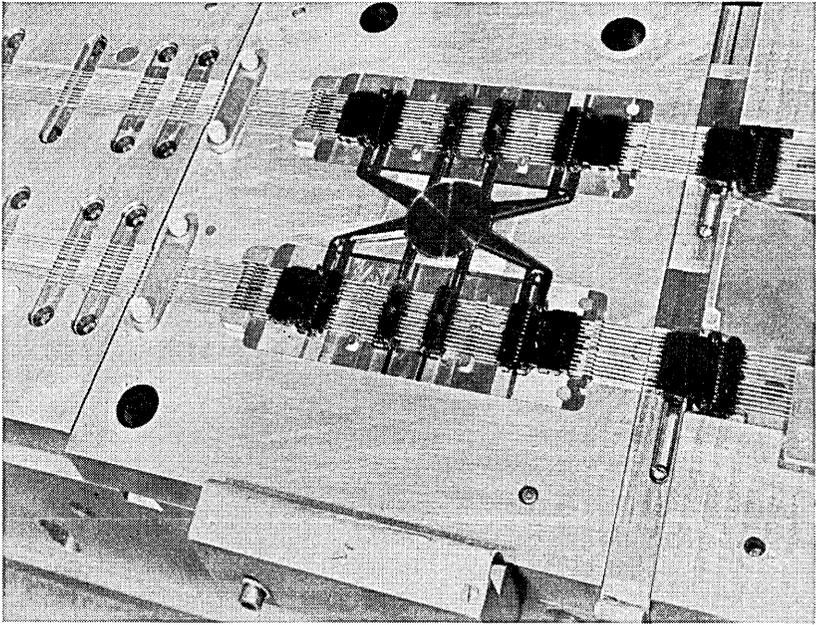
Fig. 15 — Molding section of automatic die.
