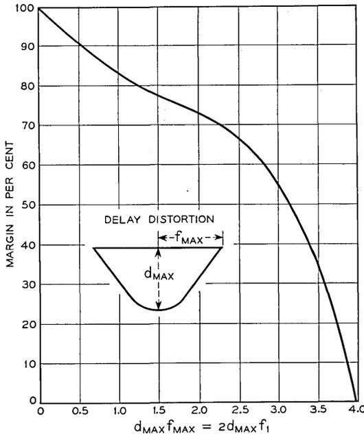
Fig. 43 — Margin against excessive peak interference in systems employing two pulse amplitudes with intervals between pulses  $\tau = \tau_1 = 1/2f_1 = 1/f_{\max}$ , for impulse transmission characteristic as shown in Fig. 23.
