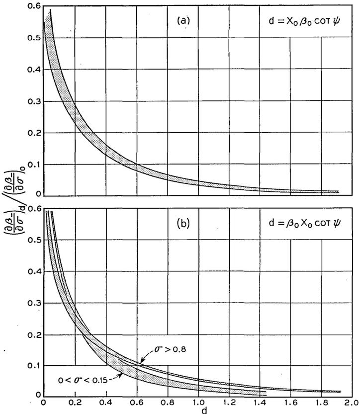
Fig. 10 — Ratios of reverse attenuation for a flat helix separated from the ferrite by a distance  $x_0$  to the reverse attenuation at  $x_0 = 0$ . Computations made from the approximate slope-formula for the loss, where applicable. (a)  $p = 0.2$ . (b)  $p = 0.8$ . In (a) all applicable  $\sigma$  values lie in the shaded region.
