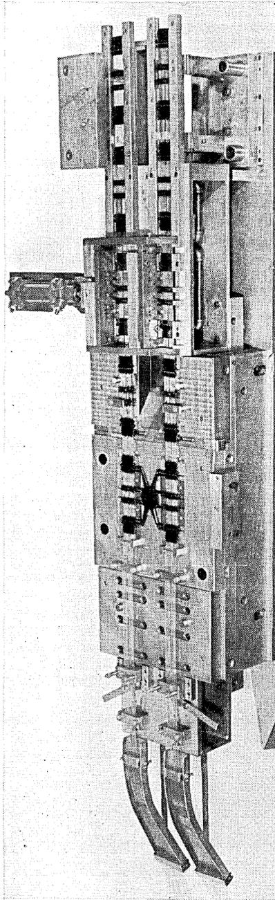
Fig. 12 — Lower half of typical automatically operated four cavity die.
