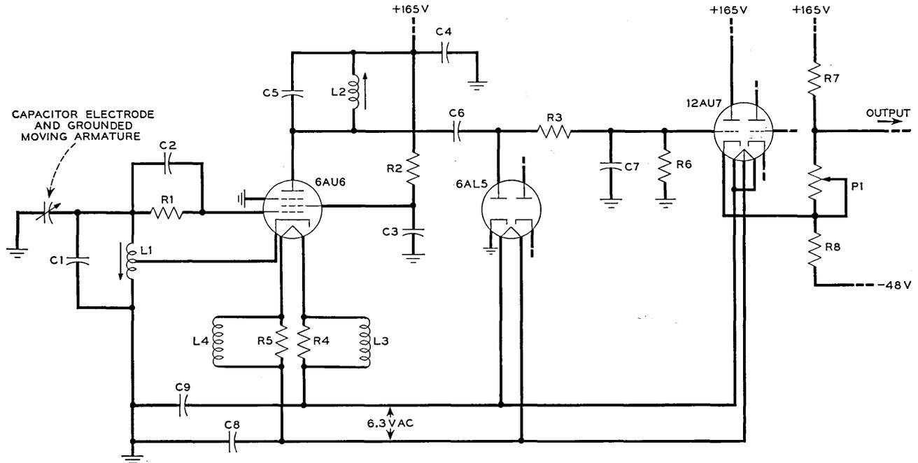
Fig. 3 — Schematic circuit of electrostatic gauge.
