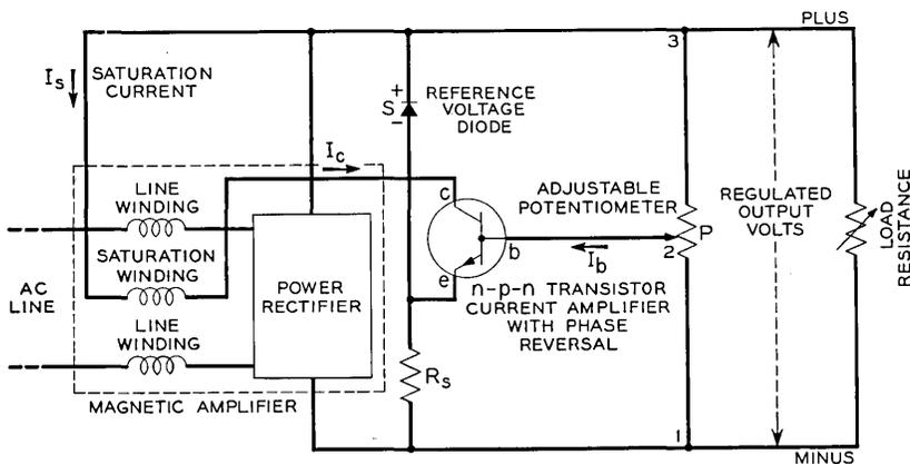
Fig. 16 — Transistor control circuit for a magnetic amplifier regulated rectifier with constant voltage regulation.
