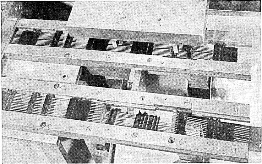
Fig. 17 — Indexing and shearing section of automatic die.
