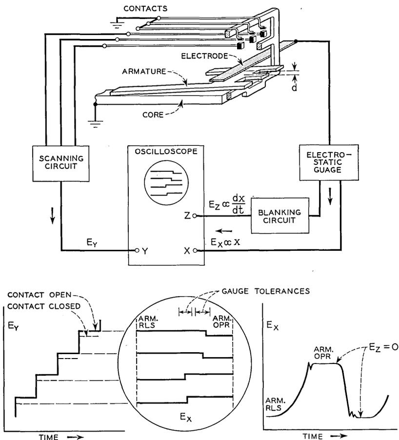
Fig. 1 — Schematic diagram of electronic relay tester.
