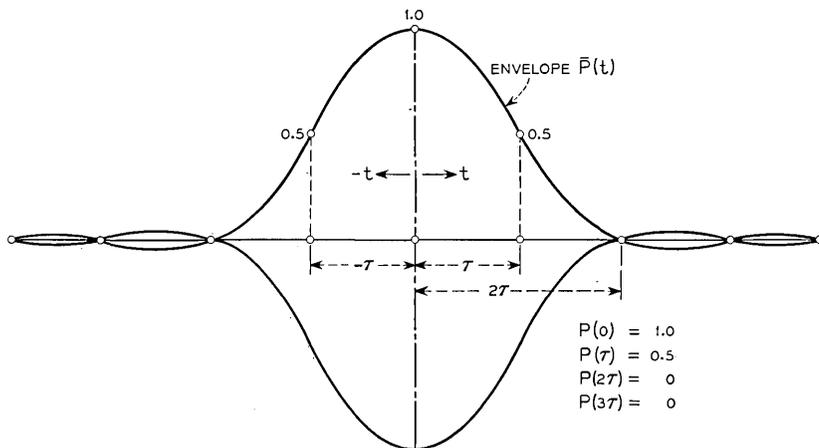
Fig. 47 — Envelope of idealized impulse characteristic.
