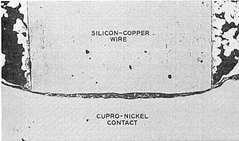
Fig. 19 — Section of a percussion weld. Original amplification 100 X.
