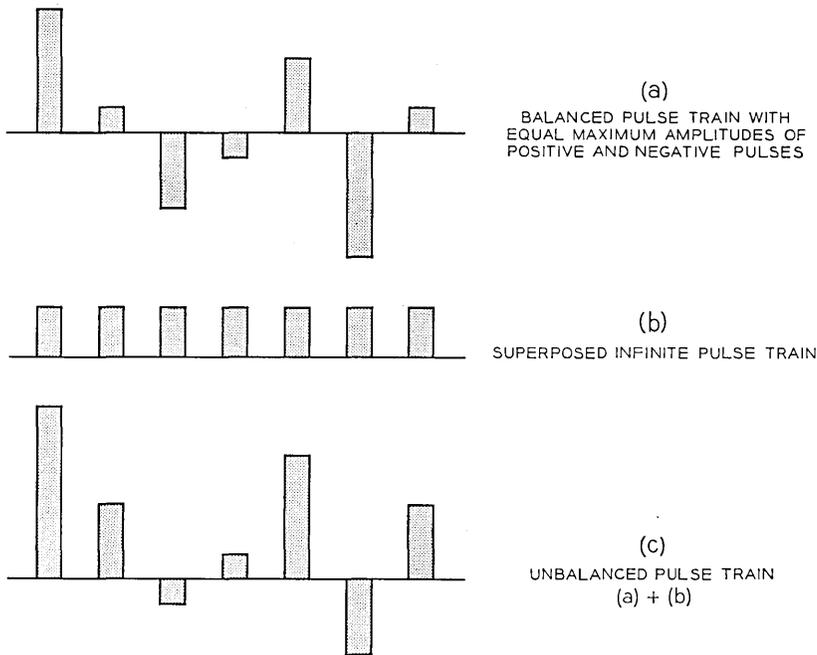
Fig. 44 Derivation of an unbalanced from a balanced pulse train by superposition of an infinite train of pulses of equal amplitude.
