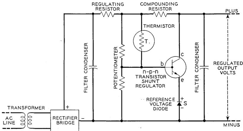
Fig. 19 — Grid-battery eliminator for phase-controlled thyatron rectifier.
