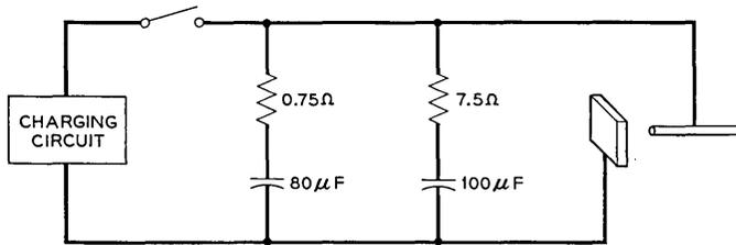
Fig. 4 — Practical welding circuit.
