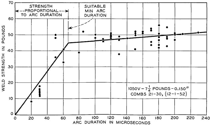
Fig. 20 — Weld strength versus arc duration.
