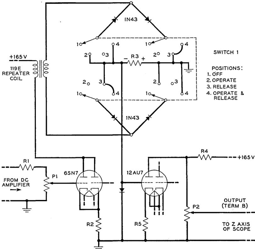
Fig. 8 — Schematic of oscilloscope brightening circuit.
