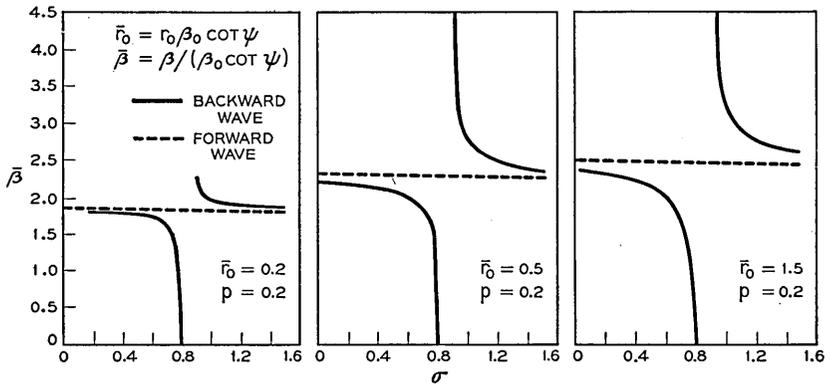
Fig. 13 — Reduced forward and reverse propagation constants versus  $\sigma$  for various reduced radii of a cylindrical helix. (Loss free case). The region  $1 - p < \sigma < \sigma_0$  is omitted. (a), above,  $p = 0.2$ . (b)  $p = 0.4$ . (c)  $p = 0.6$ . (d)  $p = 0.8$ . (e)  $p = 1.0$ .
