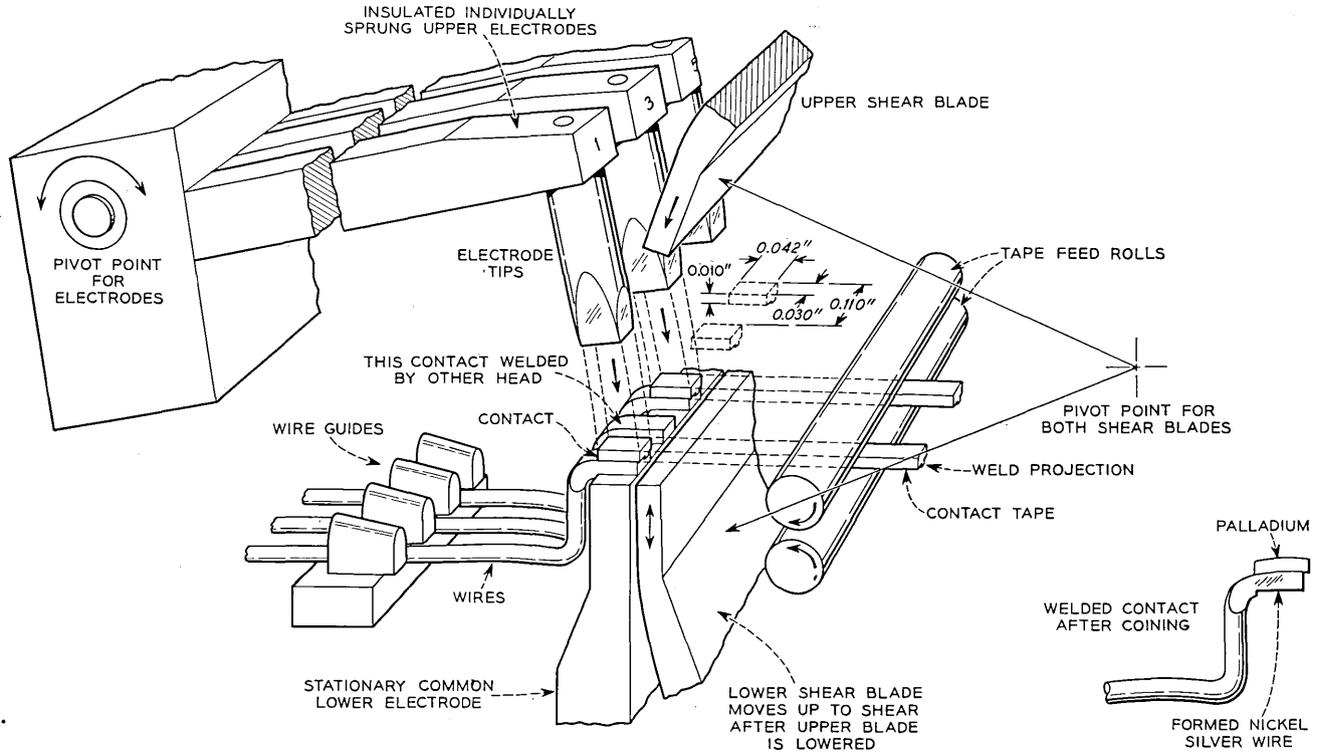
Fig. 5 — Sketch of a welding head.
