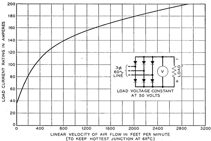
Fig. 4 — Junction rectifier forced cooling characteristics.
