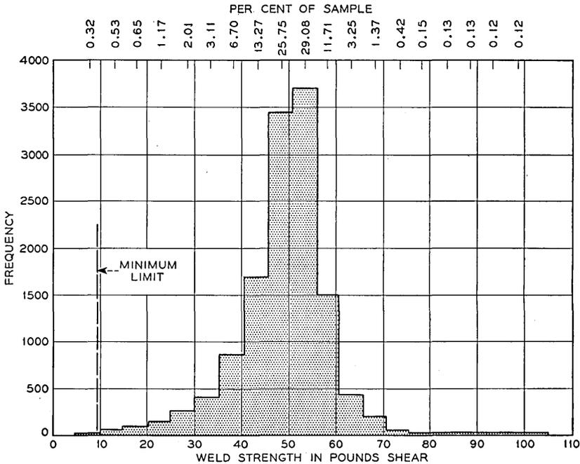
Fig. 22 — Weld strength distribution for 13,200 samples tested from 600,000 welds made in production.
