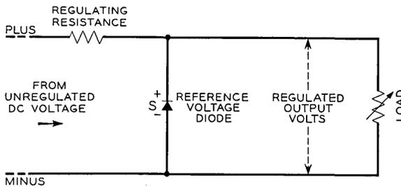
Fig. 11 — Simple shunt regulator.
