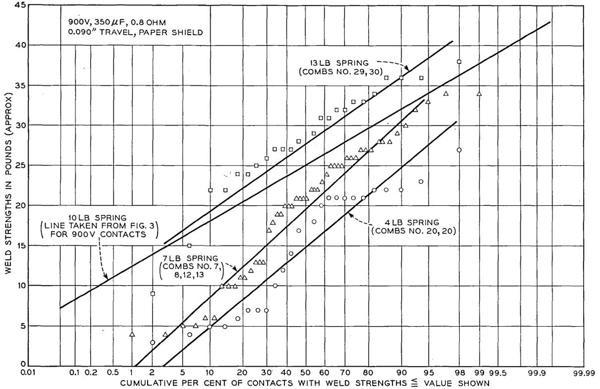
Fig. 16 — Effect of spring pressure on weld strength.
