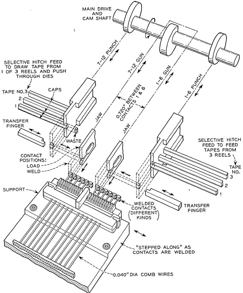
Fig. 18 — Schematic of the percussion welder.
