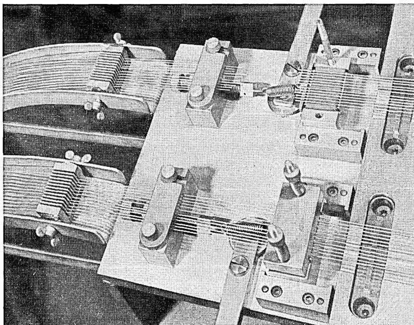
Fig. 13 — Wire guide section of automatic die.
