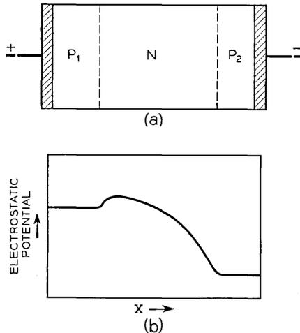
Fig. 4.1 — Space charge limited hole flow.
