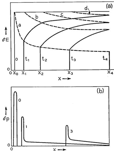
Fig. 4.3 — Graphical representation of the dependence of  $\delta E$  upon time.
