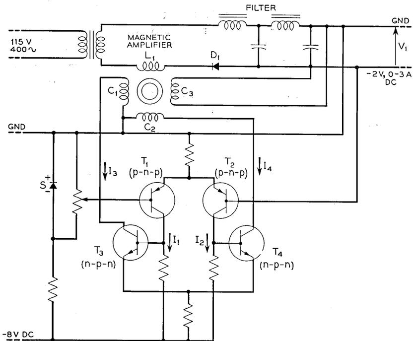
Fig. 21 — Two-volt three-ampere magnetic amplifier regulated rectifier.
