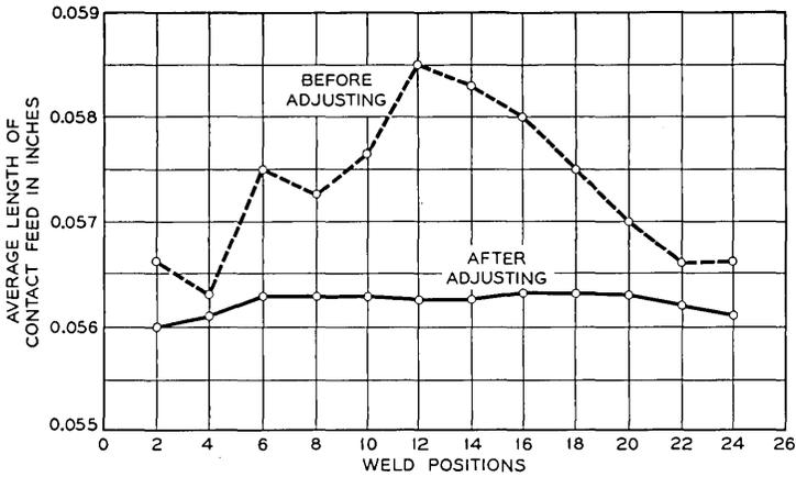
Fig. 6 — Contact length before and after adjusting hardness of rubber feed rolls and omitting gears between them.
