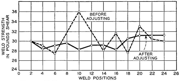
Fig. 8 — Weld strength versus resistance adjustment.
