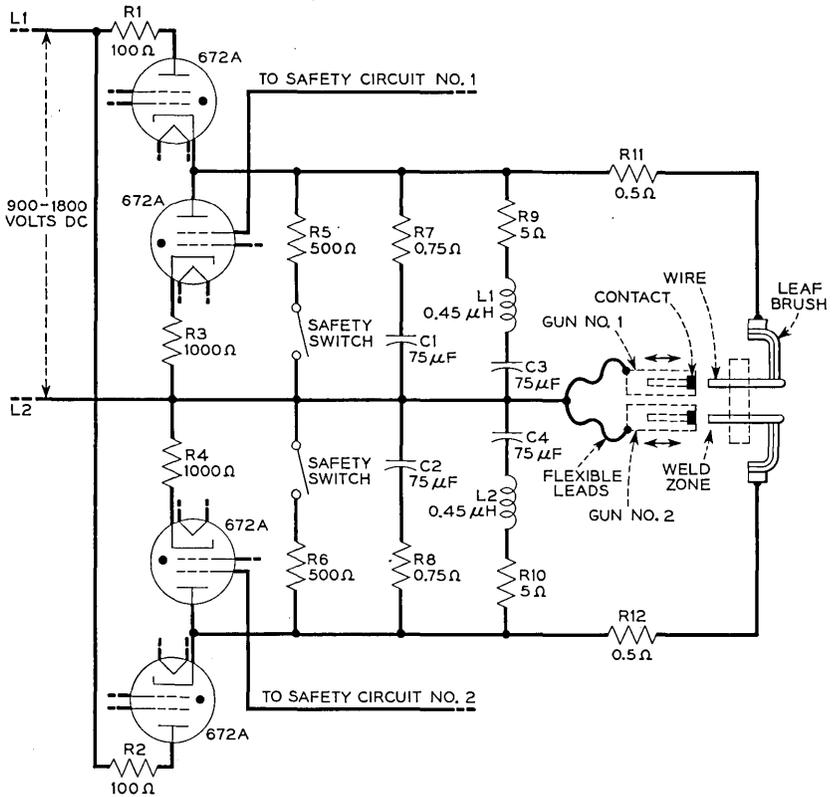
Fig. 21 — Schematic of percussion welder circuit.
