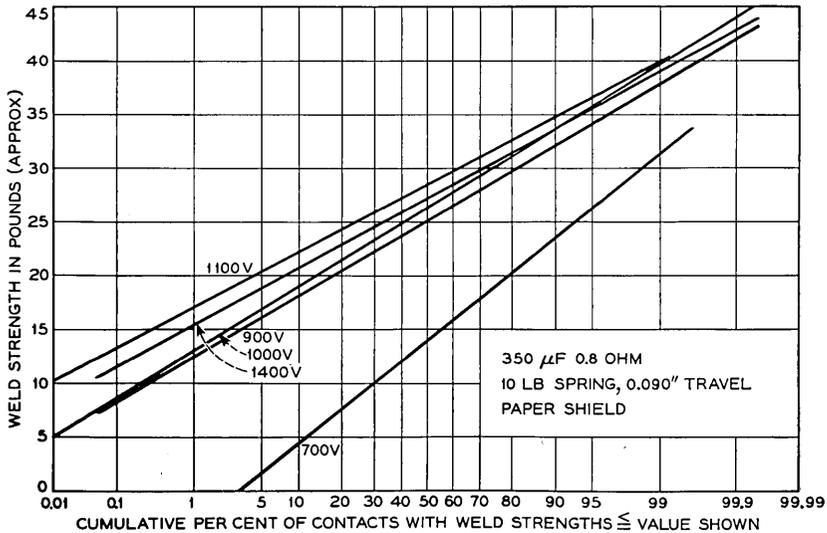
Fig. 15 — Effect of voltage variation on weld strength.
