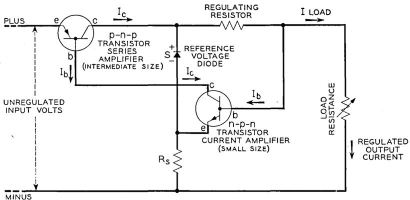
Fig. 15 — Transistor series regulator constant current regulation.
