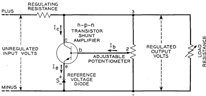
Fig. 12 — Transistor shunt regulator using one transistor.
