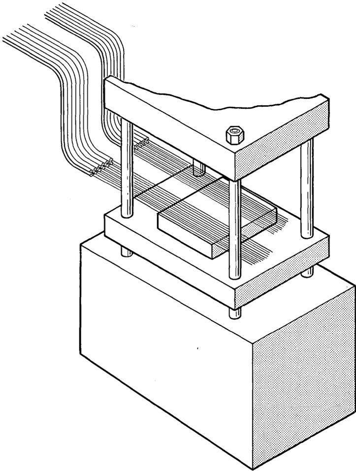
Fig. 3 — Sketch showing method of handling straightened wire from storage tubes.
