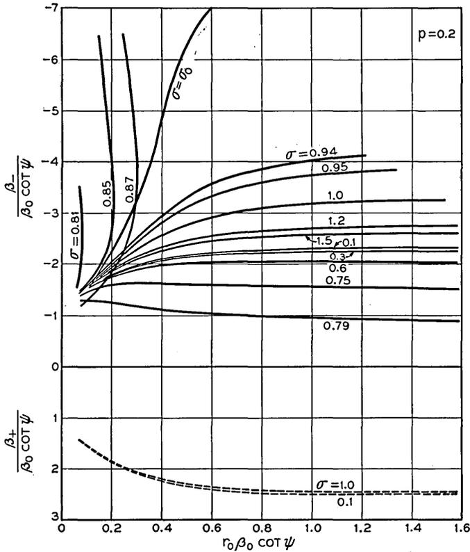
Fig. 12 — Reduced forward and reverse propagation constants versus reduced radius of a cylindrical helix (loss-free case) for various  $\sigma$  and  $p$ . The range  $\sigma_1 < \sigma < \sigma_0$  where
