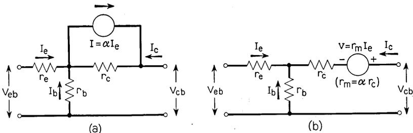
Fig. 9 — Junction transistor equivalent circuits. Typical values for a 50-mil-watt transistor:  $r_e$ , 25 ohms;  $r_b$ , 500 ohms;  $r_c$ , 5 megohms;  $\alpha$ , 0.98; and  $r_m$ , 4.9 megohms.
