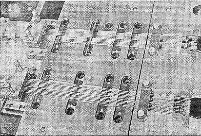
Fig. 14 — Anchoring section of automatic die.
