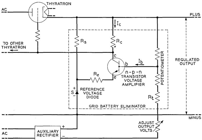
Fig. 20 — Grid-battery eliminator for magnitude controlled thyatron rectifier.
