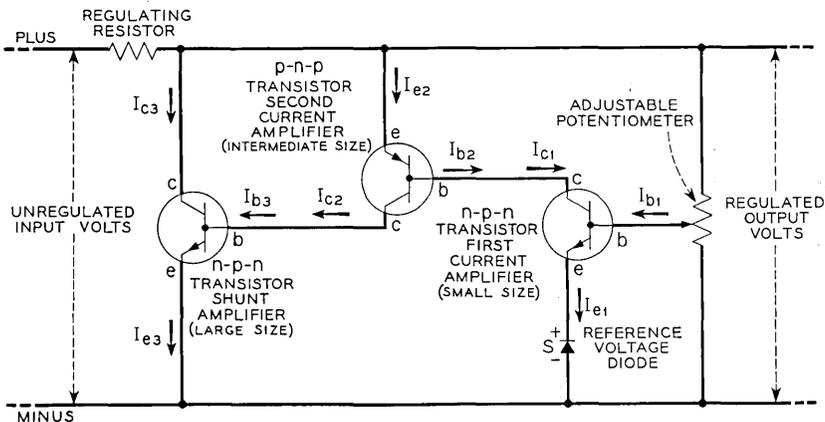
Fig. 13 — Transistor shunt regulator using three transistors.
