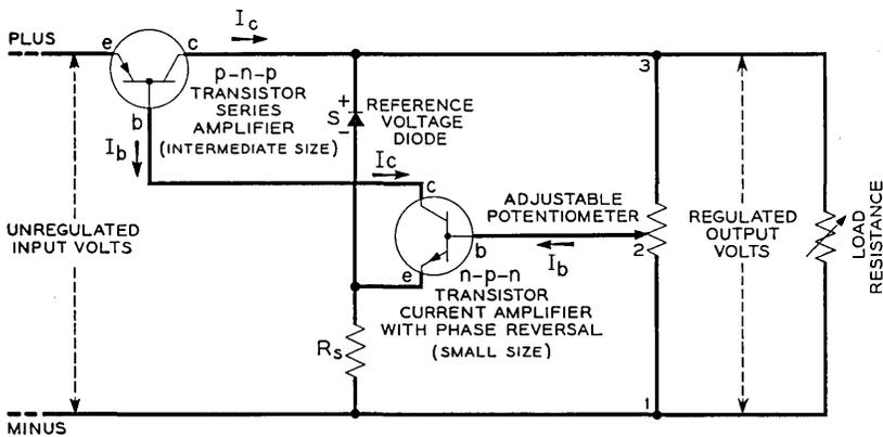
Fig. 14 — Transistor series regulator constant voltage regulation.
