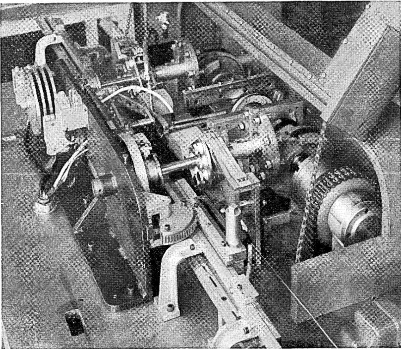
Fig. 11 — Percussion welder for contacts on single-wire combs.
