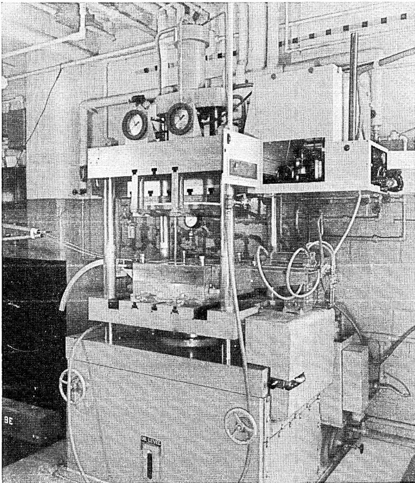
Fig. 8 — Experimental prototype automatic transfer molding machine.
