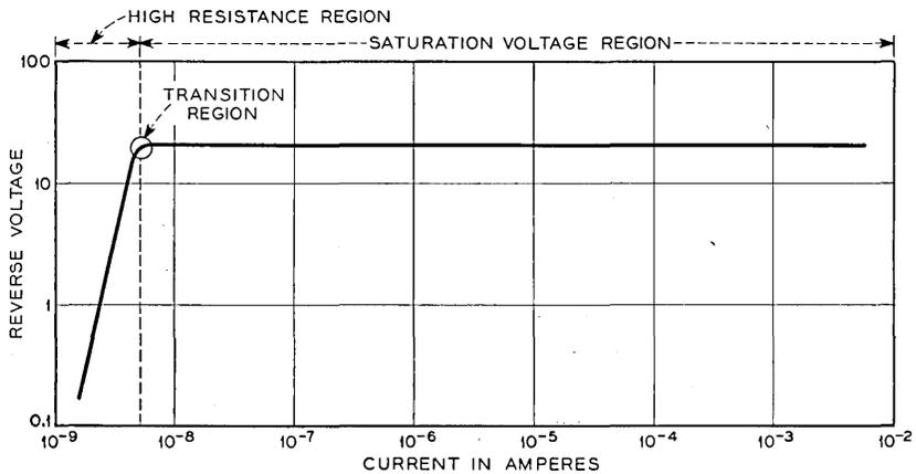
Fig. 5 — Reverse characteristics of a reference voltage diode.
