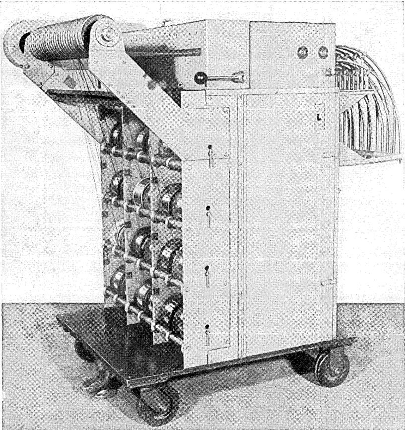
Fig. 4 — 24 double head wire straightening machine.
