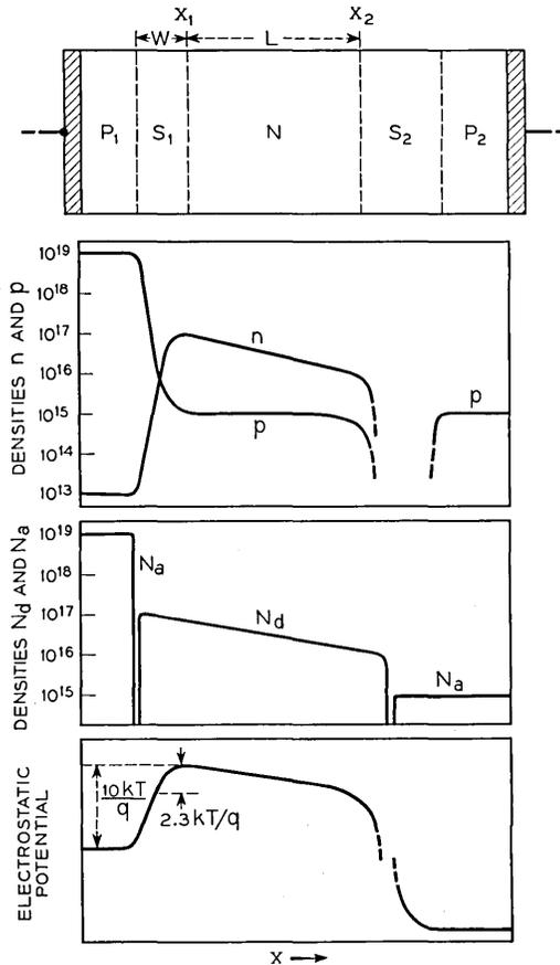
Fig. 3.1 — Constitution of minority carrier delay diode.
