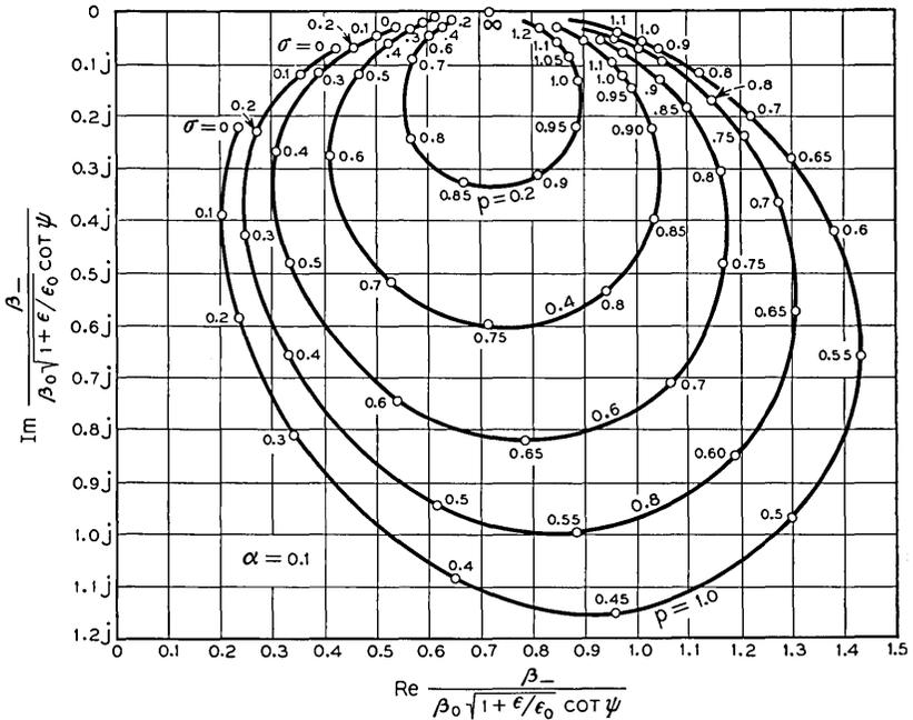
Fig. 6 — Real and imaginary parts of the reverse propagation constant  $\beta_-$  of a flat helix versus  $\sigma$  for various  $p$  and for  $\alpha = 0.1$  (the parameter  $\sigma$  is marked along the curves). The forward propagation constant has a very small imaginary part which hardly varies with  $\sigma$ .
