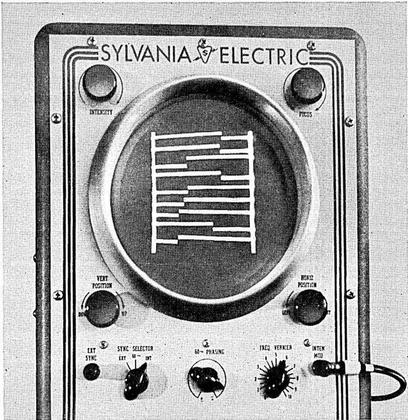
Fig. 7 — Photograph of the 7-inch oscilloscope with a typical gauging pattern on the screen.
