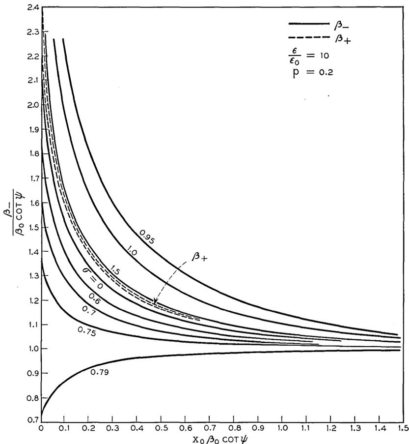
Fig. 9 — Propagation constants for a flat helix separated from the ferrite by a distance  $x_0$  for various values of  $\sigma$ . (Loss-free case) (a)  $\beta_-$  and  $\beta_+$  for  $p = 0.2$ , (b)  $\beta_-$  for  $p = 0.8$ , (c)  $\beta_+$  for  $p = 0.8$ . In (a), above, the dotted lines bound all  $\sigma$  values.
