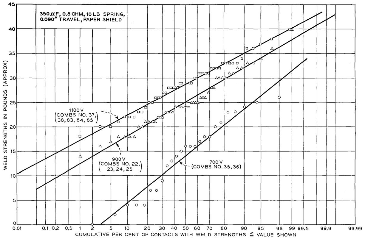
Figs. 14 — Effect of voltage variation on weld strength. (Typical establishing data.)
